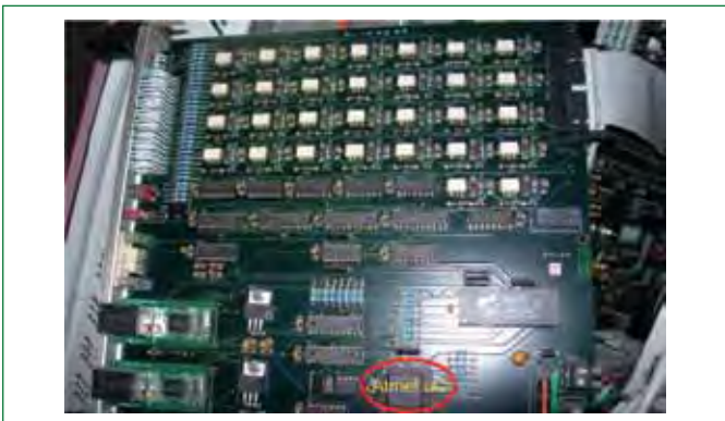
Figure 4: Microcontroller based RTU board
