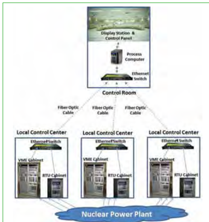
Figure 1: Architecture of distributed digital control systems
