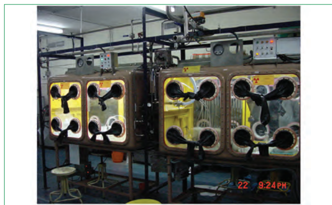
Figure 7: Mixer-settler facility used for flow sheet development studies
