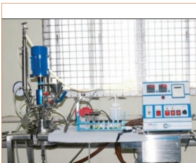
Figure 1: Experimental set up: SS- autoclave
