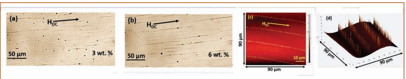
Figure 2: Optical phase contrast microscopy images showing linear chain-like structures along the direction of an external magnetic field ( H_{DC} \sim 80 G, indicated in the figure) for ferrofluids with MNP concentrations of (a) 3 wt. % and (b) 6 wt. %. (c) AFM topography image of oriented ferrofluid (serially diluted) dried in-situ on a freshly cleaved mica substrate, in the presence of H_{DC} \sim 80 G. (d) 3D topography view of Figure 2c
