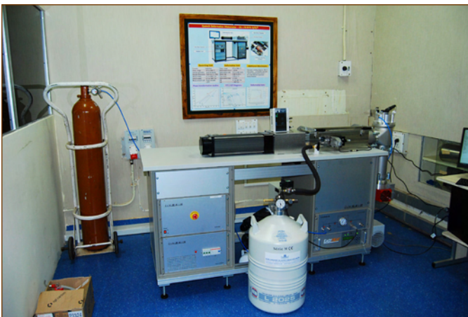
Figure 1: Quench Deformation Dilatometer with subunits installed in PMD/MMG
