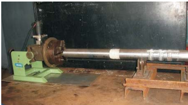
Shaft mounted on the weld set-up
