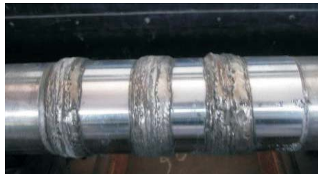
Reconditioned shaft after welding
