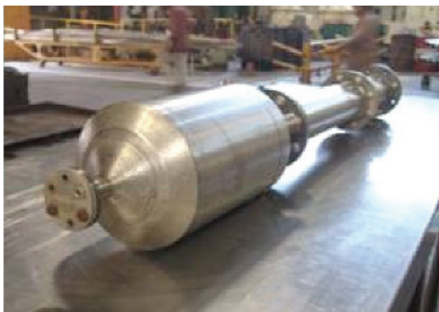
Figure 2: Zircaloy-4 corrosion testing system (10 litres) for three phase corrosion evaluation in 11.5M nitric acid
