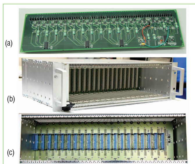
Figure 1: (a) Conceptual active backplane, (b) industrial prototype passive backplane with 3U bin and (c) backplane field I/O connectors
