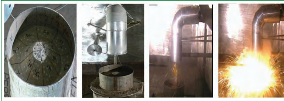
Figure 4: Test sequence of flowing sodium fire scenario on concrete
