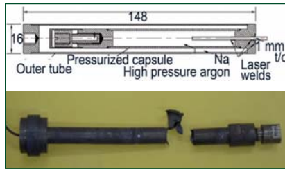
Fig. 1 Sketch of pressurized capsule and the ruptured pressurized capsule
