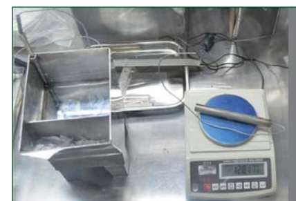
Fig. 4 Pressurized capsule with sodium filled in the safety tube inside the glove box
