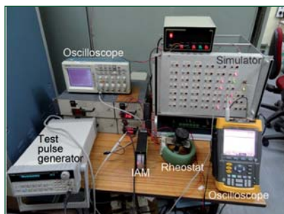
Fig. 2 Laboratory test setup of relay based safety logic system
