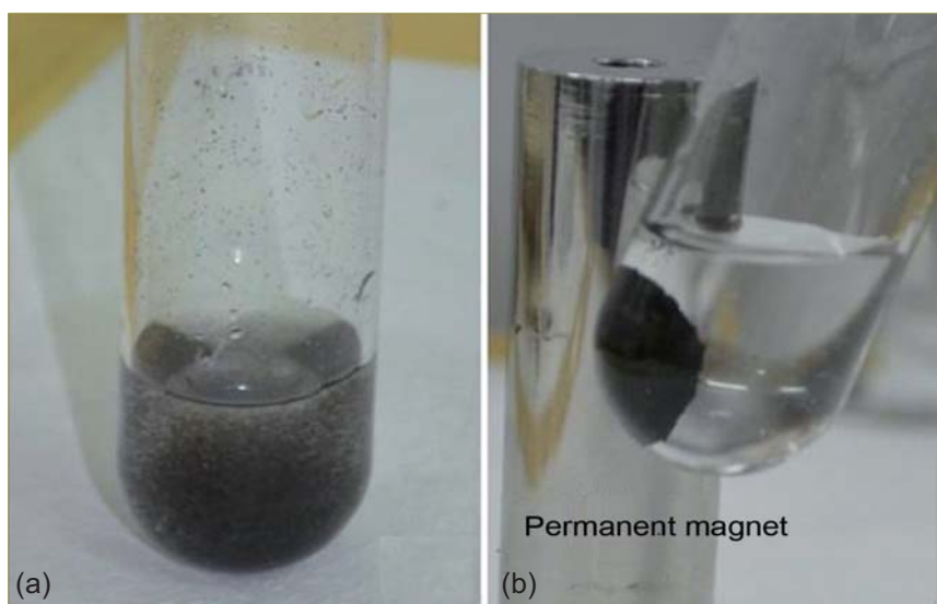
Fig. 2 (a) Metal ion solution and (b) separation in the presence of magnetic field
