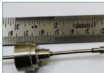
Fig. 3 Photograph of miniature sodium leak detector
