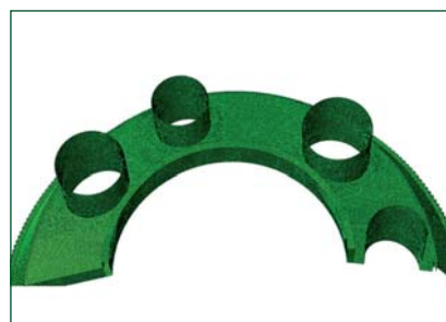
Fig. 2 Meshed model of roof slab
