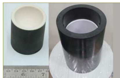
Fig. 2 As-received yttria coated HDG crucibles without bond coat for uranium melting experiments
