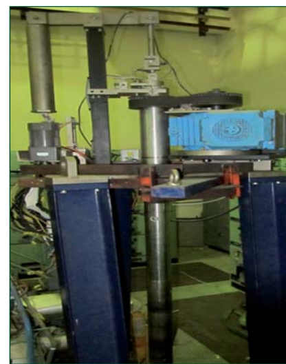
Fig. 2 Indigenously developed pin on disc tribometer
