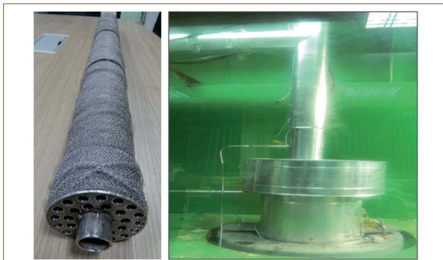
Fig. 3 Wire mesh arrangement and sodium bubbler facility
