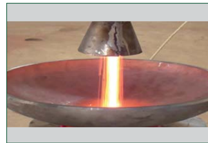
Fig. 2 Experimental simulation of fall of granules
