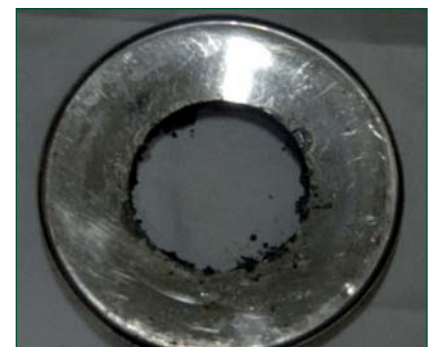
Fig. 6 Fusible plug after melting
