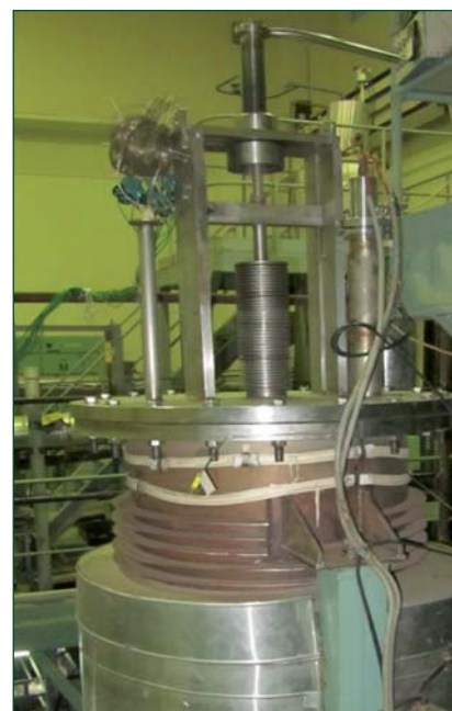
Fig. 3 Thermal striping test vessel
