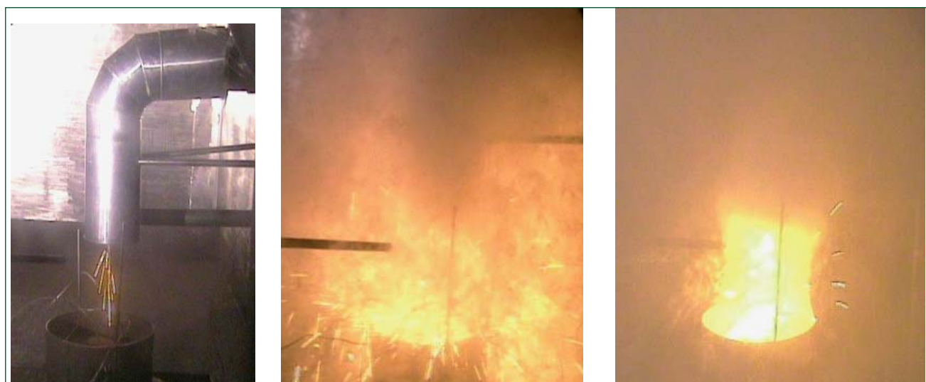
Fig. 2 Scenarios of sodium fire on concrete specimen
