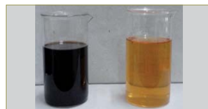
Fig. 2 Simulated raffinate solution before and after passing ozone
