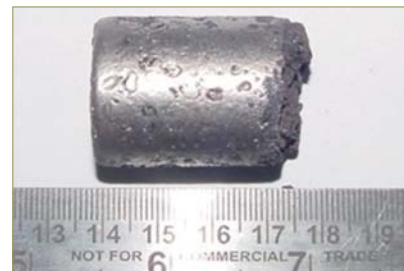
Fig. 2 Uranium ingot obtained after induction melting
