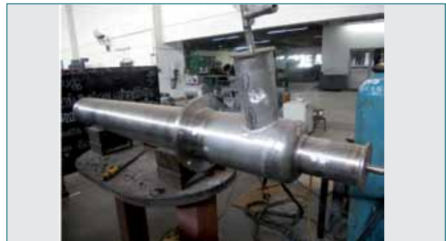
Fig. 2 Leak testing of ALIP
