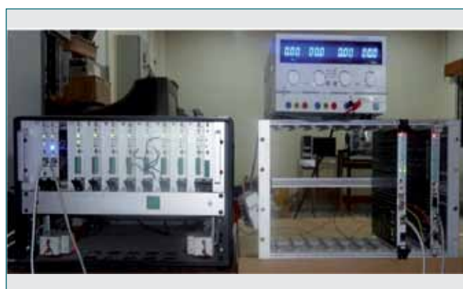
Fig. 2 Prototype data diode test setup
