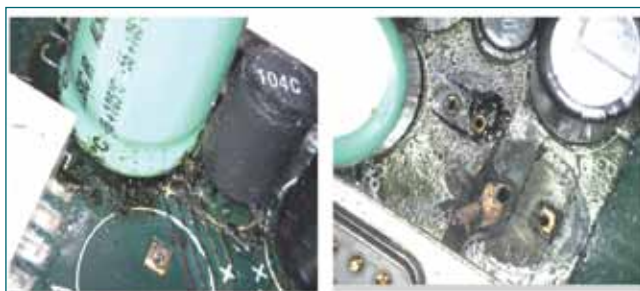
Fig. 1 Burnt tracks capacitor leak in failed PCB
