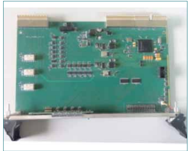
Fig. 2 Compact PCI bus based optical encoder interface card
