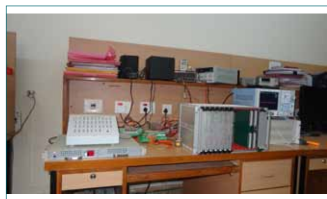
Fig. 3 Functional testing of PCL bin with signal simulator
