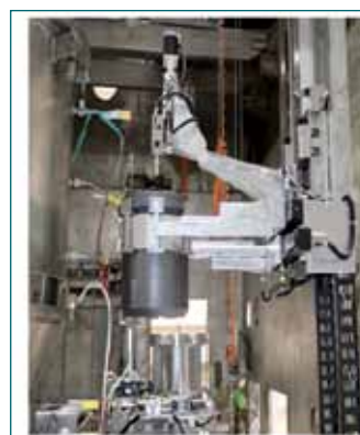
Fig. 2 CTM gripping graphite crucible inside CB
