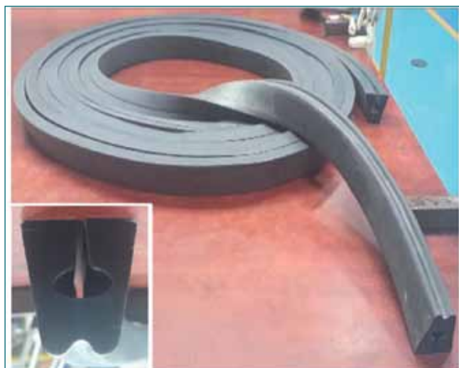
Fig. 3 Seven metre continuous length back-up seal (inset: cross section of the seal)
