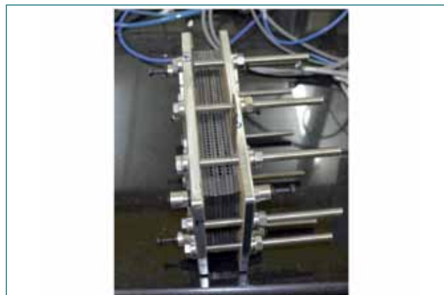
Fig. 2 Fuel cell stack using WC/C coated SS 304 mono-polar plates
