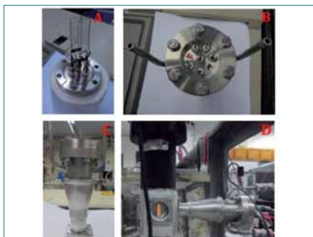
Fig. 1 Photograph showing the electron-gun assembly (A) tungsten filament with accelerating grid (B) top view of feed through connectors on which filament and accelerating grids are connected (C) complete electron-gun assembly and (D) coupling of electron-gun assembly and matrix isolation set-up
