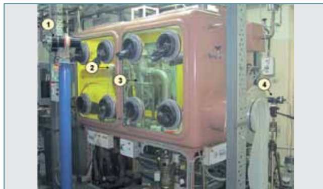
Fig. 2 Spot-technique equipment used for the measurement of solidus-liquidus temperature of metallic fuel. 1: Magnifying device (long distance optical microscope); 2: vacuum gauge; 3: experimental chamber; 4: pyrometer
