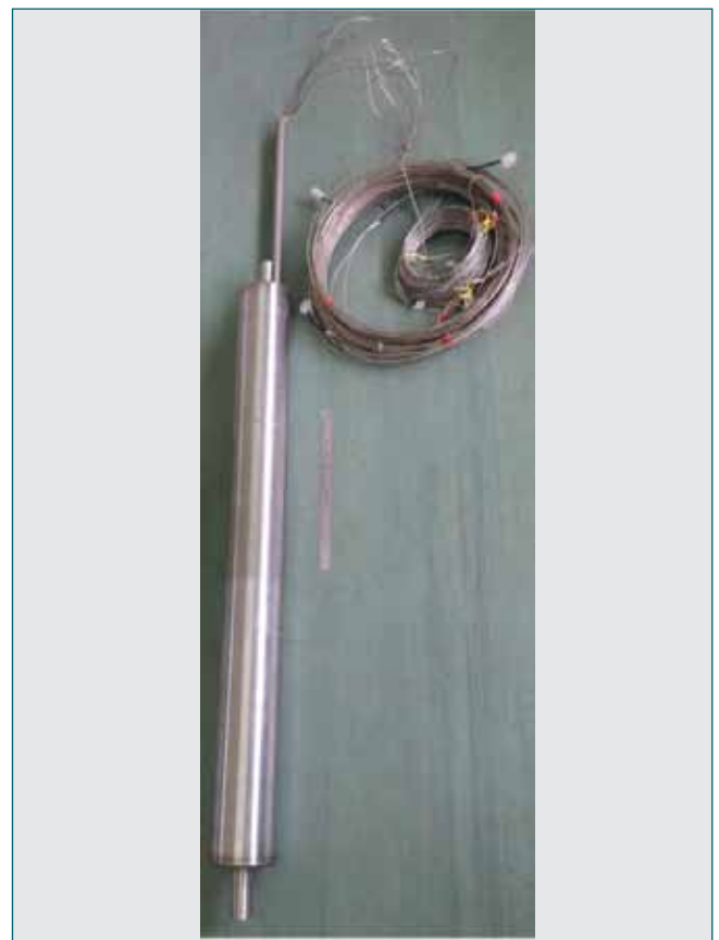
Fig. 2 Photograph of manufactured miniature ALIP
