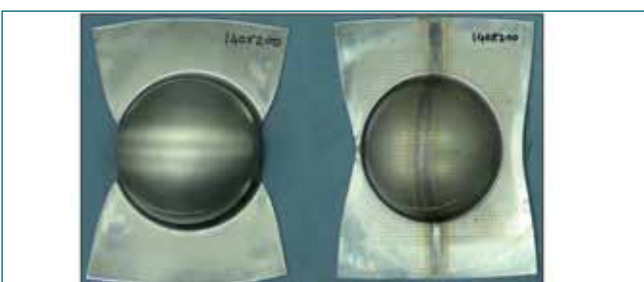
Fig. 1 Earring in formed samples, as received and TWB
