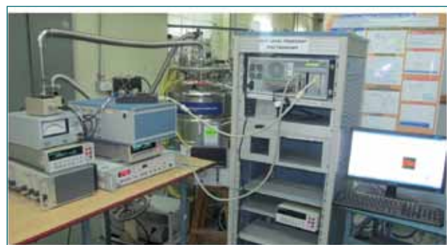
Fig. 1 DLTS experimental set up (20-400 K)
