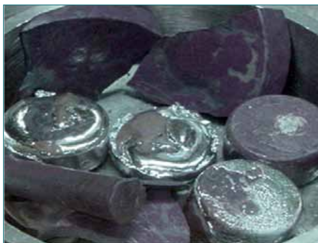
Fig. 4 Cadmium and salt after back extraction experiments
