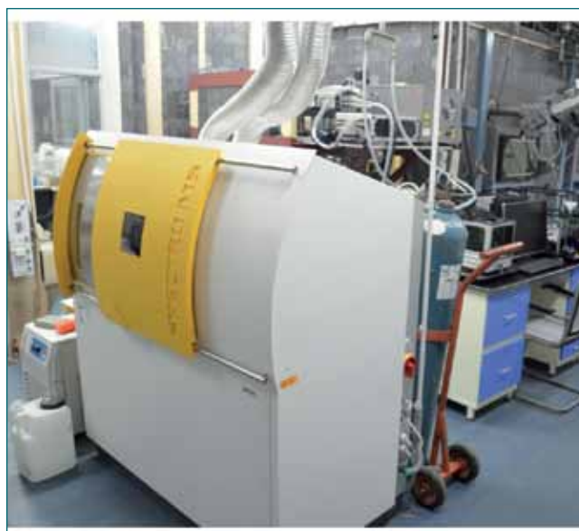
Fig. 5 LIBS and LA-ICP-MS facility in mini cell
