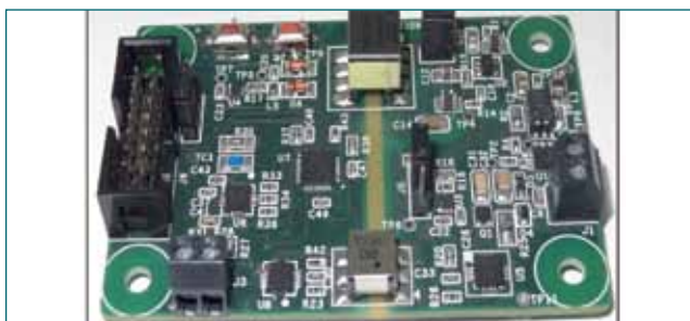
Fig. 2 Prototype thermocouple loop powered transmitter sufficient efficiency also at very small power range (few 10's of mW).
