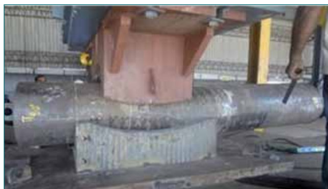
Fig. 2 Pressing of pipe in full length die
