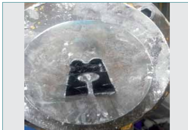
Fig. 1 Back-up seal is being extruded
