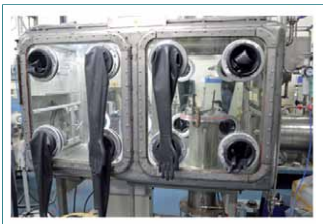
Fig. 1 Sodium bonding furnace inside glovebox
