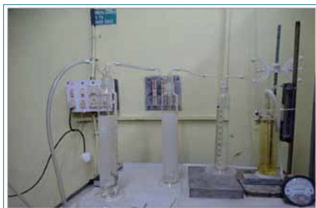
Fig. 1 Sketch of NO x scrubbing experimental setup
