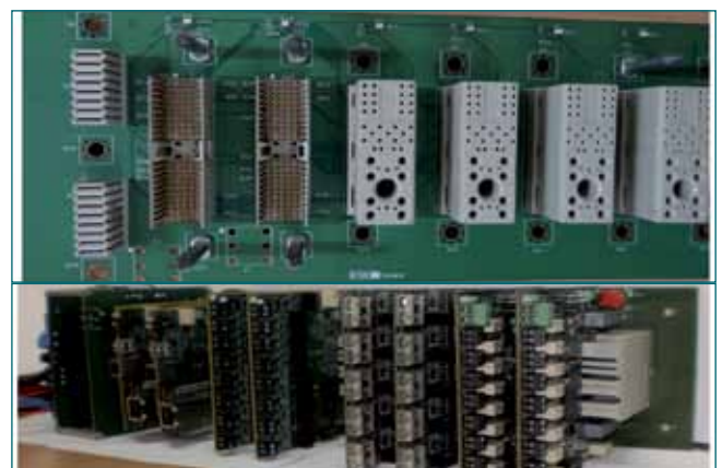
Fig. 3 (a) Fabricated backplane and (b) complete system assembled with dual redundant power supply, dual redundant CPU and various IO modules
