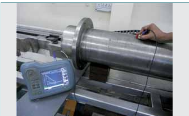
Fig. 1 UT of ALIP outer duct
