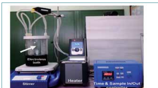
Fig. 1 Photograph of the electroless bath assembly for nano copper coating inside titanium tubes. Arrow indicating the Ti tube being coated
