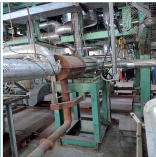
Fig. 1 5 m 3 /h annular linear induction pump in sodium loop
