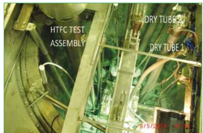
Figure 5: Dry tubes and high temperature fission counter assembly
