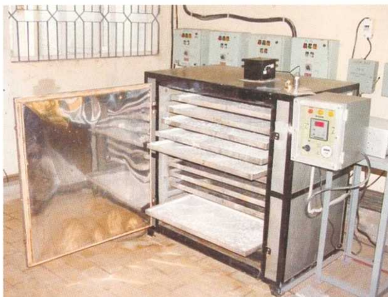
Fig. 3 A view of Tray Drier with powder in trays
