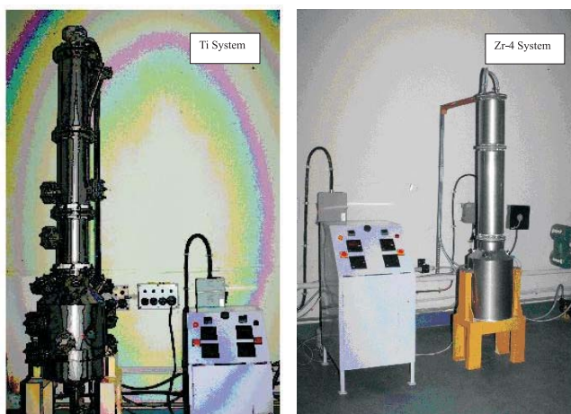
Fig. 7: Titanium Gr-2 and Zircaloy-4 Corrosion testing systems
