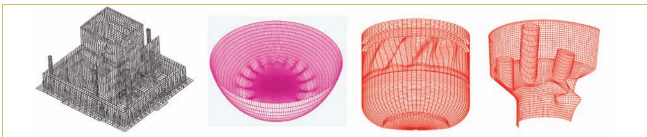
Figure 2: Finite element models of nuclear island inter-connected buildings and vessels for investigations of buckling under seismic forces
