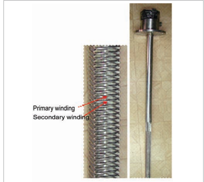
Figure 2: Continuous type mutual inductances level probe
