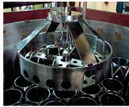
Figure 7: Transducer holder for under sodium ultrasonic scanner
