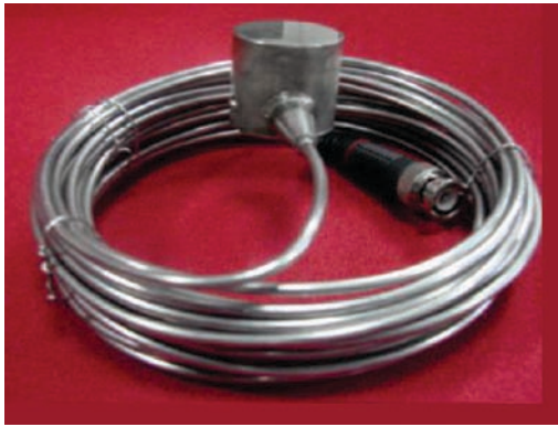
Figure 6: Under sodium ultrasonic transducer
