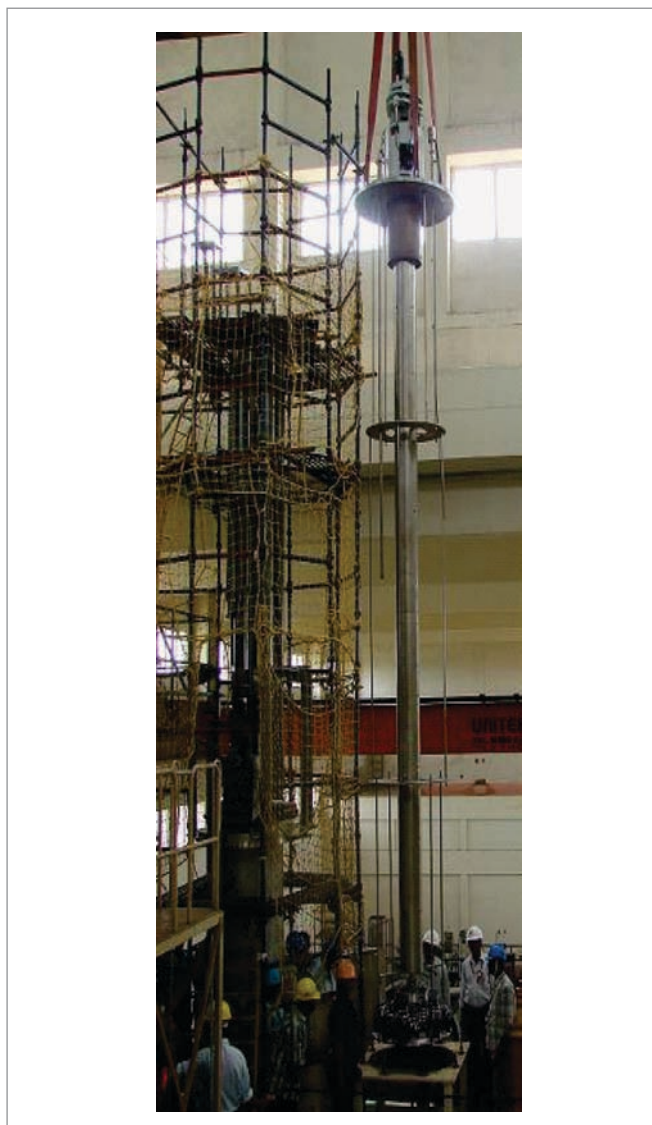
Figure 5: Under sodium ultrasonic scanner
