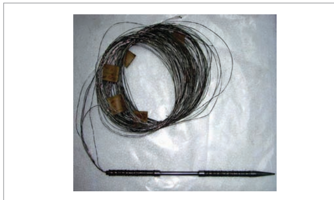
Figure 4: Eddy current flow sensor for PFBR
