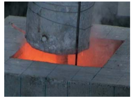
Fig. 5. Sodium Exposure on Test Block
