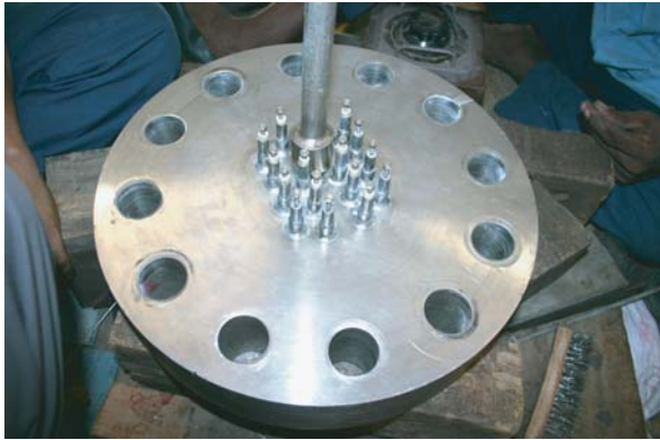
Fig. 1. Heater assembly for surge tank
