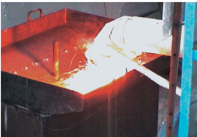
Fig. 1. Experiment on a typical Leak Collection Tray
