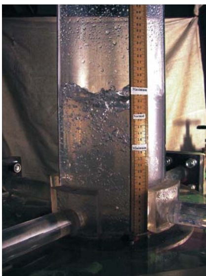
Fig.1. Perspex model of Surge Tank
