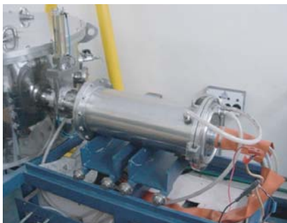
Fig. 1. The plasma torch integrated with the aerosol chamber through plenum chamber
