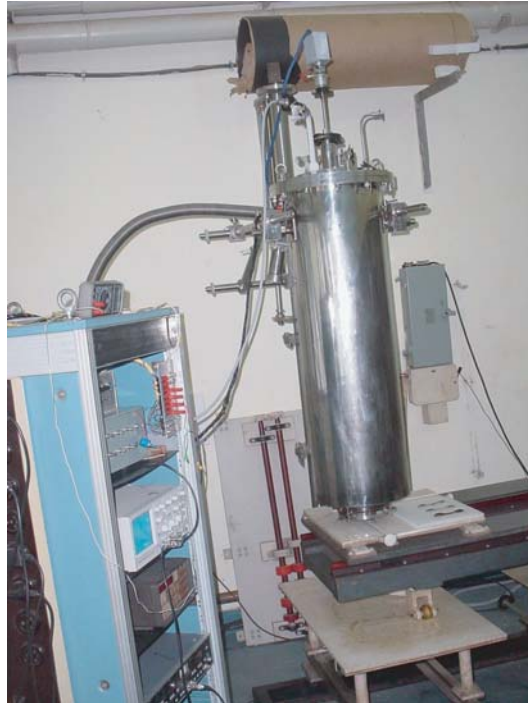
Fig. 1. SQUID based system for NDE.
