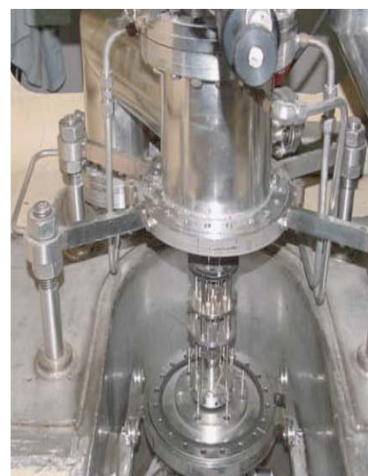
Fig. 1. A quadrupole mass spectrometric system and the electron bombardment furnace assembly for conducting vaporization thermodynamic studies of radioactive substances.
