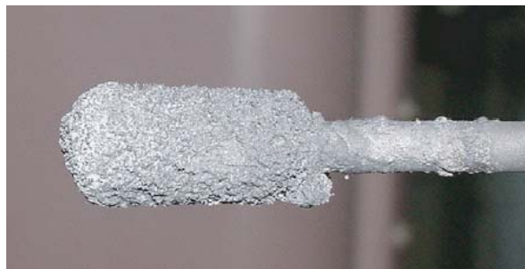
Fig. 2. Cathode deposit of \text{UO}_2
