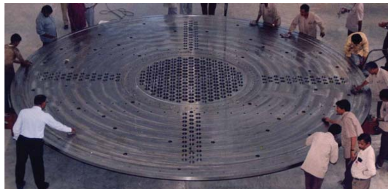
Fig. 2. Bottom plate after final machining
