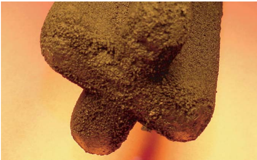
Fig 3. Enriched elemental boron deposit
