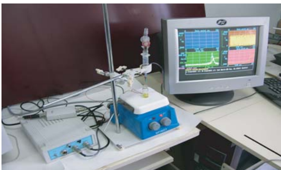
Fig. 1. An in-house built miniature rapid potentiometric titration facility.
