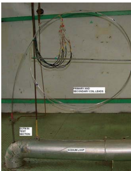
Fig 2. Test section in 500 kW loop
