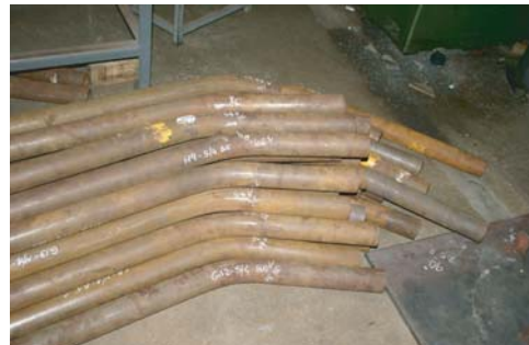
Fig. 1. Inlet and outlet feeder pipes for MAPS-1
