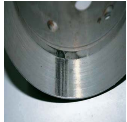
Fig. 4 . Scoring Marks on the Handling Head
