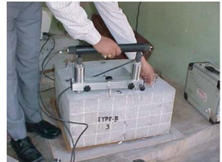
Fig. 2: Impact Echo Testing
