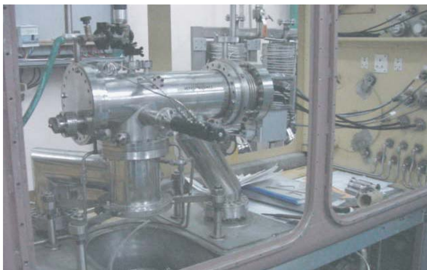
Fig. 1. A quadrupole mass spectrometric system and the electron bombardment furnace assembly for conducting vaporization thermodynamic studies of radioactive substances.
