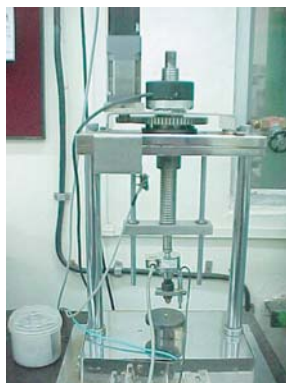
Fig. 1b. Motorised ball screw test system
