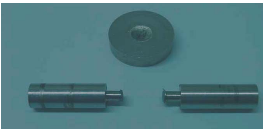
Fig 4. Pin and Disc used in tribometer
