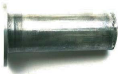
Fig. 1. Pin with Longitudinal Marks
