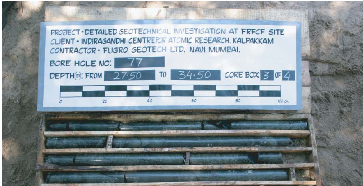
Fig. 2. Photograph showing typical rock core sample.
