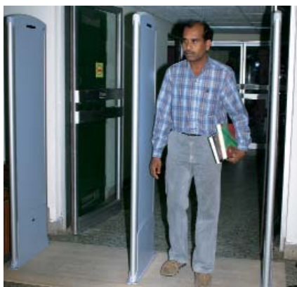
Fig. 2. The RFID anti-theft system
