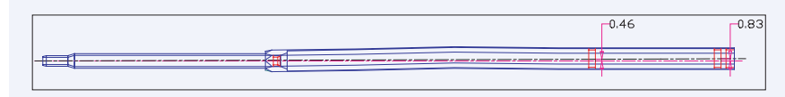
Fig. 5. Shift in the axis of the control rod sheath at the stellite tracks w.r.t. its foot region
