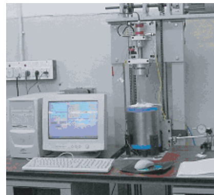
Fig. 3. The indigenously built dilatometer system.
