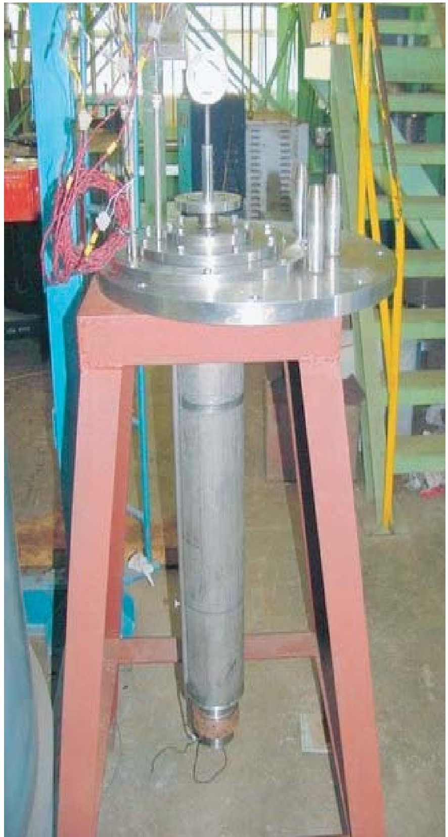
Fig. 3. ECPS model for sodium testing.
