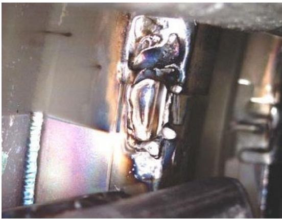
Figure 7: Damage in JET Tokamak by Runaways
