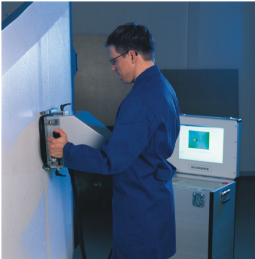
Fig. 7: Portable shearography system for field inspection of composite materials
