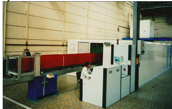
Fig. 1: Helicopter rotorblade inspection system
