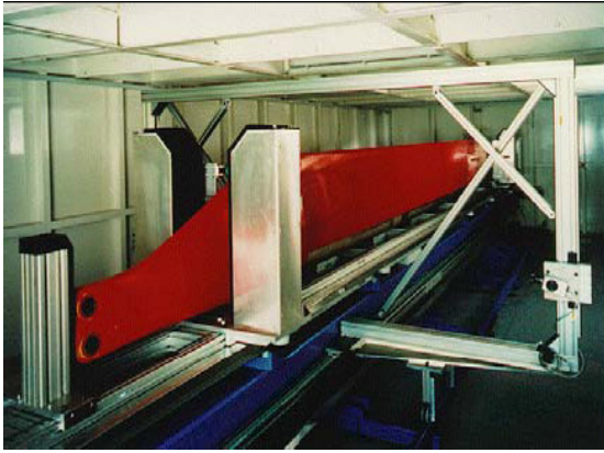
Fig. 2: View inside the vacuum chamber with rotorblade in testing position
