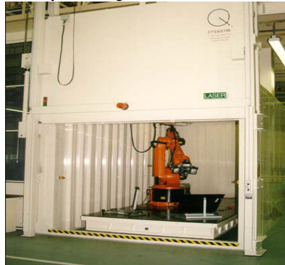
Fig.3: 6-axis industry robot in automatic inspection system of thermal protection parts.
