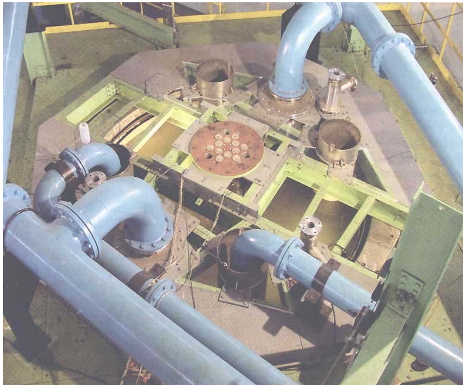
Fig.2: Top view of the model showing the control plug, IHX and DHX positioned in the hot pool
