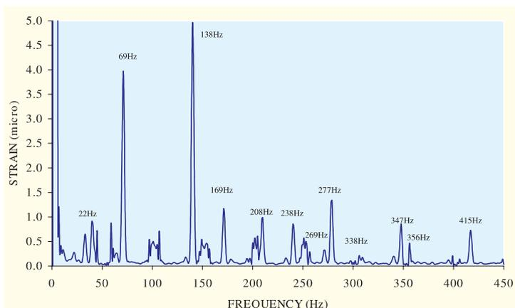
Fig. 1 : Vibration spectra of fuel pin (Flow-184 Cu.m/h)
