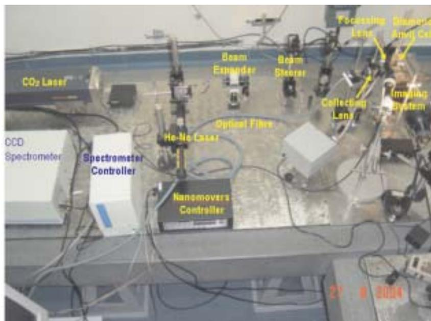
Fig.2: Photograph of the set-up; All components, including the lasers are mounted on a granite table located on a special foundation, structurally isolated from the rest of the building to minimize vibrations.
