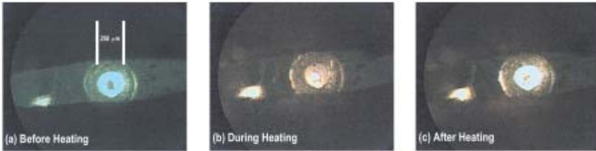
Fig. 3 : Heating of Graphite with the LHDAC set-up of P~14 GPa: (a) before heating; (b) during heating by CO<sub>2</sub> laser and (c) after heating. (Webcam Pictures)
