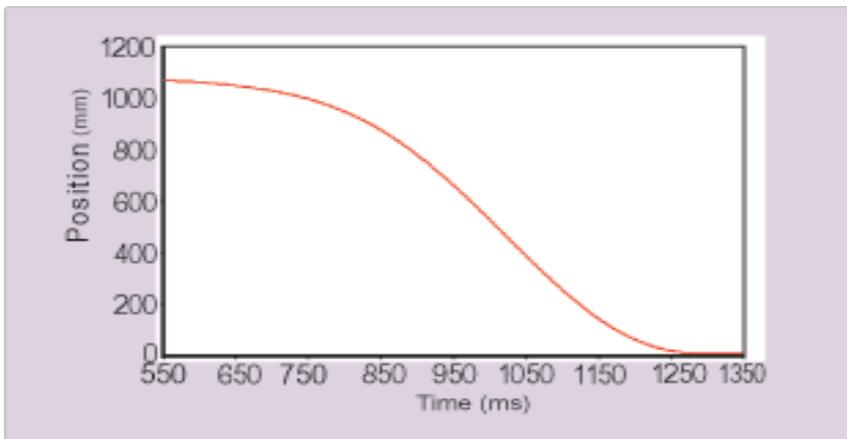
Fig.2: Displacement of CSR w.r.t. Time during SCRAM
