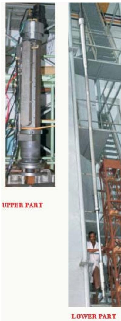
**Control and Safety Rod Drive Mechanism**
