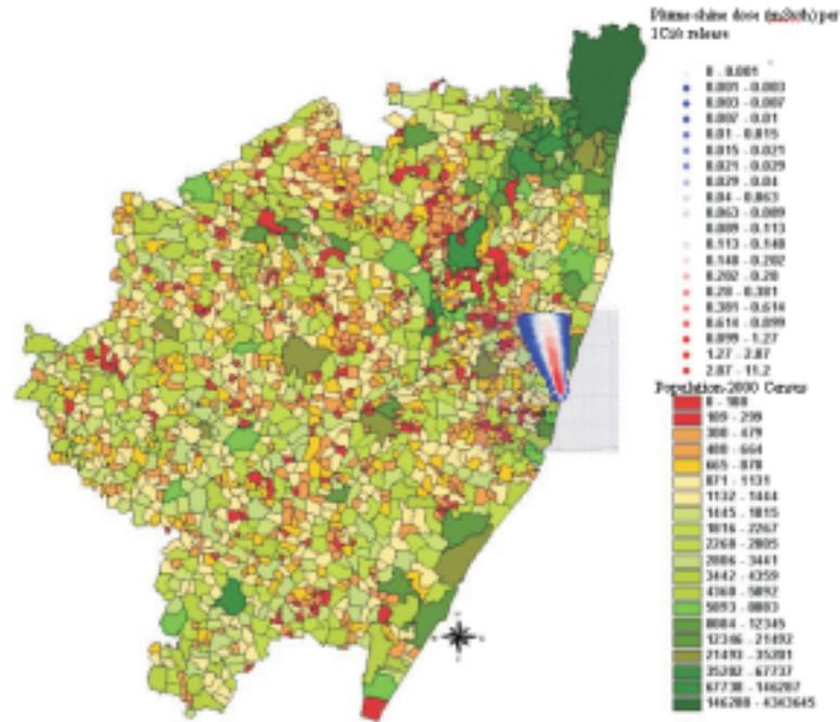
Fig.5. The Decision Support system using GIS and local cadastral database. Figure shows the village boundary map of Kanchipuram dist on which simulated air borne plume is over-laid.
