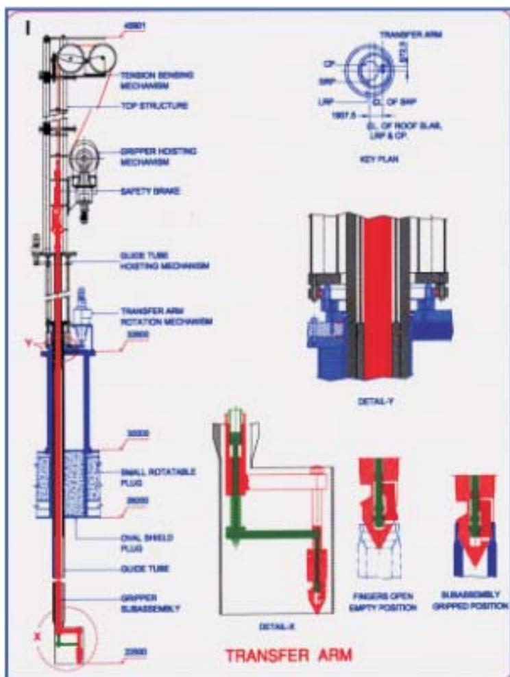
Fig 1: General Assembly of Transfer arm
