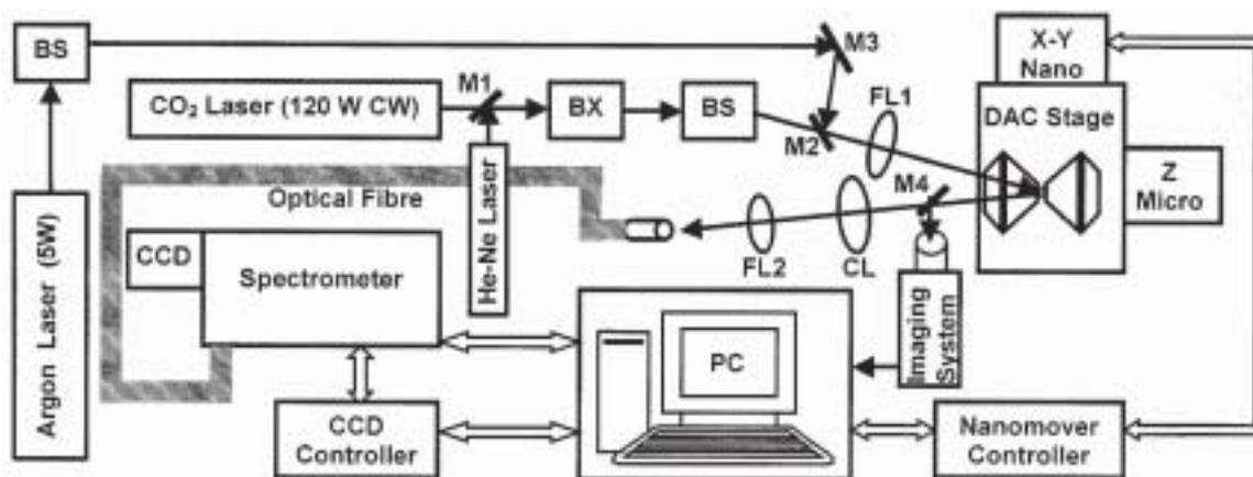
Fig 1: Schematic of the LHDAC set-up; M1, M2, etc.: Mirrors; BS: Beam Steerer; BX: Beam Expander; FL1 and FL2: Focussing Lenses; CL: Collecting Lens;
