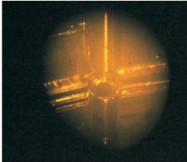
Fig.3 Siphon Break Pipe and the reflection of its open end in sodium
