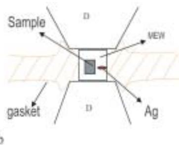
Fig1: (a) DAC mounted in pressure cell holder. (b) Schematic of sample assembly for HPXRD. D stands for diamonds mounted on cylinder and piston, sample and Silver loaded in the gasket hole of  $\Phi \sim 200 \mu\text{m}$ , MEW stands for Methanol Ethanol and Water mixture.
