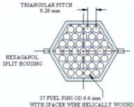
Fig.2: Crosssection of 37 pin subassembly
