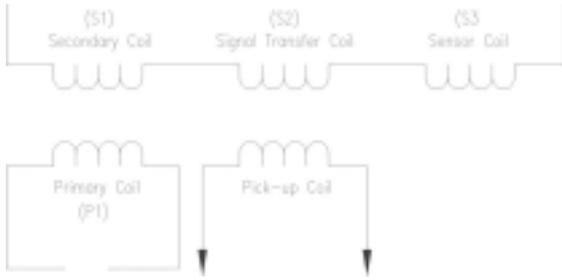
Fig. 1 : ECPS Circuit Configuration
