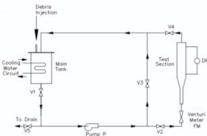
Fig.1 Schematic layout of experimental loop
