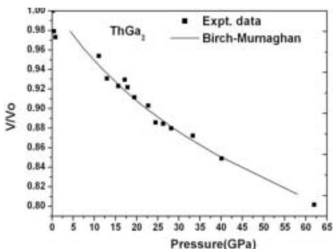
Fig. 3:  $V/V_0$  vs pressure. Birch Murnaghan equation of state is used to carry out curve fitting.
