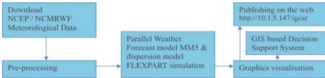
Fig. 2: Major components of the simulation system
