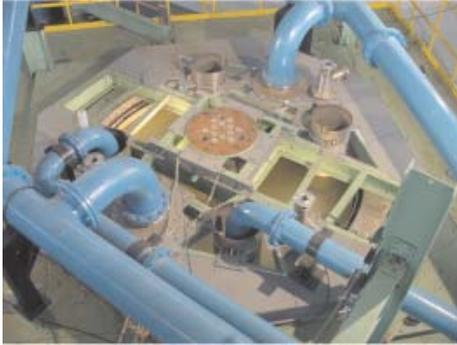
1/4 Scale Model of Reactor Assembly of PFBR
