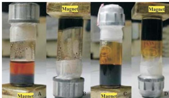
Fig 3: Photograph of magnetite (nanoparticles of average diameter of 6.5 nm) based ferrofluid under magnetic field (i) unstable (A&B) (ii) stable ferrofluid (C&D).
