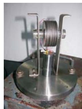
Fig. 4 : A prototype on-line transformer oil monitoring probe.
