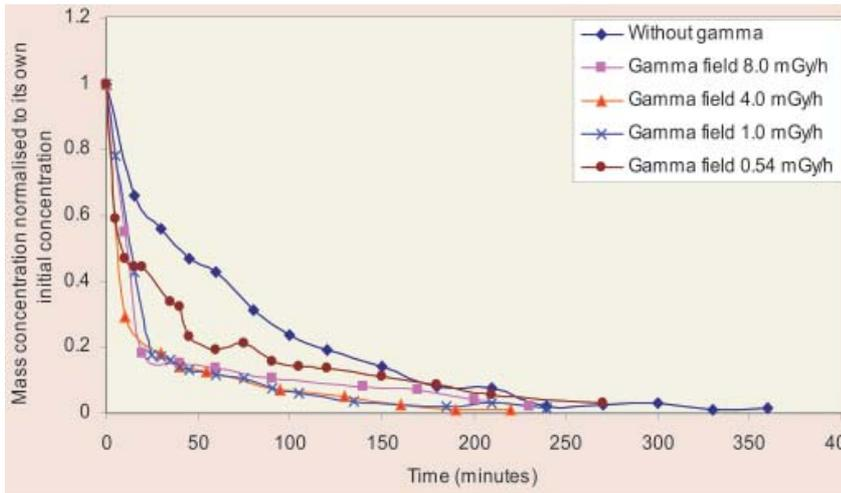
Fig.5: Depletion of suspended sodium compound aerosol mass concentration with time under gamma field
