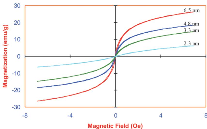
Fig 2: The magnetization curves of samples prepared at different ethanol-water ratio
