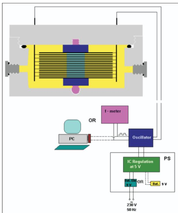
Fig. 1 : Schematic representation of the oil monitoring device.
