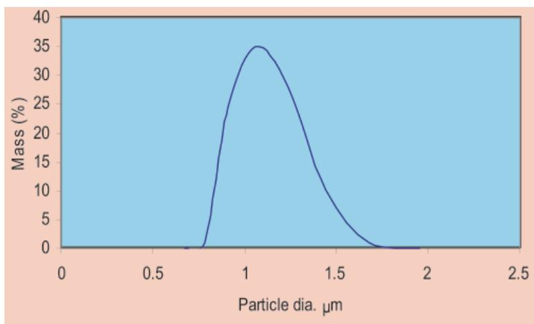
Fig.2 The initial Mass-size distribution (20s) of sodium compound aerosols for the ignition temperature of  $550 \text{ }^\circ\text{C}$  at 50%RH measured by Mastersizer.
