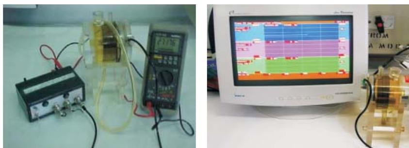
Fig. 2 : a) A typical pulsating sensor based transformer oil field monitoring kit. b) A PC based data acquisition system for the oil monitoring device.
