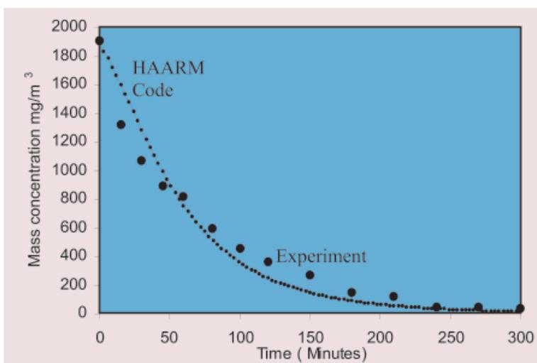
Fig.4: Depletion of suspended sodium compound aerosol mass concentration with time in the absence of gamma field
