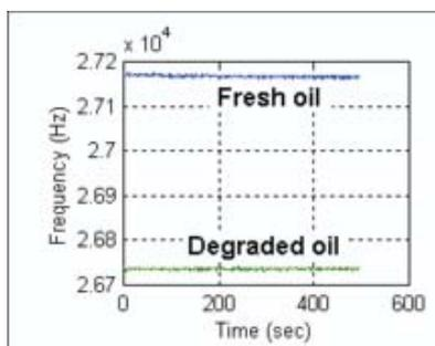
Fig. 3 : Pulse frequencies recorded as a function of time for fresh oil and a sample of service oil.
