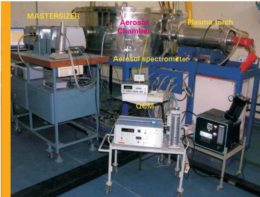
Fig.1 Photograph of Aerosol Test Facility showing plasma torch, aerosol chamber and aerosol diagnostic equipments.
