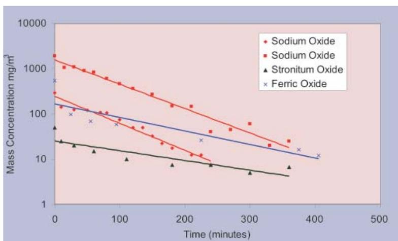
Fig.3 The depletion of mass concentration of sodium compound aerosol along with  $Fe_2O_3$  and  $SrO_2$  aerosols
