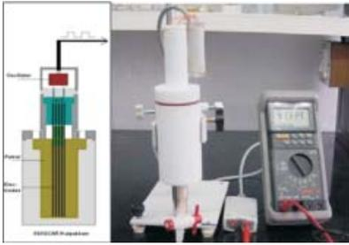
Fig. 5: The schematic diagram with a photograph of the portable field monitoring kit for assay of ethanol in petrol.
