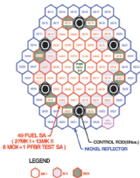
Fig. 1 : Core configuration for 14<sup>th</sup> irradiation campaign
