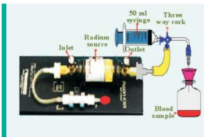
Fig 1. Irradiation of Blood sample using the Radon Source
