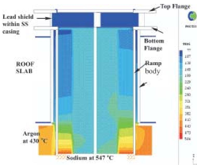
Fig. 3: Temperature distribution in IFTM at Roof Slab
