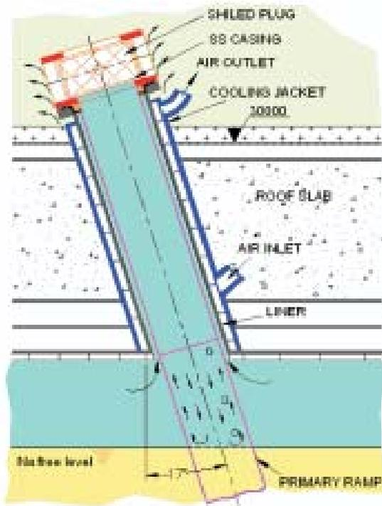
Fig. 1: Schematic of IFTM at Roof Slab
