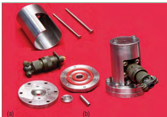
Figure 6: (a) Various parts and (b) assembly of sealing arrangement
