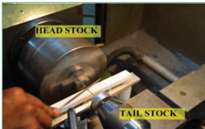
Figure 4: Precision machining in lathe to reduce the wire diameter
