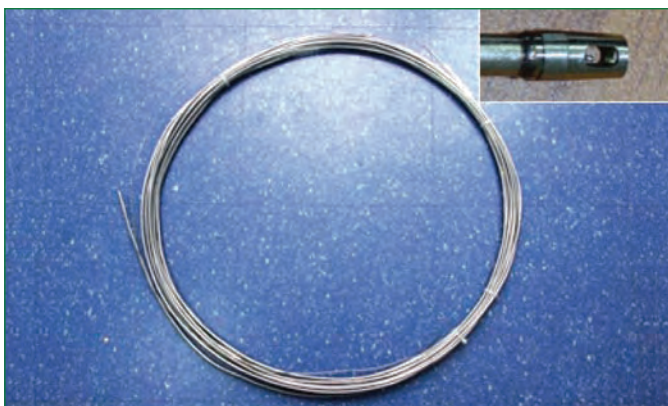
Figure 2: Sensor with 24 meters long mineral insulated cable and stainless steel thin walled tube; stainless steel protection cap is shown in insert
