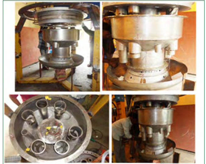
Figure 5: Photographs of thermocouples being fixed in the model
