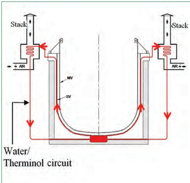
Figure 4: Schematic of safety vessel cooling arrangement for liquid coolant
