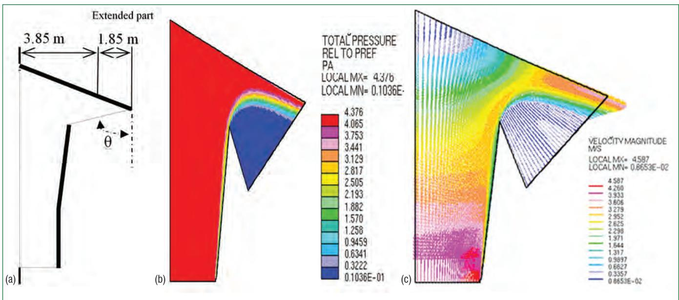
Figure 2: a) Schematic of the hood with extended roof design, b) Pressure distribution in extended roof design, c) Velocity distribution in extended roof design
