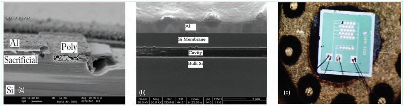
Figure 3: Cross-sectional SEM image of a single cMUT cell (a) showing the non-removal of sacrificial layer (Surface Micromachining method) (b) showing cavity properly etched out (Wafer Bonding method). However, cavity height appears to be less than the designed value (c) Diced and packaged 5×5 arrays of cMUT device
