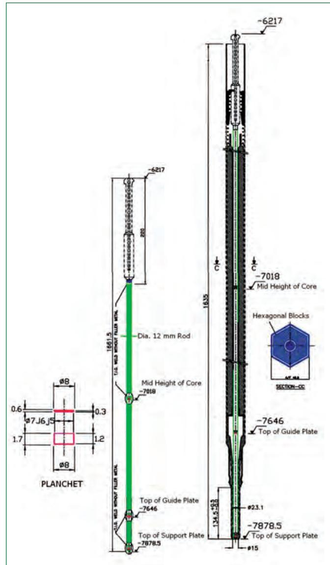
Figure 4: Special subassembly with capsule to measure the fast flux at the Grid Plate locations using Np foils.
