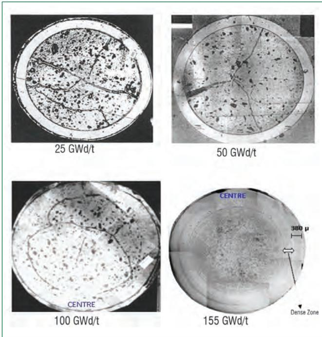
Figure 2: Fuel pin cross-section by PIE at different burnups
