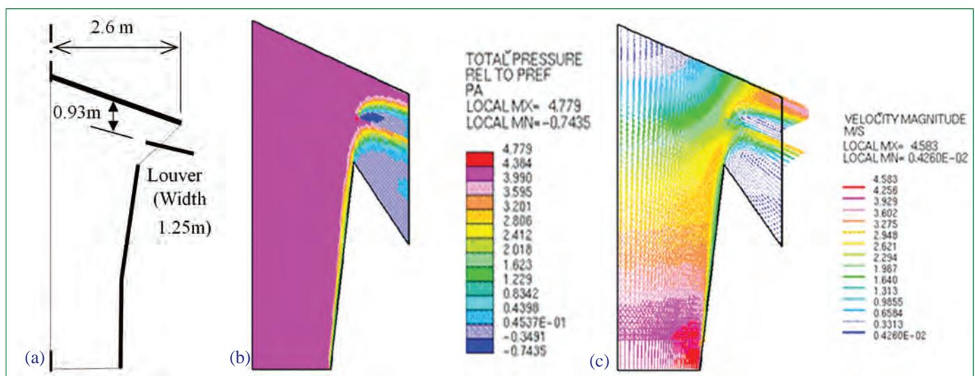
Figure 3: a) Schematic of the hood with additional louver, b) Pressure distribution due to addition of louver, c) Velocity distribution due to addition of louver
