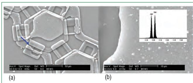
Figure 5: (a) SEM image of the (a) cMUT cell and (b) Al electrode and Si interface. It is clear from these figures that top Al electrode of the fabricated device is not centered. Also several micro cracks are seen and are shown by blow arrows.
