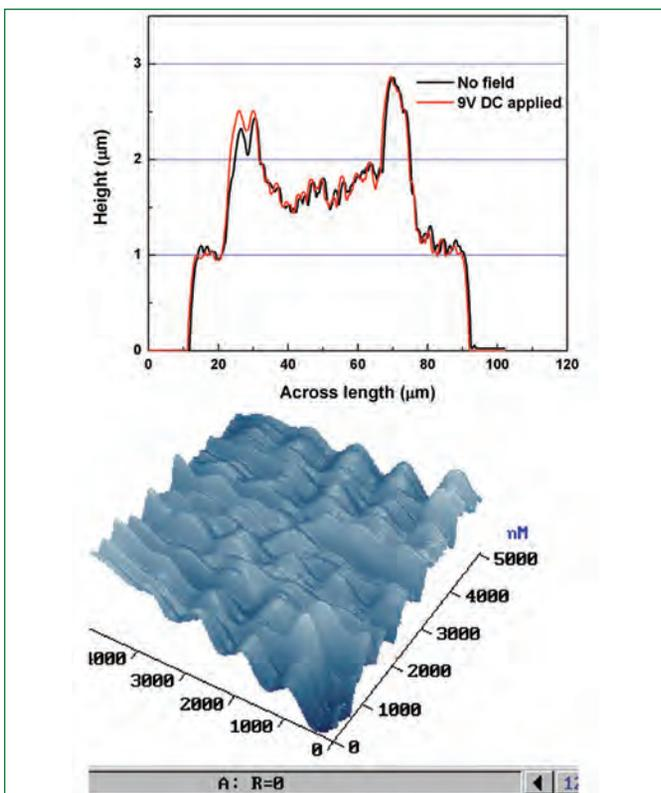
Figure 4: Surface line profile of (a) single cMUT cell with and without DC voltage and (b) surface morphology of cMUT cell.
