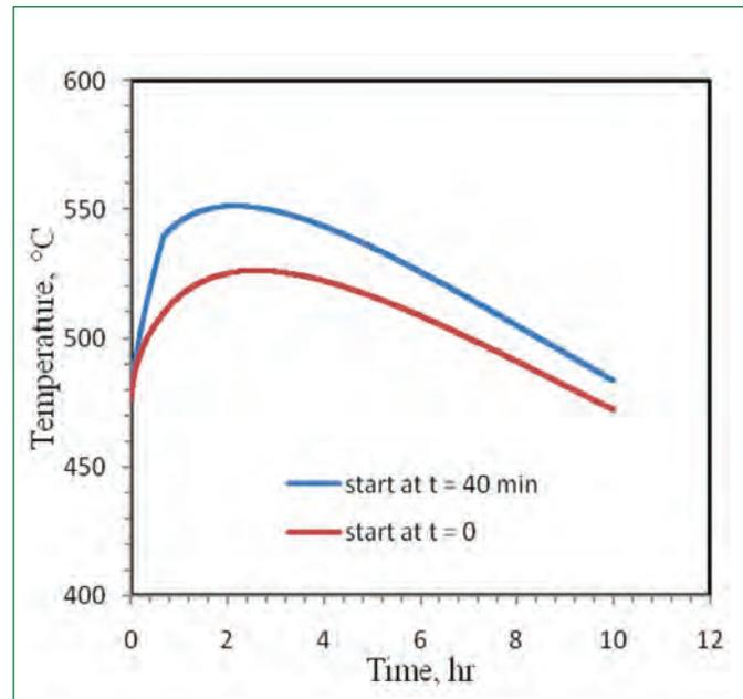
Figure 5: Evolution of sodium pool temperature with heat removal by vessel cooling system
