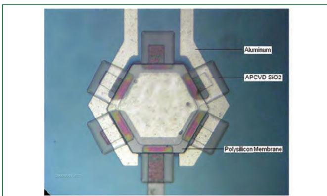
Figure 2: Single element of cMUT device with poly silicon membrane and aluminum coated top electrode.
