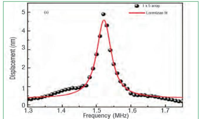
Figure 6: Frequency response of single cMUT cell measuring using NVA.
