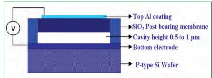
Figure 1. Schematic diagram of a single cMUT cell.
