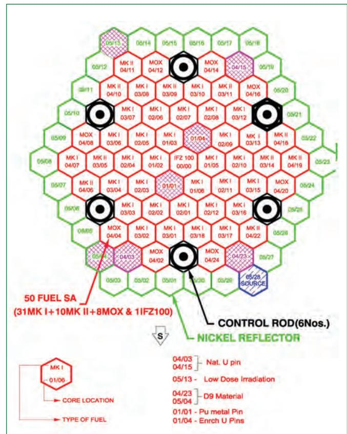
Figure 3: Core configuration for 23<sup>rd</sup> Campaign
