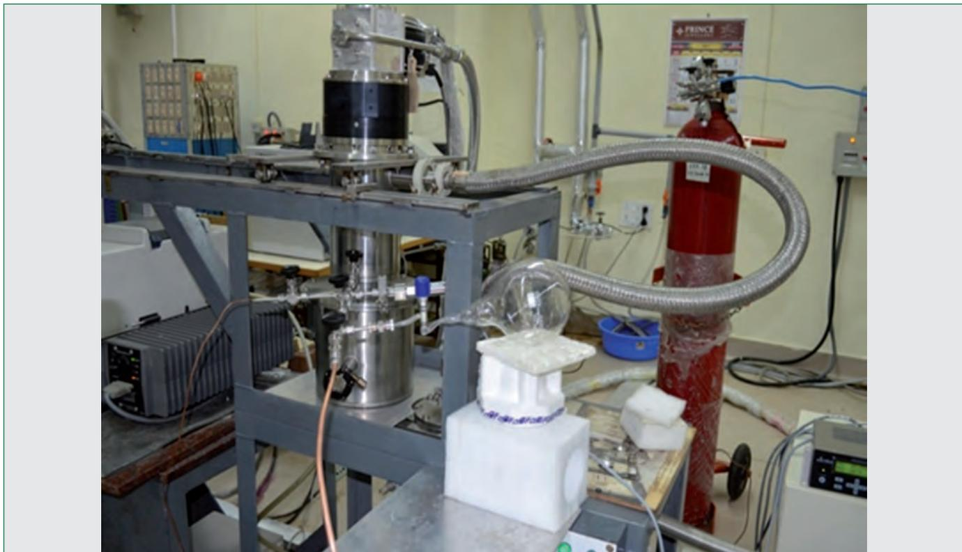
Figure 2: Photographs showing the p-H<sub>2</sub> generation set-up
