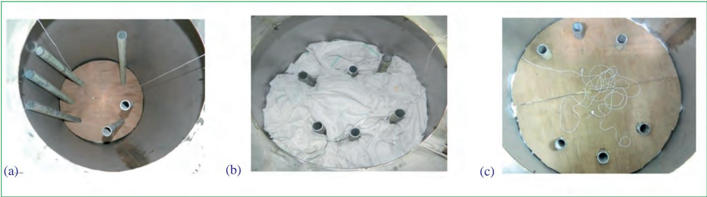
Figure 2: Simulated stainless steel waste drum filled with (a) six stainless steel rod, wooden plate at the bottom (b) cotton waste around the stainless steel tube and (c) wooden plate at the top
