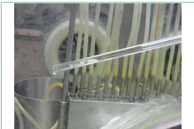
Figure 5: Crud formed during Mixer-Settler runs
