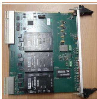
Figure 9: 3 Channel synchro to digital converter board
