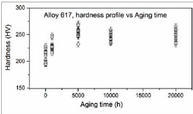
Figure 2: The hardness profile of Alloy 617
