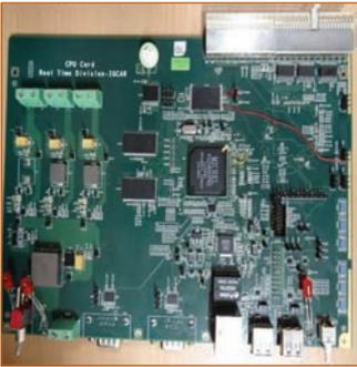
Figure 3: ARM9 Processor based CPU board
