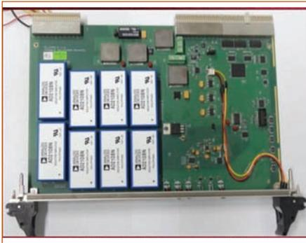
Figure 13: 8 Channel thermocouple input board
