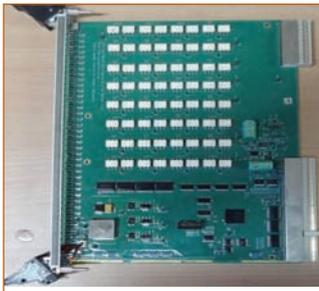
Figure 7: 32 Channel digital output board
