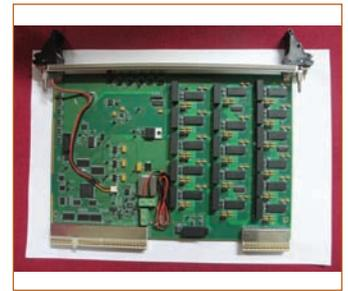
Figure 12: 16 Channel leak detector board
