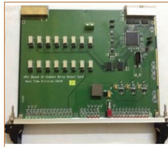
Figure 8: 16 Channel relay output board
