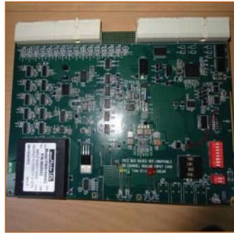
Figure 4: 30 Channel analog input board
