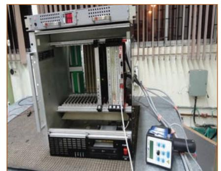
Figure 18: Pre-EMI/EMC test setup
