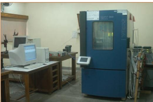
Figure 16: Environmental test chamber
