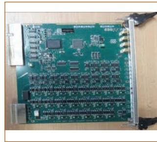
Figure 11: 4/12/4 Channel counter timer board
