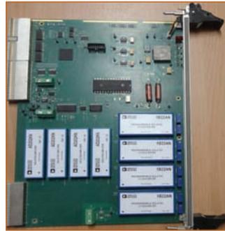
Figure 5: 4 Channel analog output board
