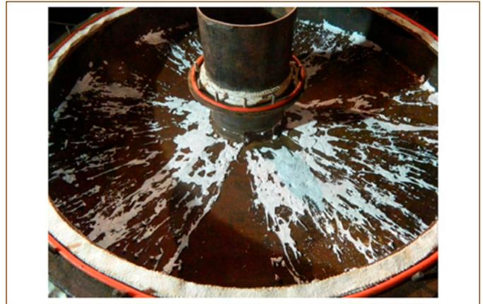
Figure 10: Ejected sodium without insulation
