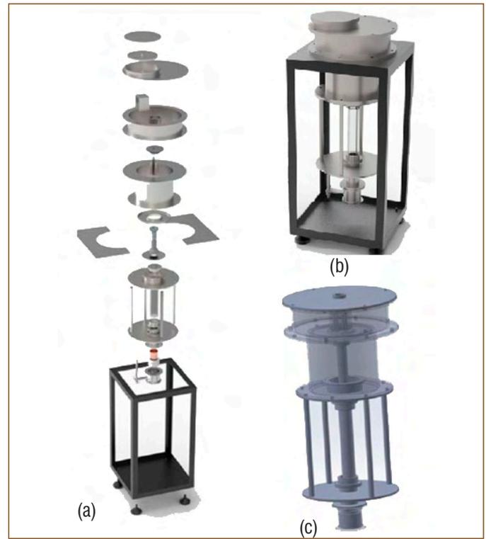
Figure 3: (a) Exploded diagram (b) Schematic diagram (c) Transparent view of drop calorimeter.
