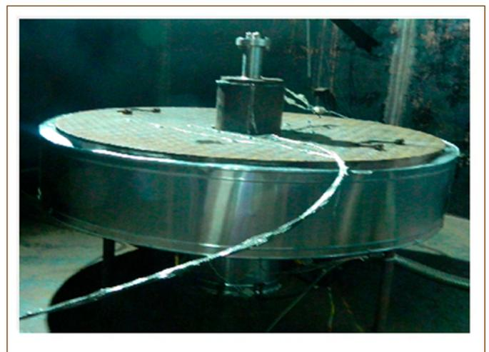
Figure 3: Simulation of roof slab-LRP leak path
