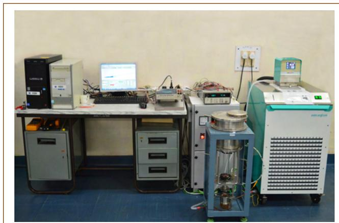
Figure 1: Photograph of in-house developed drop calorimeter.
