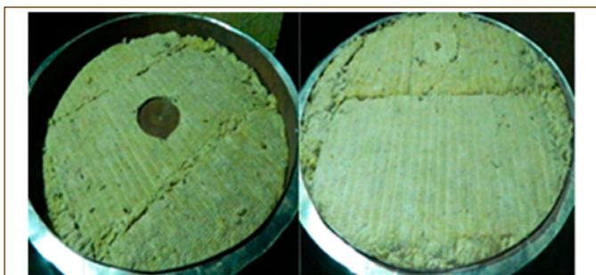
Figure 5: Packing of insulation around leak path
