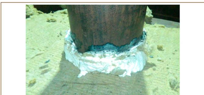
Figure 9: Ejected sodium around the radial gap of leak path
