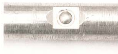
Fig. 2 : View of rupture disc after bursting
