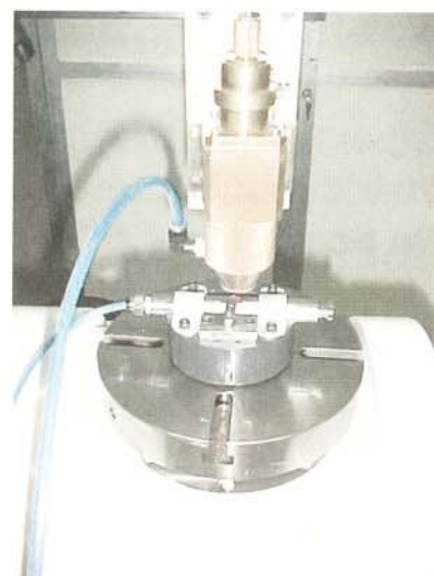
Fig. 1 : Tube and rupture disc positioned on the CNC rotary table for welding.
