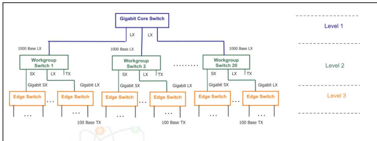
Figure1: Upgraded Setup of Campus Backbone Network with Gigabit Technology
