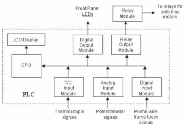
Fig. 4: DMD Controller Block Diagram
