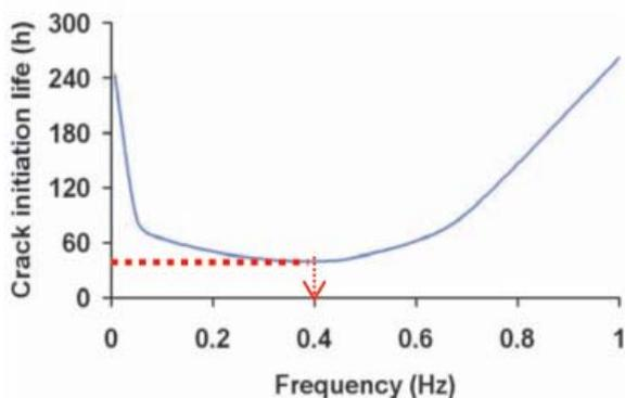
Fig.6: Concept of critical frequency
