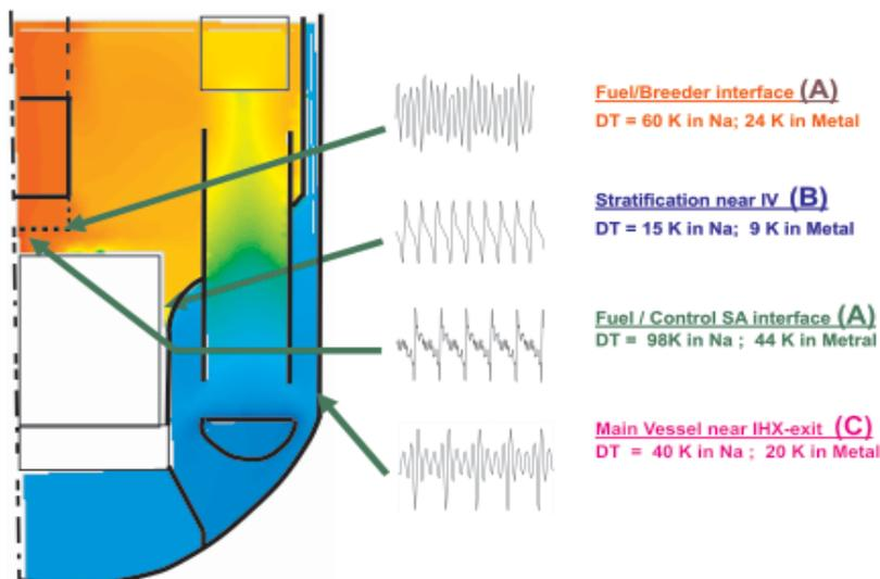
Fig.8: Thermal stripping zones and temperature fluctuations in hot and cold pools of PFBR
