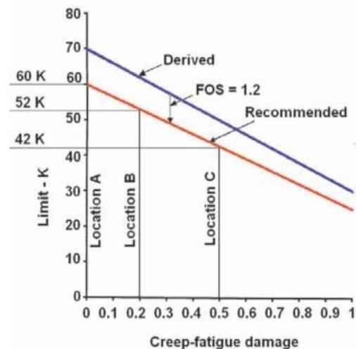
Fig.7 Thermal striping limits for PFBR
