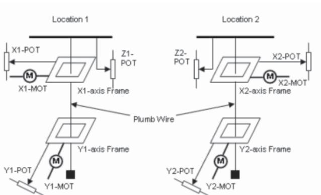
Fig. 3: Diagram of Reactor Vessel Displacement Measuring Device
