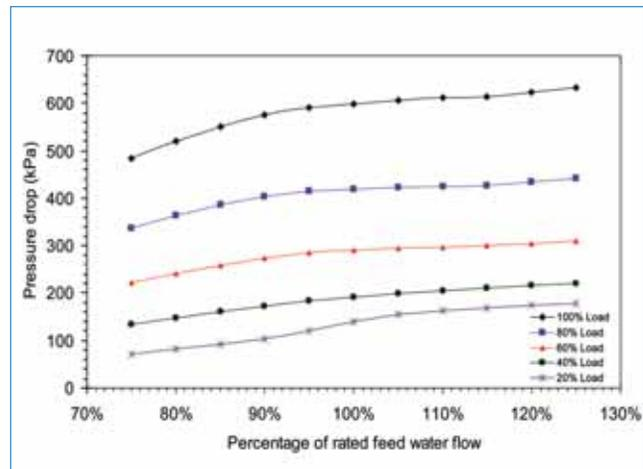
Figure 7: Variation of pressure drop as function of feed water flow rate
