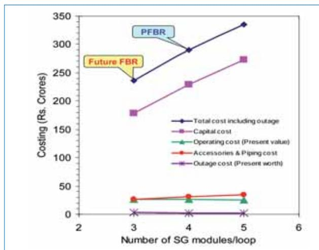
Figure 4: Variation of cost as function of total number of steam generators
