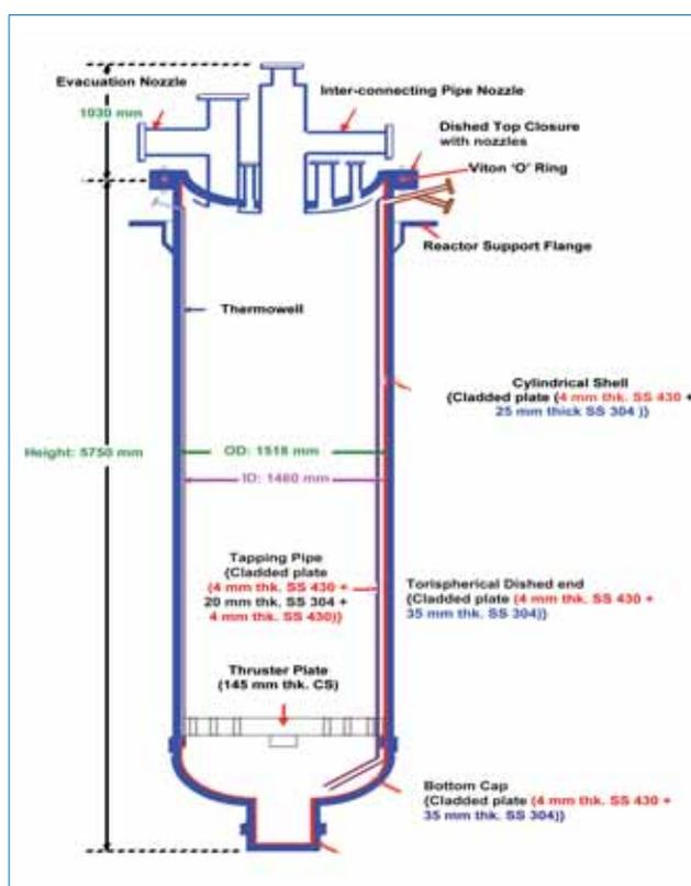
Figure1: Schematic of the Clad SS 304 / SS 430 Reactor (assembled) for KMML's 500 tonnes per annum titanium sponge
