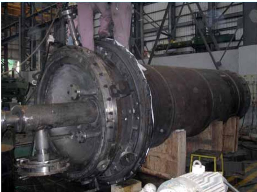
Figure 2: Cladded Reactor for Titanium Sponge Production
