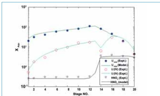
Figure 3: Comparison of calculated and experimental data on uranium reduction in a 20-stage electrolytic mixer settler
