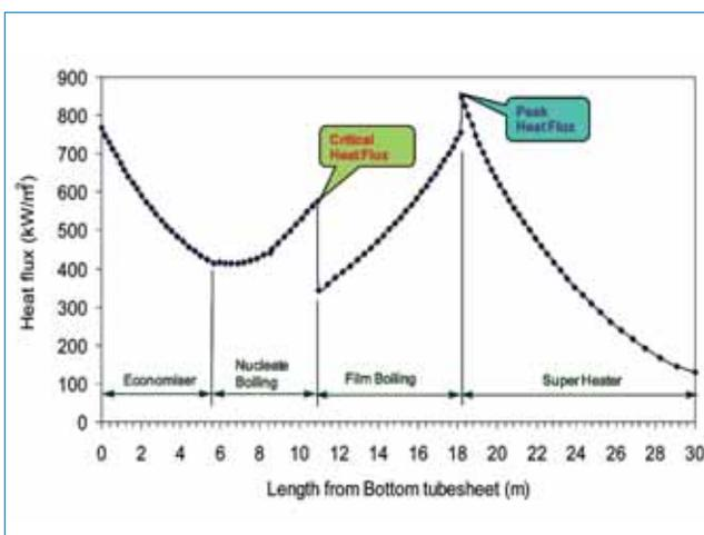
Figure 6: Variation of heat flux along the tube length
