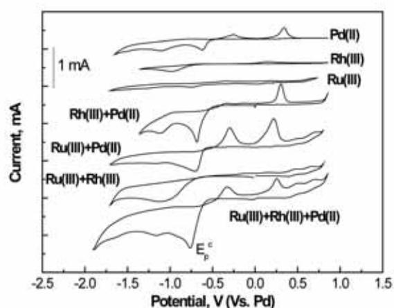
Figure 4: Cyclic voltammogram of 60mM each Ru(III), Rh(III), and Pd(II) in bmimCl and their equi-molar mixtures in bmimCl recorded at a glassy carbon working electrode. Counter electrode: glassy carbon, Quasi-reference palladium wire. T:373 K
