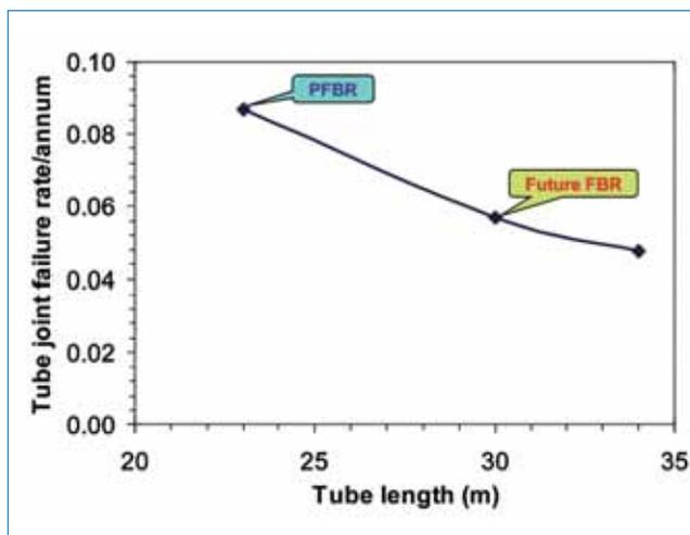
Figure 3: Variation of tube joint failure as a function of tube length
