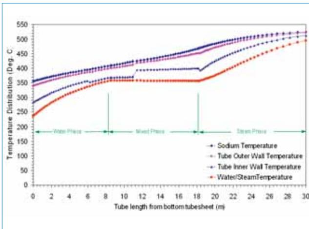
Figure 5: Temperature distribution with variation of tube length
