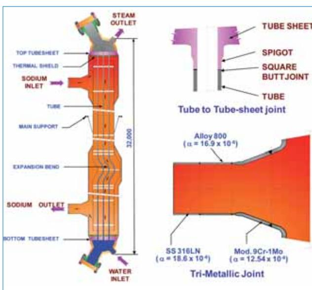
Figure 1: Integral once through steam generator for future FBRs
