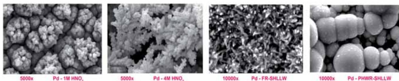
Figure 2: SEM images of palladium deposited from 1M and 4M nitric acid and Fast Reactor-Simulated High Level Liquid Waste and PHWR-Simulated High Level Liquid Waste solutions. Working electrode: stainless steel, counter electrode: platinum, quasi-reference electrode: Pd wire. T: 298 K. Duration of electrolysis: 8 hours. Applied cathodic potential:  $-0.5$  V (Vs. Pd)
