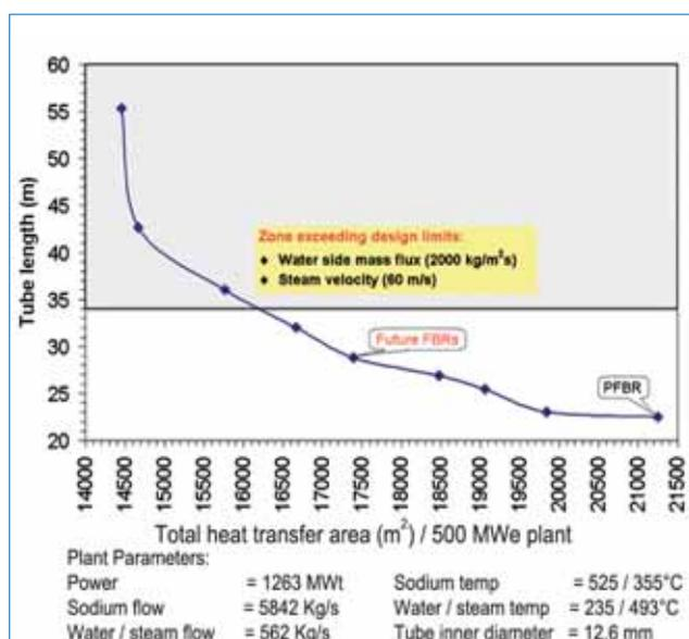
Figure 2: Variation of total heat transfer as a function of tube length
