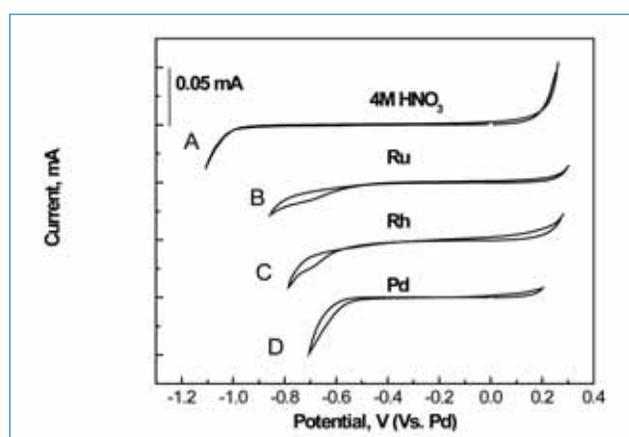
Figure 1: Comparison of cyclic voltammogram of 4 M nitric acid and Ru(III), Rh(III), Pd(II) in 4 M  $\text{HNO}_3$  recorded at stainless steel working electrode. Counter electrode: platinum, Quasi-reference electrode: palladium wire. Scan rate:  $0.01 \text{ Vs}^{-1}$  T:298 K
