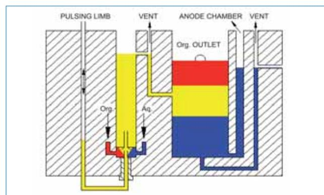
Figure 2: Schematic of one stage of mixer-settler bank
