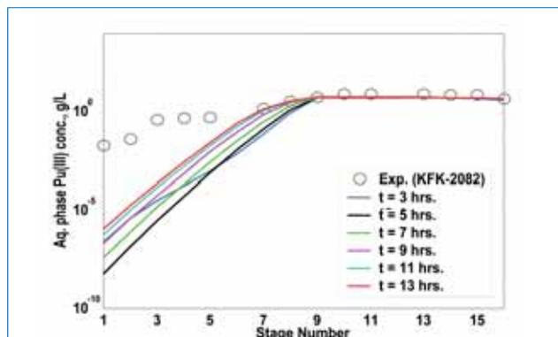
Figure 4: Comparison of experimental and calculated profile of Pu(III) in 16-stage 1B contactor (KFK-2999)
