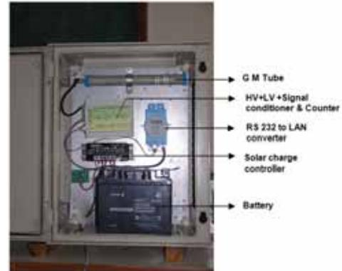
Figure 1: Schematic of the indigenous on-line gamma dose logger
