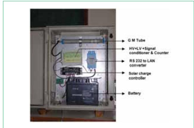
Figure 1: Schematic of the indigenous on-line gamma dose logger
