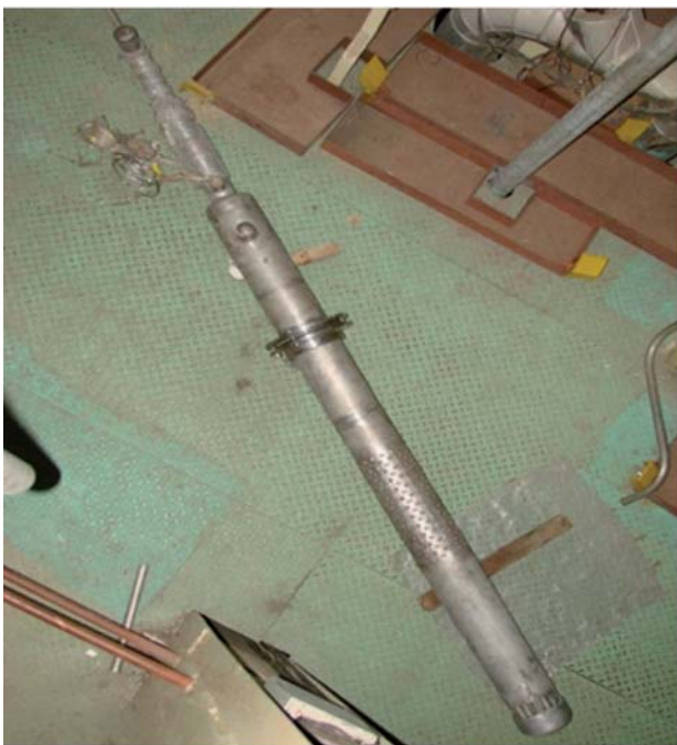
Figure 3: View of decay heat exchanger before erection
