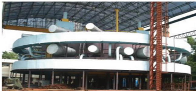
Figure 6: Full scale top shield layout mockup
