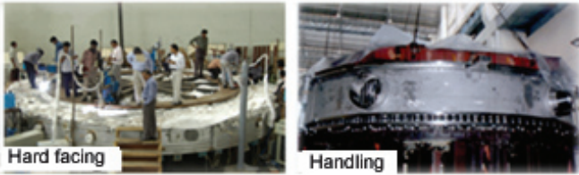
Figure 2: Manufacturing stages of grid plate
