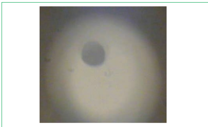
Figure 2: Full spot at the melting temperature of zirconium
