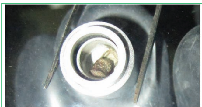
Figure 4: Mark I Mixed carbide fuel pellet of FBTR after melting and solification
