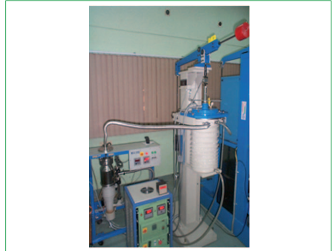
Figure 1: Impression creep testing machine developed at IGCAR
