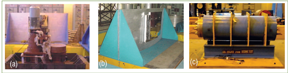
Figure 5: (a) Rotatable plug gear boxes (b) safety vessel insulation panel and (c) PFBR electrical penetration assembly
