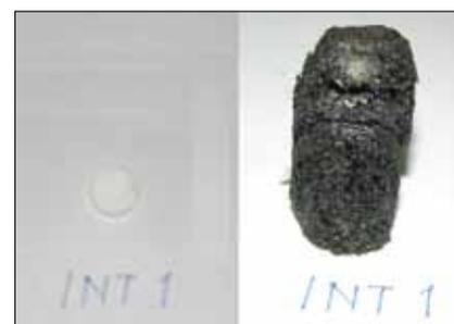
**Fig. 2** Intumescence on heating
