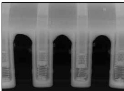
**Fig. 1** Gamma radiograph of dislocated orifice assemblies
