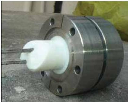
**Fig. 1** Photograph of a typical conductance probe mounted vertically in test section of SF
