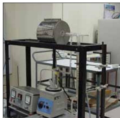
**Fig. 1** Photograph showing the apparatus used for carrying out pyrohydrolysis
