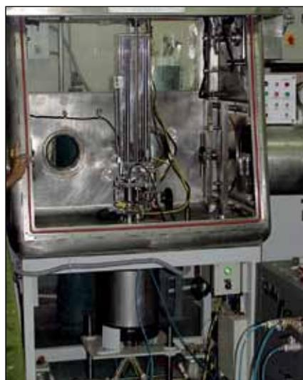
Fig. 1 Dilatometer assembly
