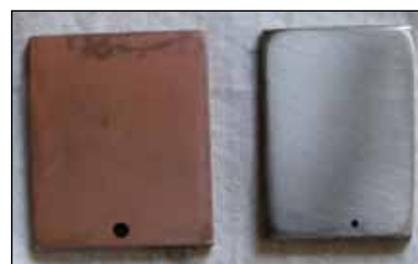
**Fig. 1** Titanium surface with and without copper coating
