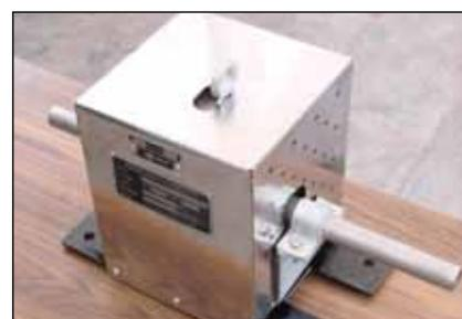
Fig. 1 20 NB SmCo permanent magnet flow meter
