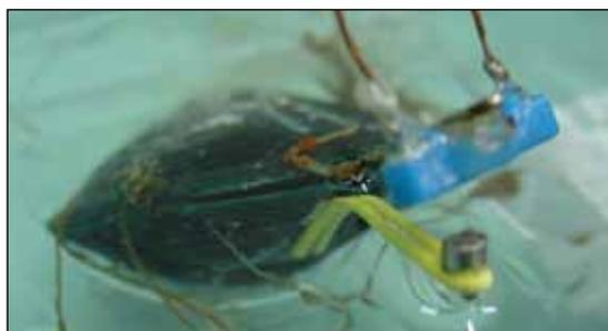
**Fig. 1** Open-close detection system deployed on a mussel
