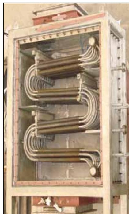
Fig. 2 Air heat exchanger in the side plate opened condition
