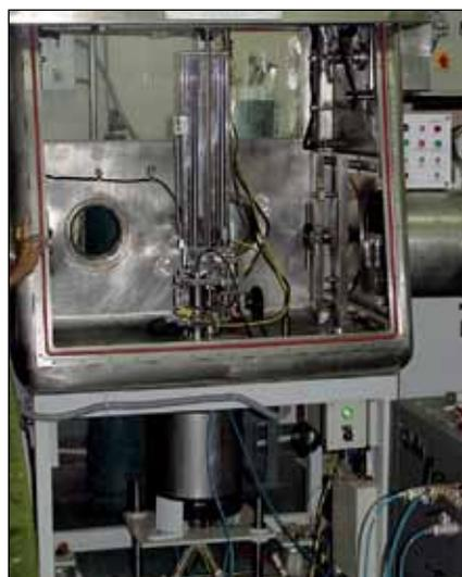
Fig. 1 Dilatometer assembly
