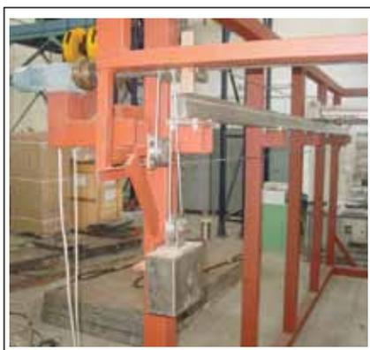
**Fig. 1** View of the wire rope tensioning arrangement
