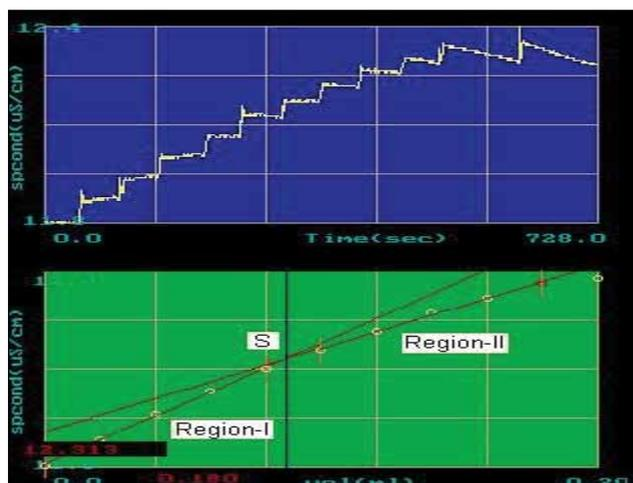
**Fig. 3** A real time conductivity plot both in time and volume domain during addition of 1mM  $\text{AgNO}_3$  to 35 ml of 0.07 mM KCl in 20 micro litre steps
