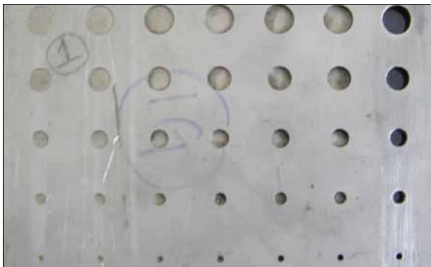
**Fig. 1** Photograph of samples with flat bottom holes
