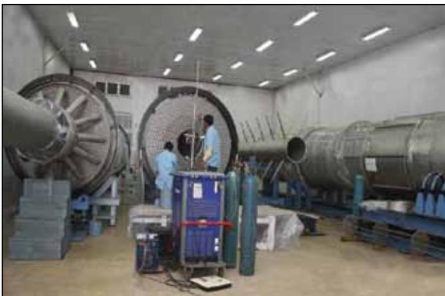
**Fig. 3** Intermediate heat exchanger
