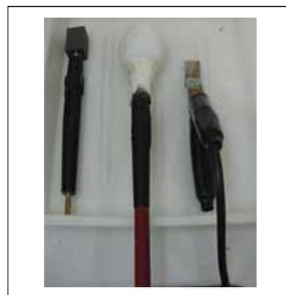
**Fig. 1** Photograph of electrochemical brush developed
