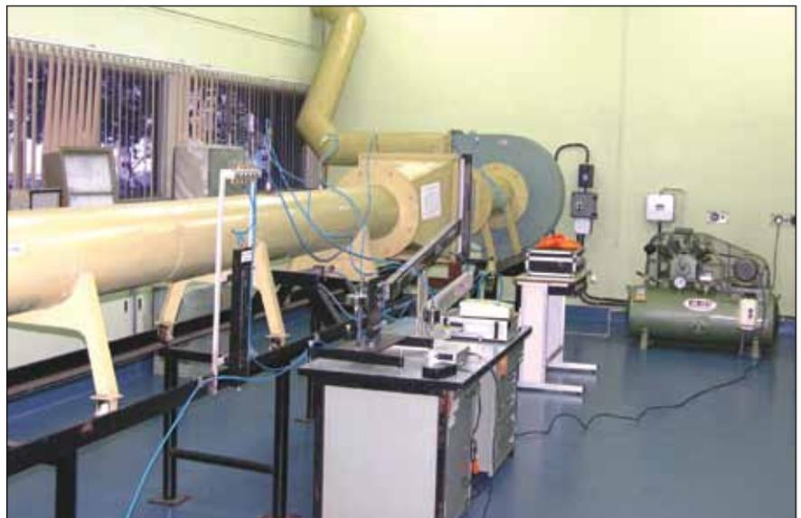
**Fig. 1** HEPA filter testing rig
