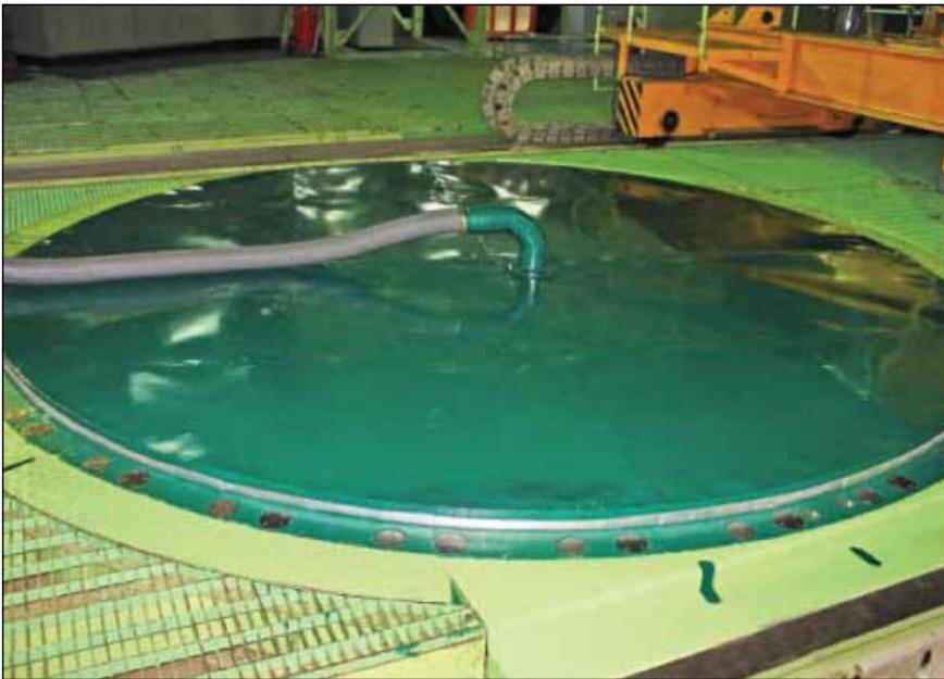
**Fig. 2** *Metallic shroud (cocoon) over the block pile*
