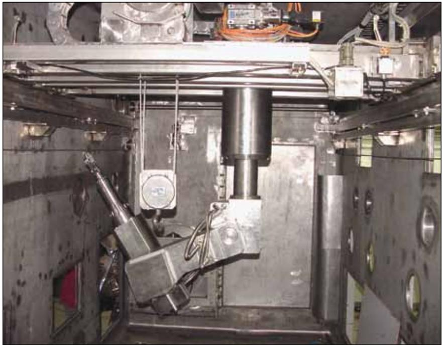
**Fig. 4** In-cell crane with power manipulator installed in the containment box
