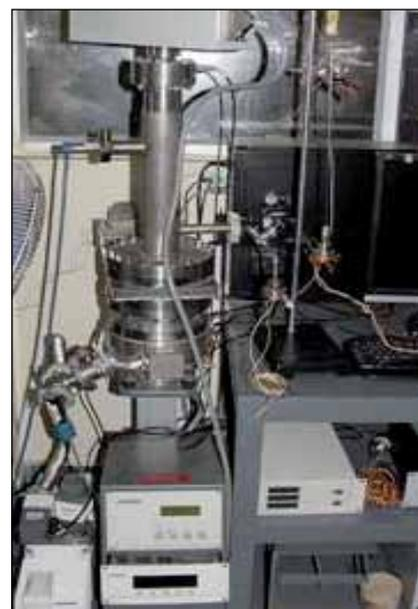
**Fig. 6** Quadrupole mass spectrometer based facility for understanding analyte – oxide interactions
