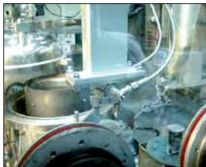
**Fig. 3** The sintering furnace housed inside a glove box
