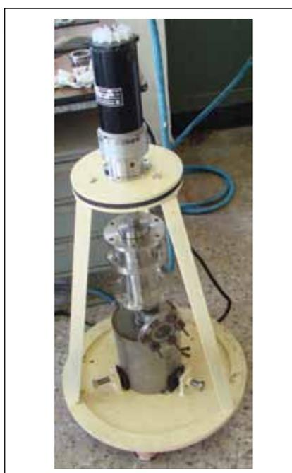
Fig. 1 Photograph of 25 mm diameter shaft seal setup
