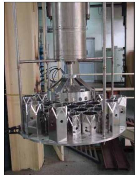
**Fig. 2** Transducer holder with subassembly heads
