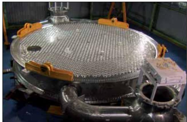
**Fig. 4** Integration of grid plate with primary piping
