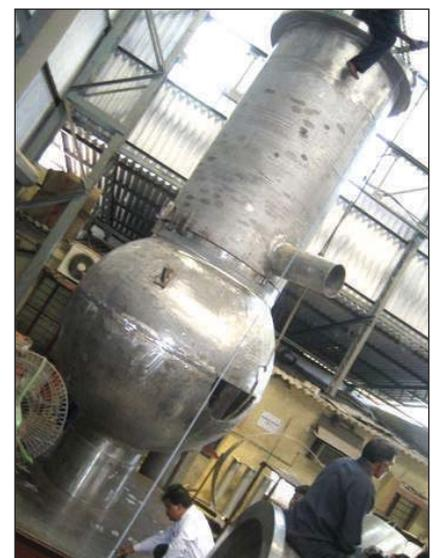
**Fig. 3** Secondary sodium pump spherical shell under manufacture
