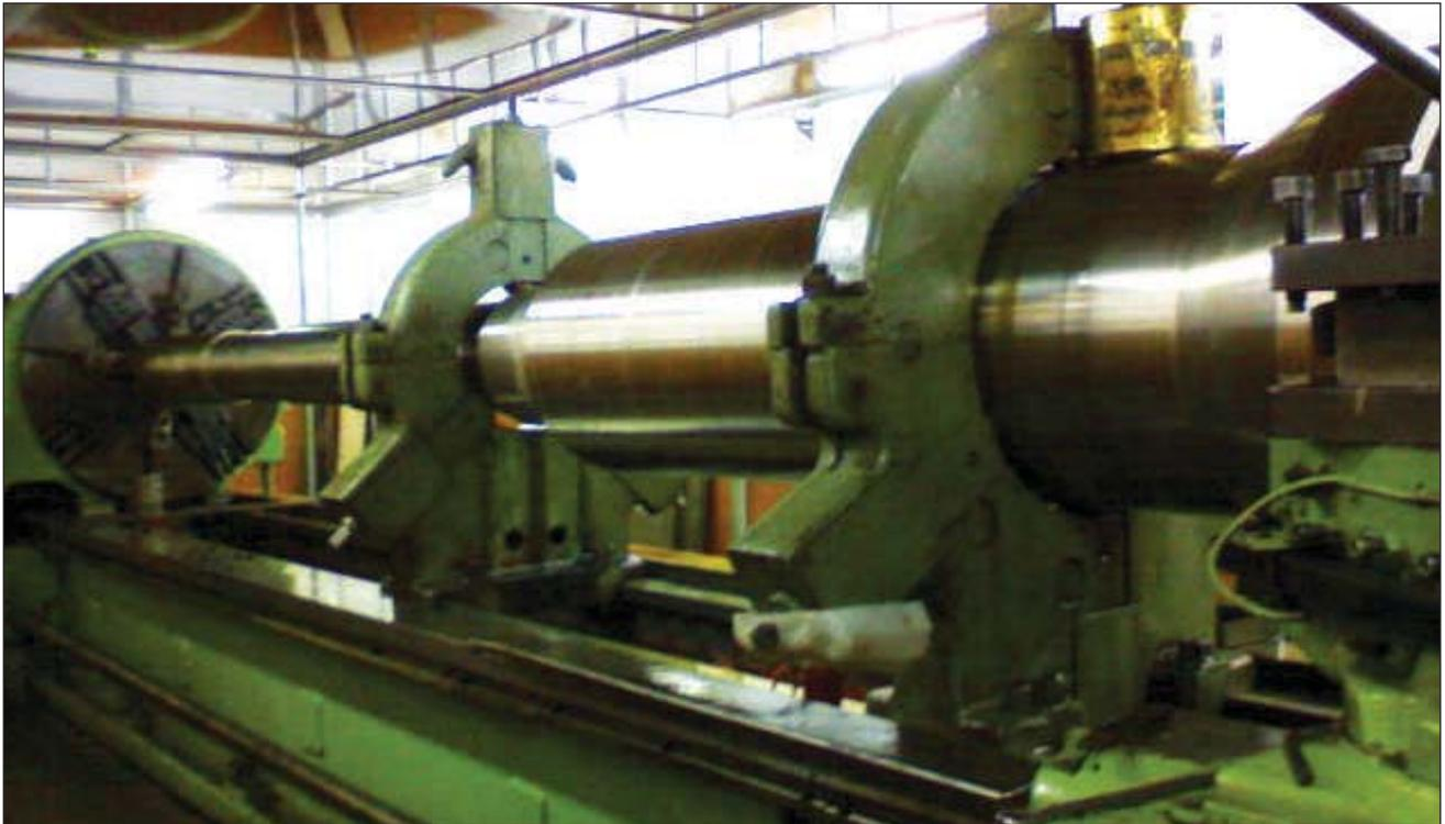
**Fig. 2** Machining of primary sodium pump shaft
