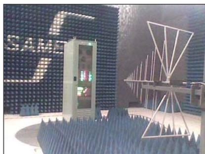
Fig. 2 Radiated susceptibility testing of PCSL system
