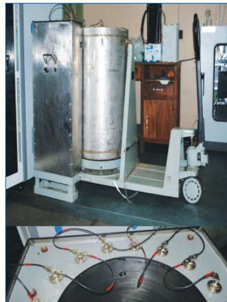
Fig. 1 Schematic view of assay including waste drum and detector assembly
