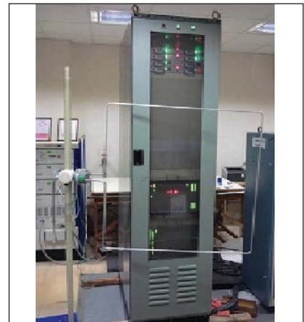
Fig. 1 Pulse magnetic field testing of SLFIT System
