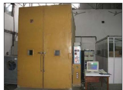
Fig. 3 Dry heat testing of SLFIT system inside walk in chamber
