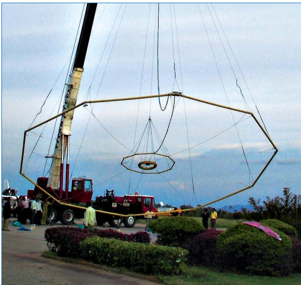
**Fig. 1** Structural integrity testing of airborne time domain electro-magnetic under-slung assembly
