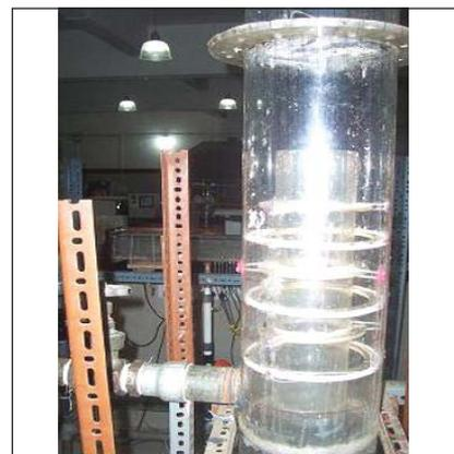
Fig. 1 1/5<sup>th</sup> scale model of the steam generator inlet plenum
