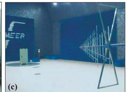
Fig. 2 (a) Environmental qualification RTU boards at our Centre (b) & (c) EMI/EMC qualification of RTU cabinet at SAMEER, Chennai
