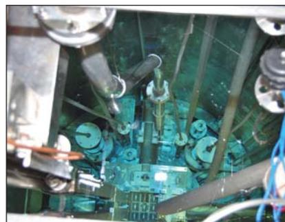
**Fig. 3** Compensated ion chamber being loaded into reactor through a dry tube
