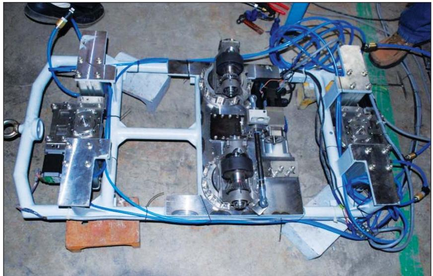
**Fig. 1** Drive transmission layout of the main ISI device
