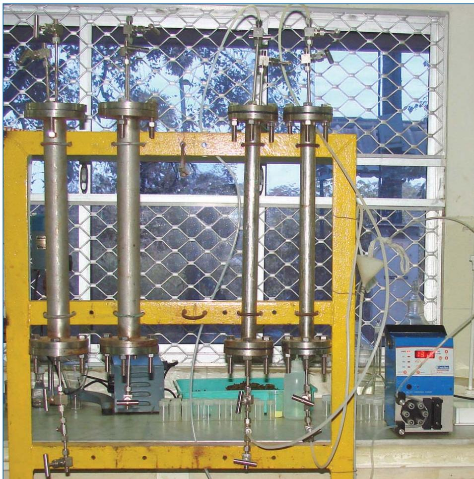
Fig.1 Pilot plant set up for cesium removal
