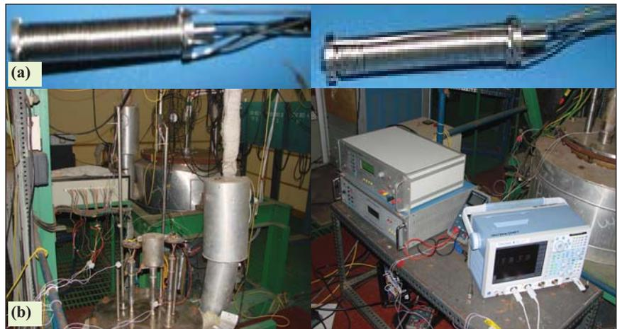
Fig. 2 (a) Fabricated sensor using mineral insulated cable (b) Experimental test facility for sodium testing of weir film thickness sensor
