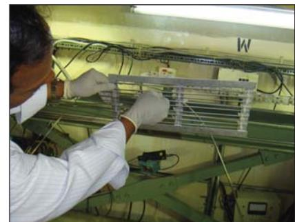
**Fig. 4** Assembly of self powered neutron detectors
