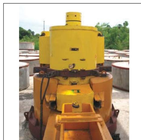
**Fig. 5** Alpha bearing high active solid waste transfer system
