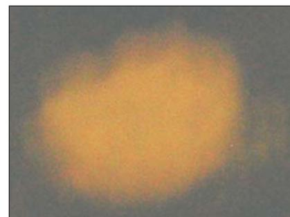
**Fig.2** Thermo luminescent emission of orange light from  $\text{Li}_2\text{B}_4\text{O}_7:\text{Mn}$  phosphor
