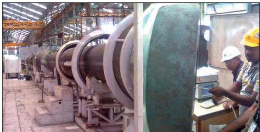
Fig. 1 Inspection of SG-A at the manufacturer's site
