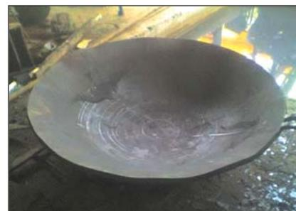
**Fig. 3** Bottom dished end, after first stage hot forming
