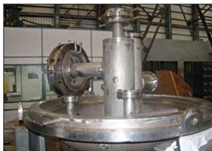
**Fig. 2** Top dished end of reactor
