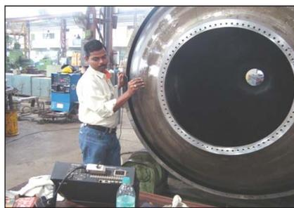
**Fig. 2** Silicon steel rocket motor casing being evaluated at WIL, Pune
