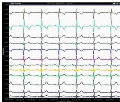
**Fig. 2** Thirteen Channel magneto-cardiogram recorded using the system
