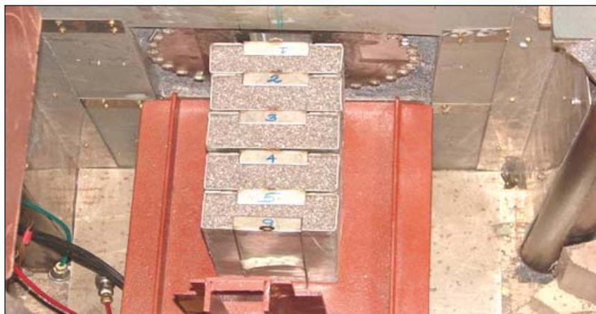
**Fig. 1** Arrangement of ferro boron filled boxes and foil holders at south beam of KAMINI
