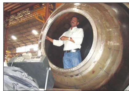
**Fig. 3** Maraging steel rocket motor casing being evaluated at WIL, Pune
