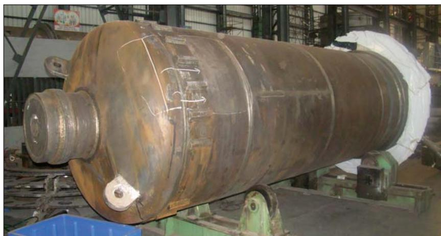
Fig. 1 Clad reactor for titanium sponge production.
