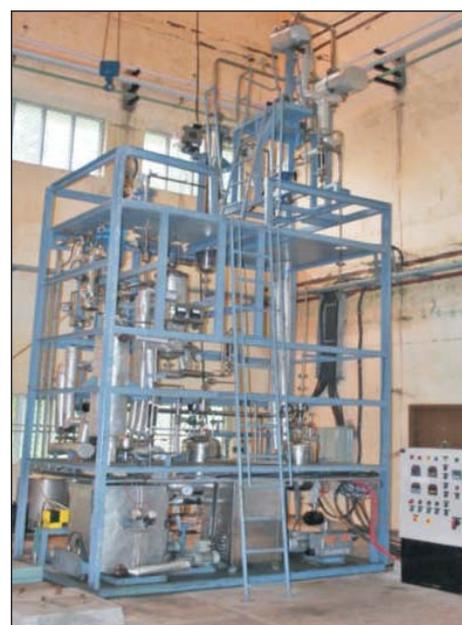
Fig.1 Pilot plant solvent purification system
