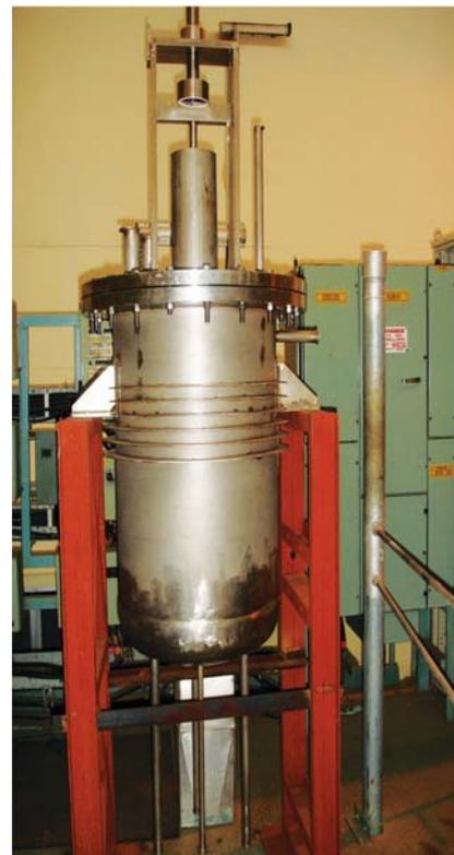
**Fig.1** Thermal striping test vessel assembly
