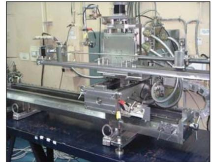
Fig.2 Four axis gamma scanning bench
