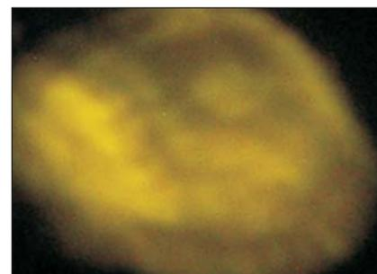
**Fig. 4** Thermo luminescent emission of pale green light from LMB:Tb phosphor
