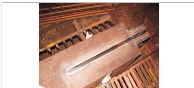
Fig. 7 Narrow groove for repair
