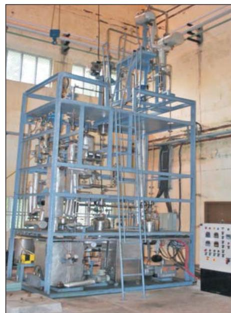
Fig.1 Pilot plant solvent purification system
