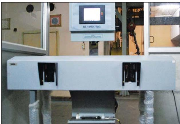
**Fig. 3** Alpha and beta hand cloth monitor
