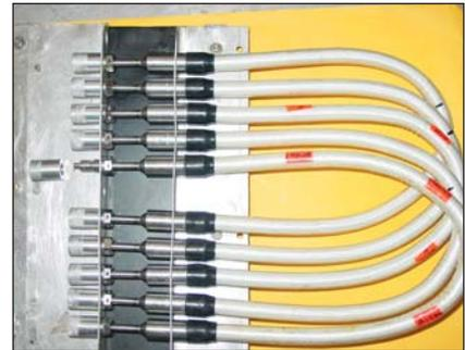
**Fig. 2** Pyro explosive transfer assembly
