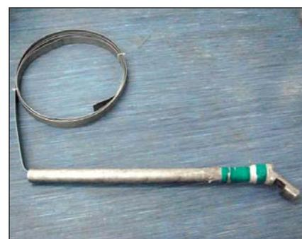
Fig. 4 Encapsulated (for 1m) wave guide with 10 m long strip
