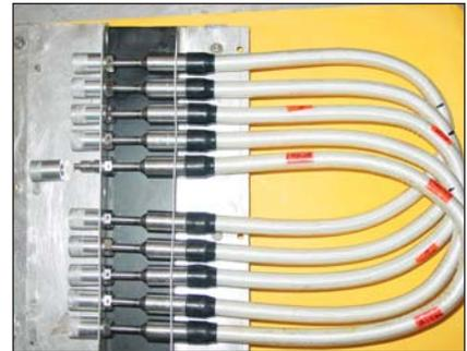
**Fig. 2** Pyro explosive transfer assembly
