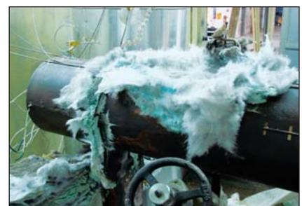
Fig. 3 Glass wool sticking to the surface of the pipe indicating the sodium leak track
