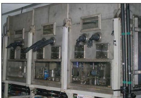
Fig. 1 Engineering scale demonstration facility for pyroprocessing studies
