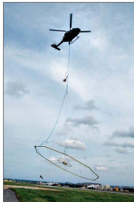
**Fig. 2** Phase-1 flight trials of the time domain electro magnetic system
