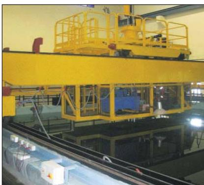
Fig.1 Water tank with moving platform
