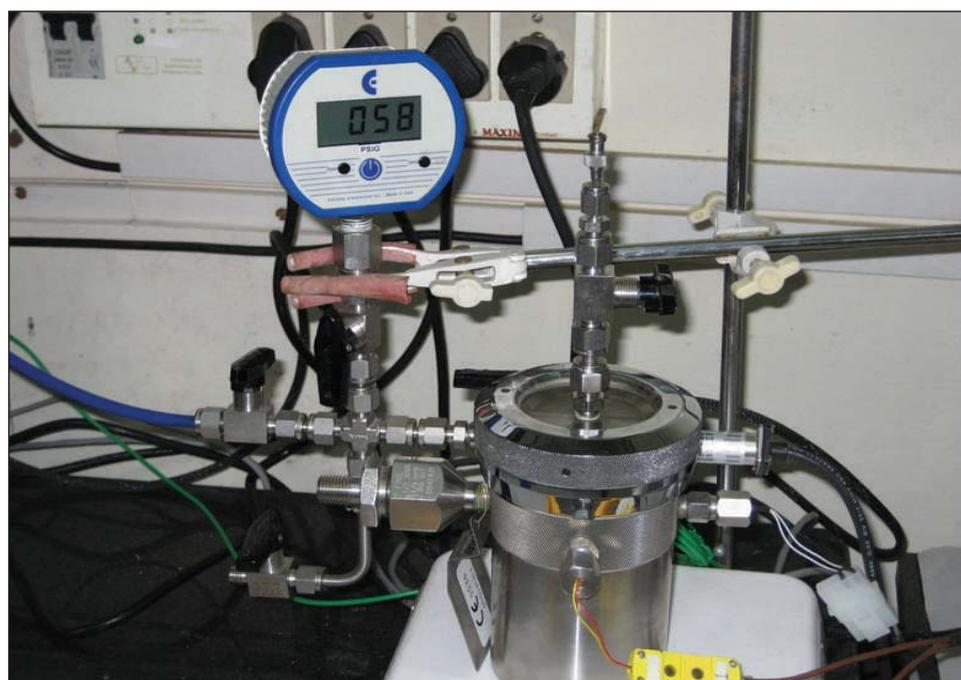
**Fig. 1** Adiabatic calorimeter setup
