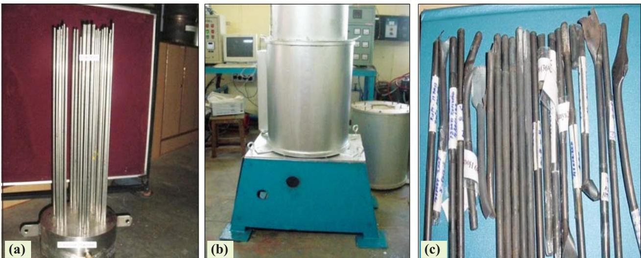
Fig. 1 Investigation of creep strength reduction factor for fuel pin end plugs: (a) Fuel pins welded to pressure chamber, (b) Pressure chamber enclosed in a furnace and (c) Ruptured fuel pins
