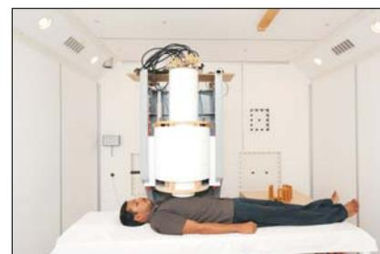
**Fig. 1** 13 channel SQUID based system for magnetocardiography
