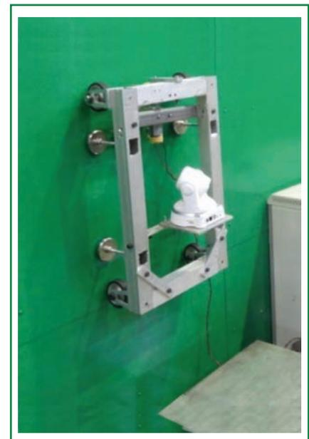
Fig. 6 Scaled-down prototype magnetic-coupled vehicle
