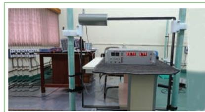
Fig. 2 Power frequency magnetic field test in progress
