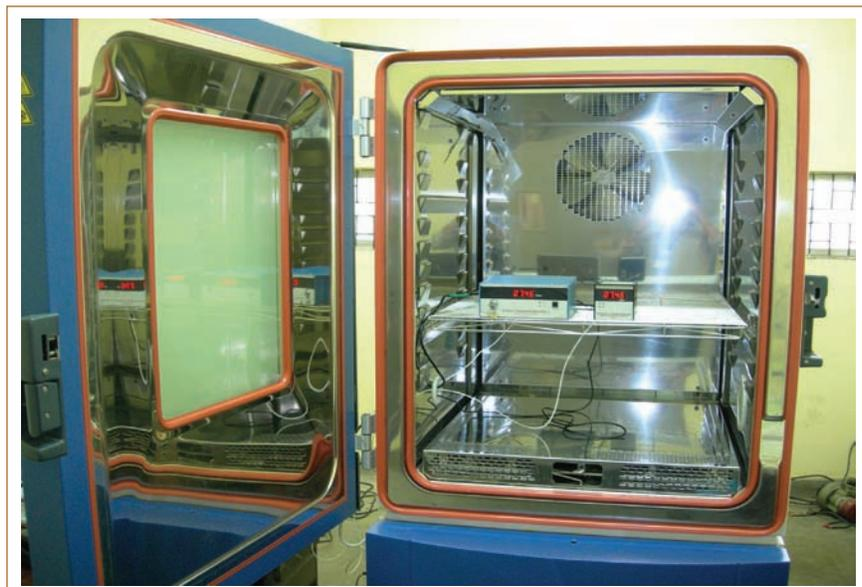
Fig. 2 Photograph of environmental chamber
