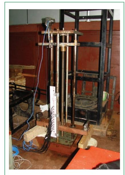
**Fig. 3** Dedicated test setup that simulates CSR translation and SCRAM
