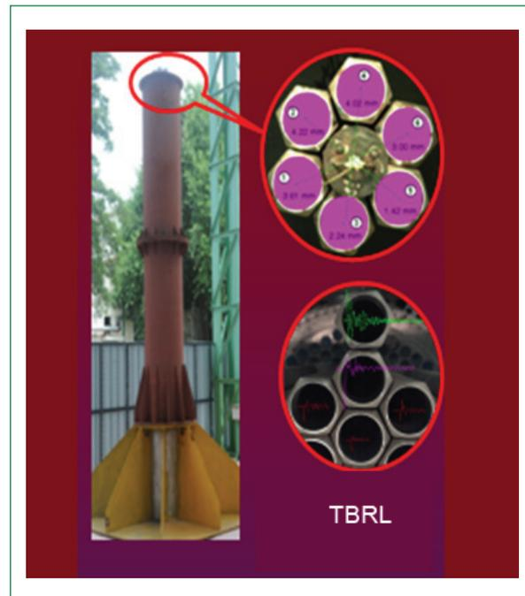
**Fig. 5** Mock-up test carried out TBRL, Chandigarh using low density explosive
