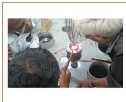
**Fig. 4** Brazing of thermocouples
