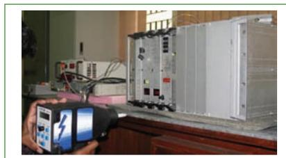
Fig. 1 ESD test in progress
