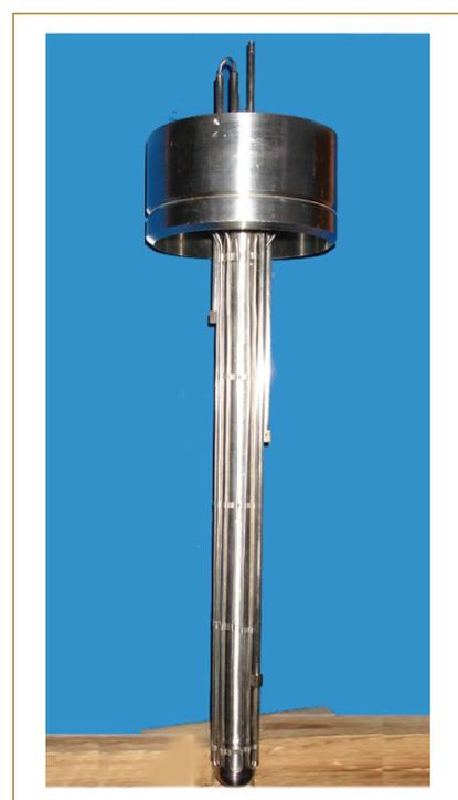
Fig. 1 Nickel coil assembly
