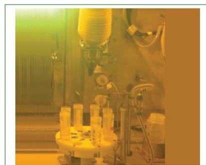
Fig. 2 Sample changer inside radioactive cell
