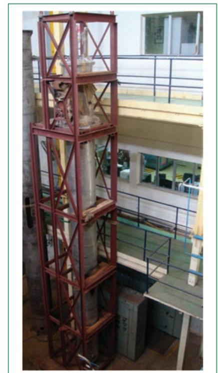
**Fig. 5** Integrated cold trap at engineering hall-III
