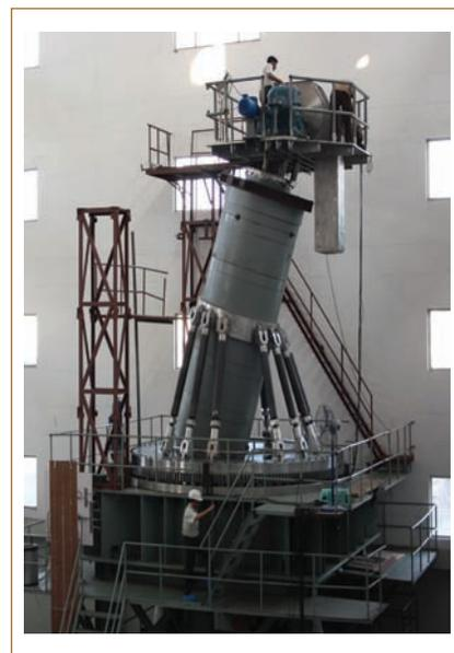
Fig. 1 Inclined fuel transfer machine
