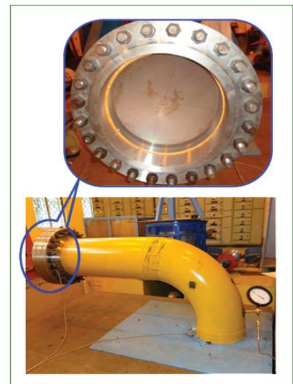
**Fig. 4** Experimental setup for the 20" rupture disc (large size)
