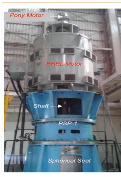
Fig. 1 Primary sodium pump-1 at test bed
