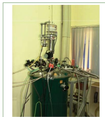
**Fig. 4** Photograph of the SQUID based VSM
