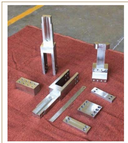
Fig. 2 Machined guide and rails
