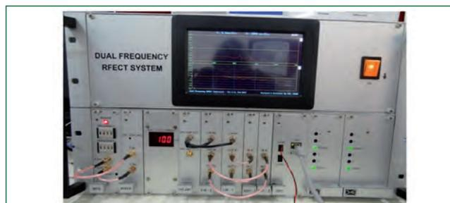
Fig. 1 Indigenous developed RFEC test instrument
