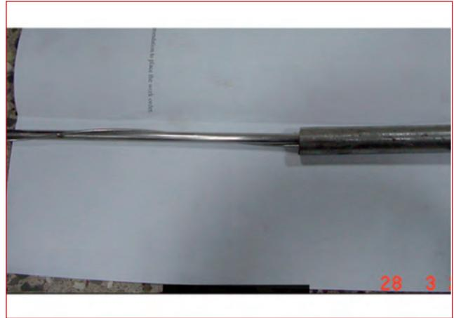
**Fig. 6** Insertion of dummy fuel pin in deflected pipe of magazine
