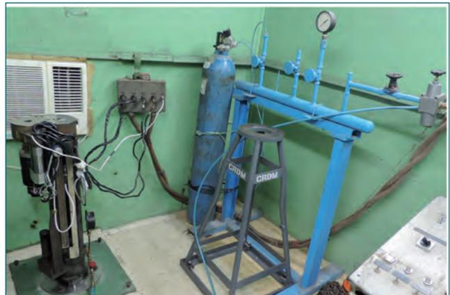
**Fig. 2** Upper part and header for pressure hold test
