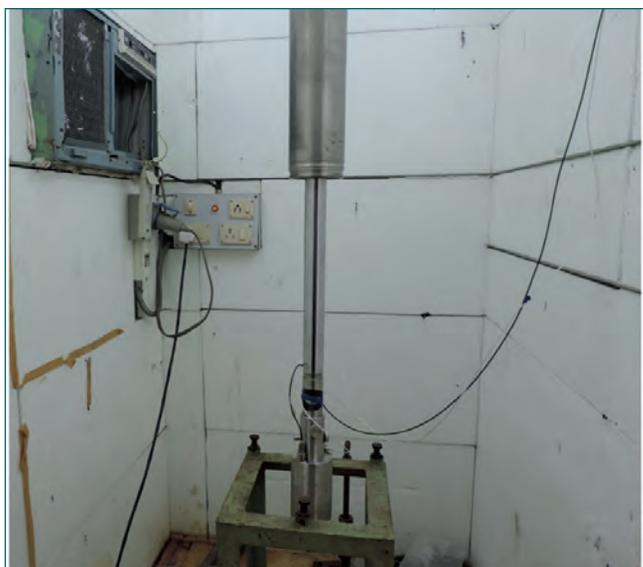
**Fig. 1** Lower part of control rod drive mechanisms
