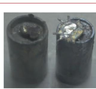
Fig. 5 Liquid cadmium cathode after electrorefining
