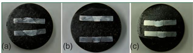
Fig. 1 Moulded samples of micro structural examination (a) 100% argon, (b) 98% argon + 2% hydrogen and (c) 95% argon + 5% helium
