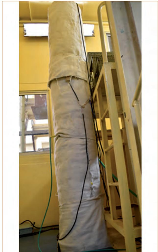
Fig. 1 DSRDM upper part enclosed with heater shell
