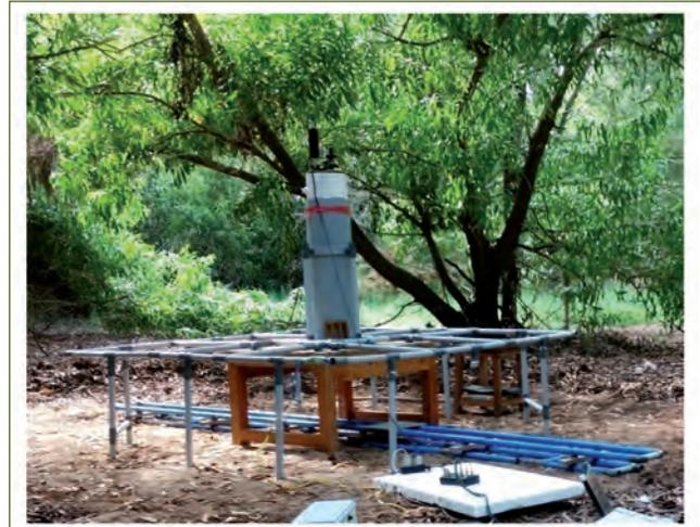
Fig. 1 Photograph of the SQUID system with transmitter loop
