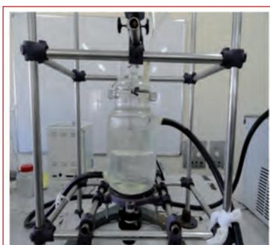
Fig. 1 Constant interfacial area stirred cell
