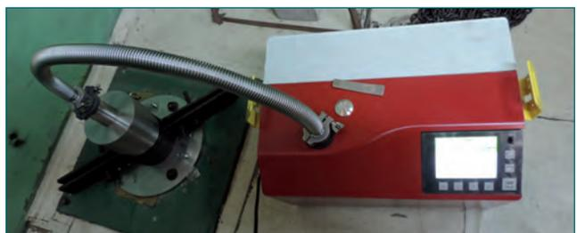
**Fig. 3** Arrangement for helium leak testing of the translation bellows
