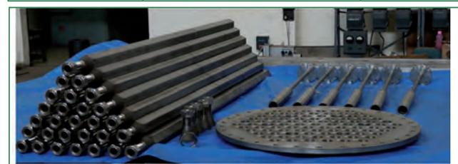
**Fig. 6** FSAs, DSR sleeves and grid plate
