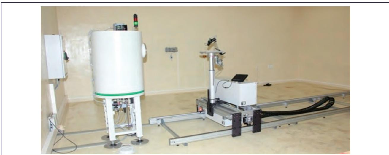
**Fig. 2** Gamma irradiator with linear distancing system
