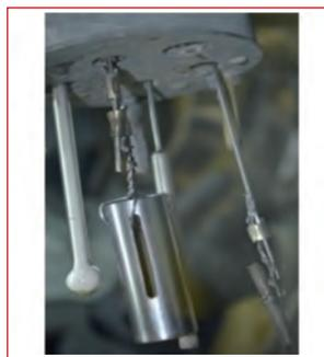
Fig. 1 Electrode assembly for ER runs
