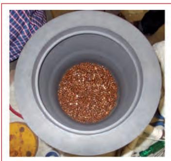
Fig. 2 Copper pellets loaded for melting
