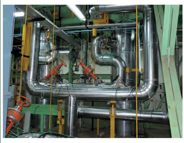
**Fig. 2** Sodium facility for component testing
