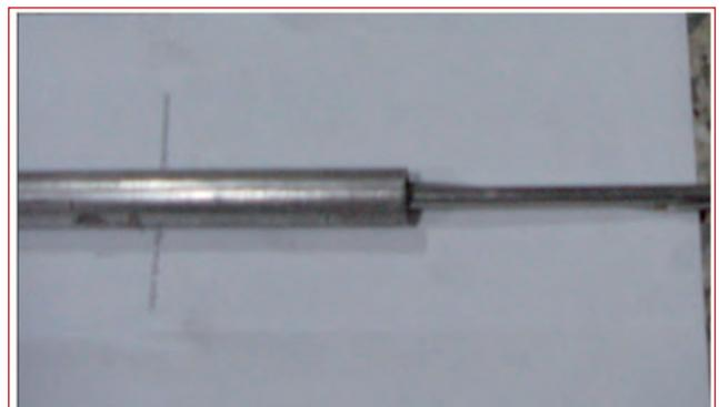
**Fig. 7** Retrieval of fuel pin from other end of deflected pipe of magazine
