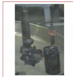
Fig. 2 Uranium deposit at SS430 cathode
