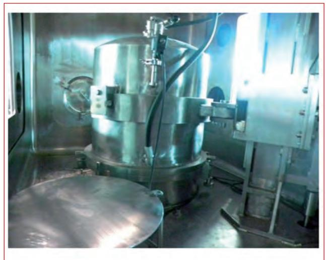
**Fig. 3** High temperature MOX sintering furnace inside glove box
