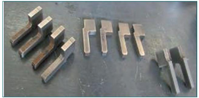
Fig. 9 Hardfaced spacers
