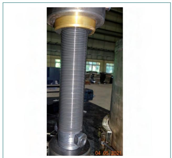
Fig. 4 Grease lubricated mock-up gripper operating tube (screw) after testing
