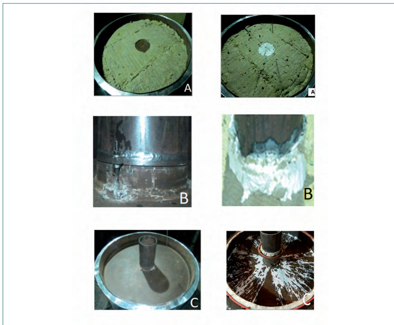
Fig. 2 Sodium leak scenario in (A) with insulation, (B) with 10 mm gap and (C) without insulation
