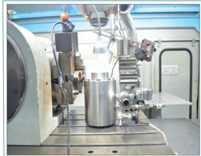
Fig. 2 LASER welding setup for sealing of pressurized capsule inside the pressure chamber
