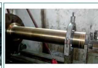
Fig. 5 ID boring of outer duct
