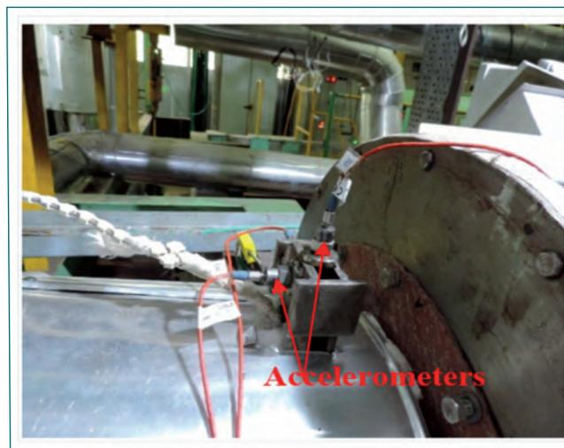
Fig. 2 Photograph of sensor locations at dish end on ALIP
