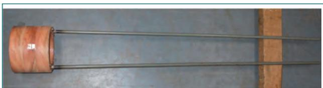
Fig. 3 Radiography film insertion and placement tool
