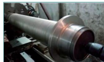
Fig. 3 OD machining of outer duct
