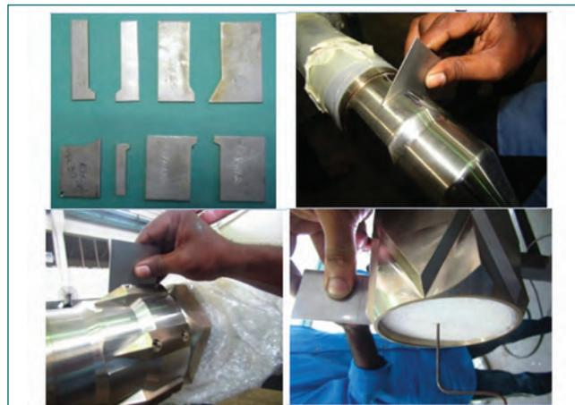
Fig. 3 Photos show machined gauges and their usage on the DSAs
