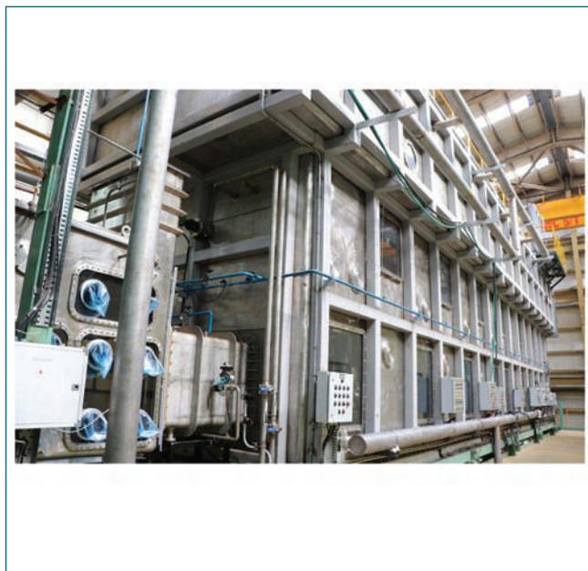
Fig. 1 PPRDF 500m<sup>3</sup> containment box
