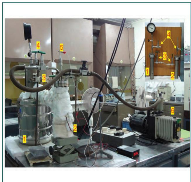
Fig. 3 photograph of the experimental setup used for cleaning sodium by vacuum distillation. (1) distillation vessel kept in a furnace, (2) sodium collection vessel with insulation, (3) SS bellow sealed valves for sodium, (4) bellow sealed valves for argon gas, (5) level probe, and (6) rotary vacuum pump
