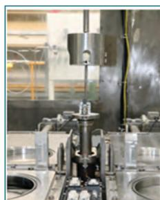
Fig. 2 Reference electrode handling tool
