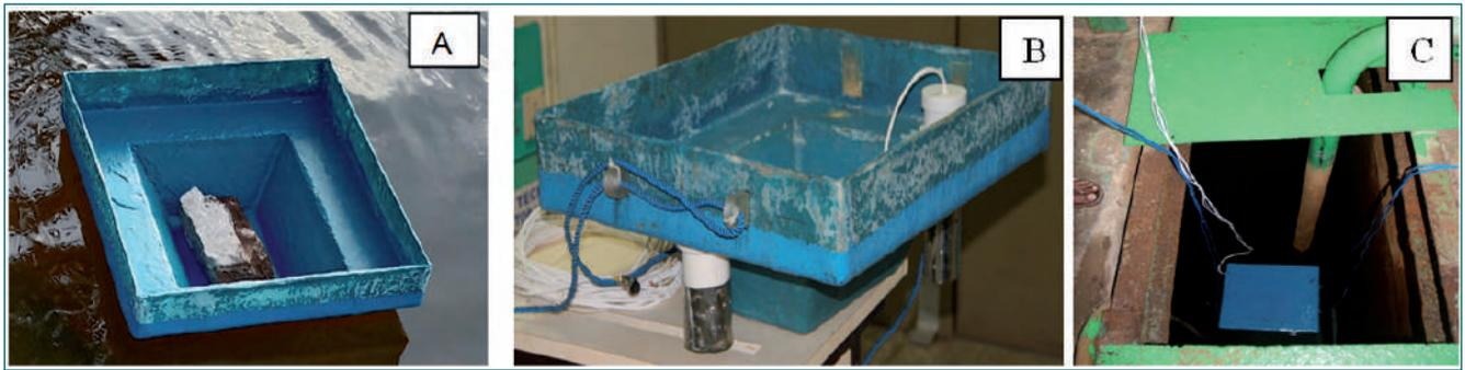
Fig. 2 Fibre float testing at fabrication site,(B) float assembled with the probes,(C) leak test of float with probes in RCL sump
