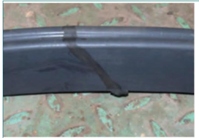
Fig. 2 Test seal with in-situ joint
