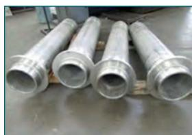
Fig. 2 Pre-machined outer duct
