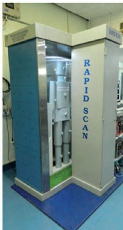
Fig. 2 Monitor with BOMAB phantom
