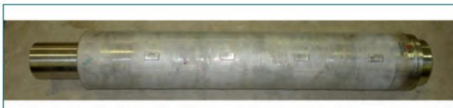
Fig. 1 Inner duct during fabrication
