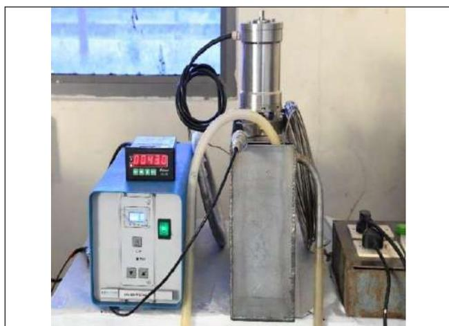
Fig. 1: Equipment for ultrasonic cleaning of centrifugal contactor bowl
