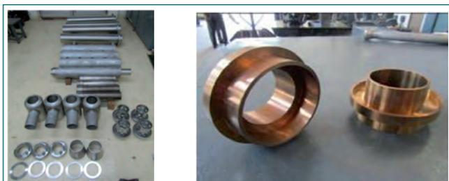
Fig. 1 Machined parts of ALIP
