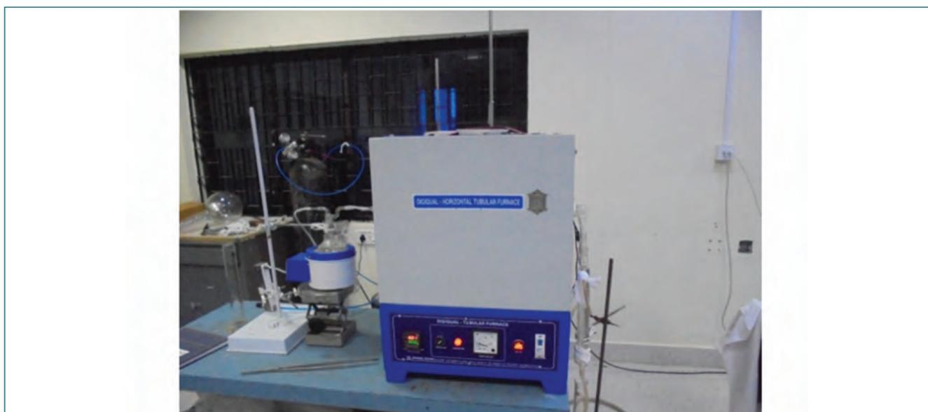
Fig. 1 Pyrohydrolysis facility for boron recovery
