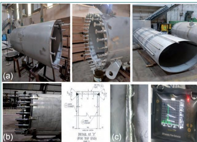
Fig. 1 (a) Annular tank assembly (b) shell with flange corner joint and ((c) UT signal from weld root
