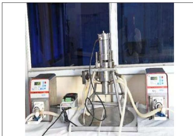
Fig.2: Experimental setup for choking of centrifugal contactor bowl
