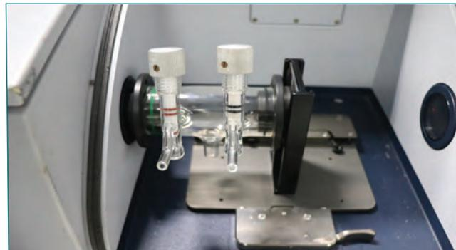
Fig. 2  $\text{CO}_2$  gas sampler placed inside the sample compartment of IR spectrometer
