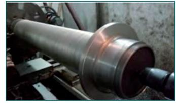
Fig. 3 OD machining of outer duct
