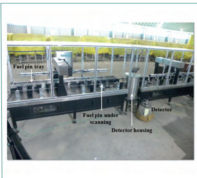
Fig. 1 Gamma scanning system
