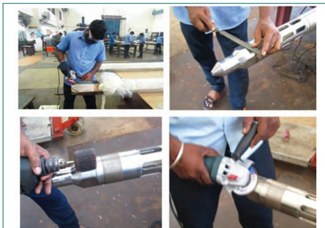
Fig. 1 Photos show radius is being formed in DSA adopting traditional method using filing and hand Grinding techniques
