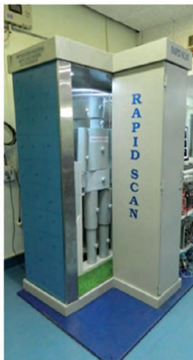
Fig. 2 Monitor with BOMAB phantom
