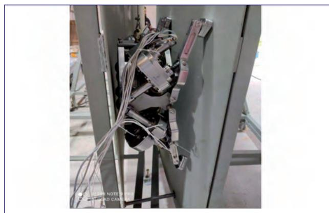
Fig. 3 MSISC system gripping on the wall
