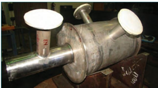
Fig. 4 Fabricated DSA cleaning setup
