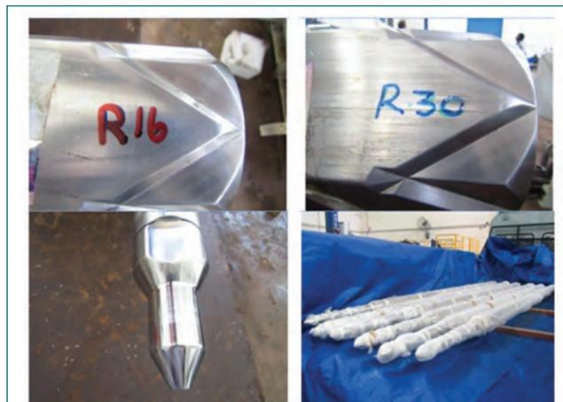
Fig. 2 Photos show radius formed DFSA ends, Discriminator guide portion and completed DFSAs
