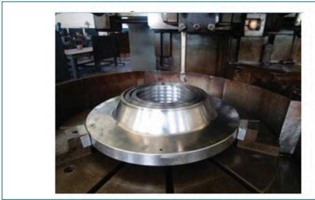
Fig. 7 Labyrinth machining in VTL Machine
