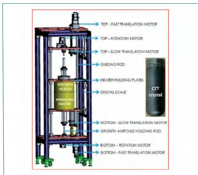
Fig. 1 Schematic of THM setup and photograph of a typical grown CZT crystal
