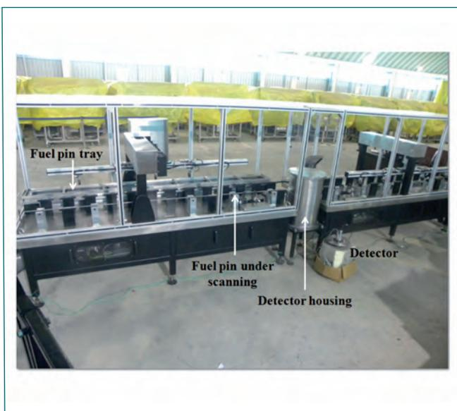
Fig. 1 Gamma scanning system
