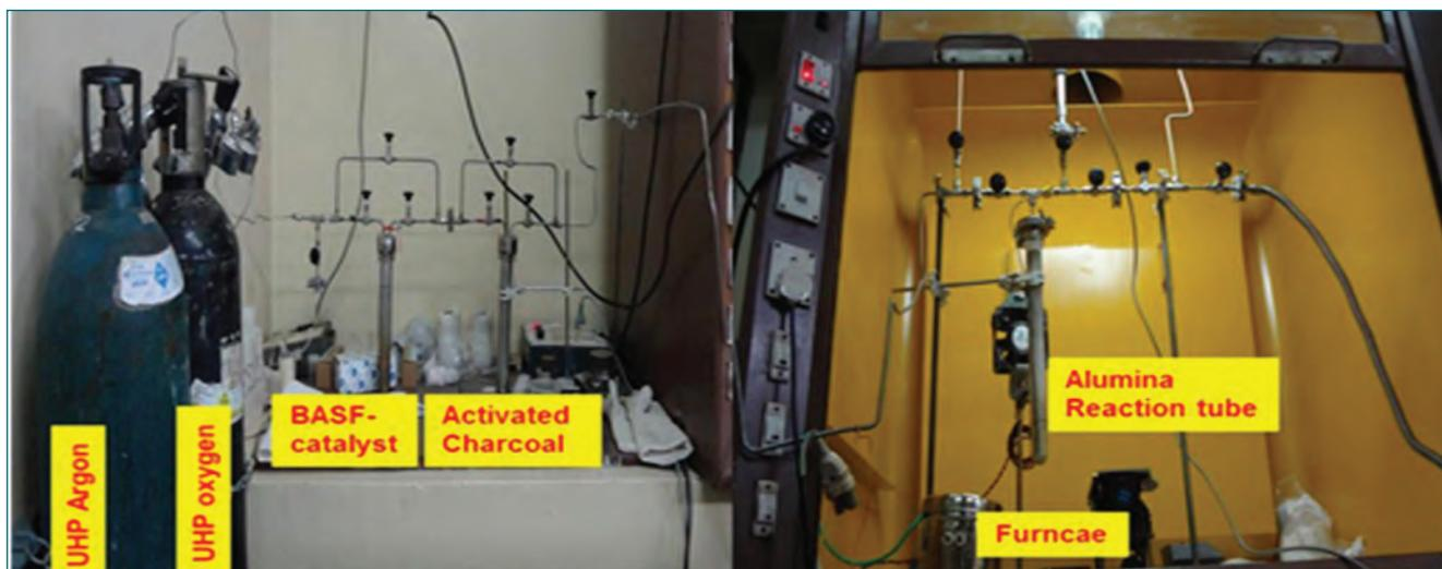
Fig. 1 Photograph of the carbon analysis combustion system established
