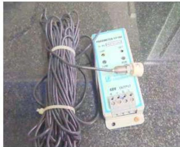
Fig.2: Sensor with pre-amplifier
