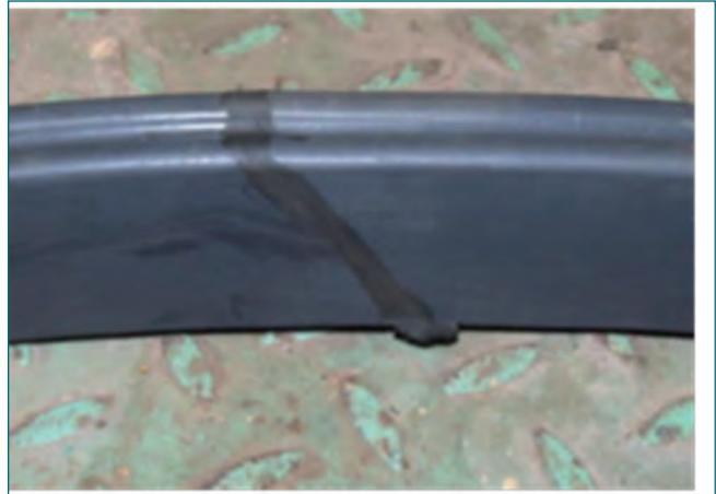
Fig. 2 Test seal with in-situ joint
