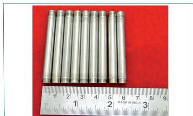
Fig. 3 Fabricated pressurized capsules of IFAC-1 SS (clad tube) & SS 316LN (plug) using laser welding and ready for biaxial creep tests
