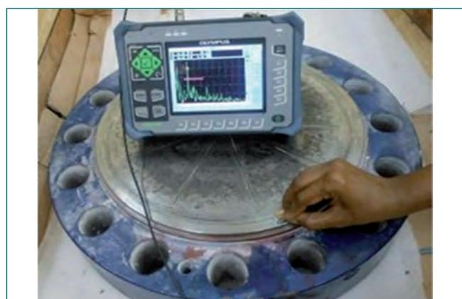
Fig. 3 Indication from discontinuity from diaphragm head
