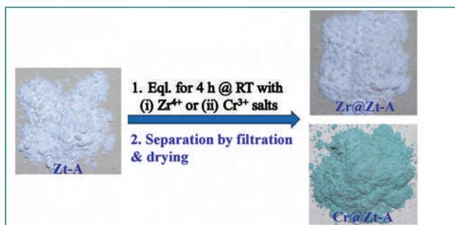
Fig. 1 Equilibration experiment of Zr & Cr with Zt-A
