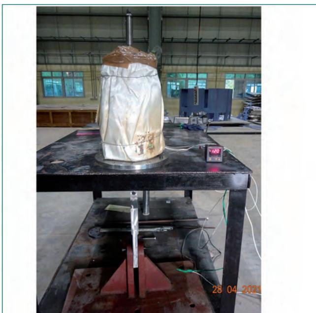
Fig. 3 Photograph of CSRDM gripper screw test setup
