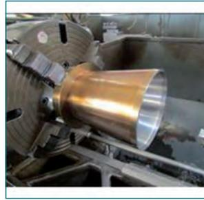
Fig. 7 Machining of diffuser cone
