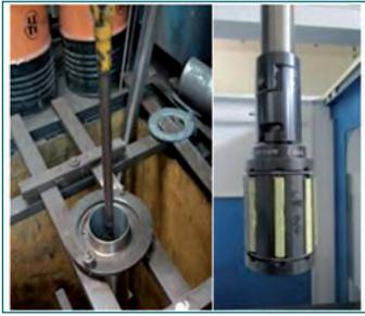
Fig. 6 Vertical honing of outer duct
