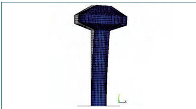
Fig. 5 Deformed shape under seismic excitation in X direction
