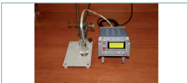
Fig. 1 Photograph of the embedded unit along with the capacitive type probe
