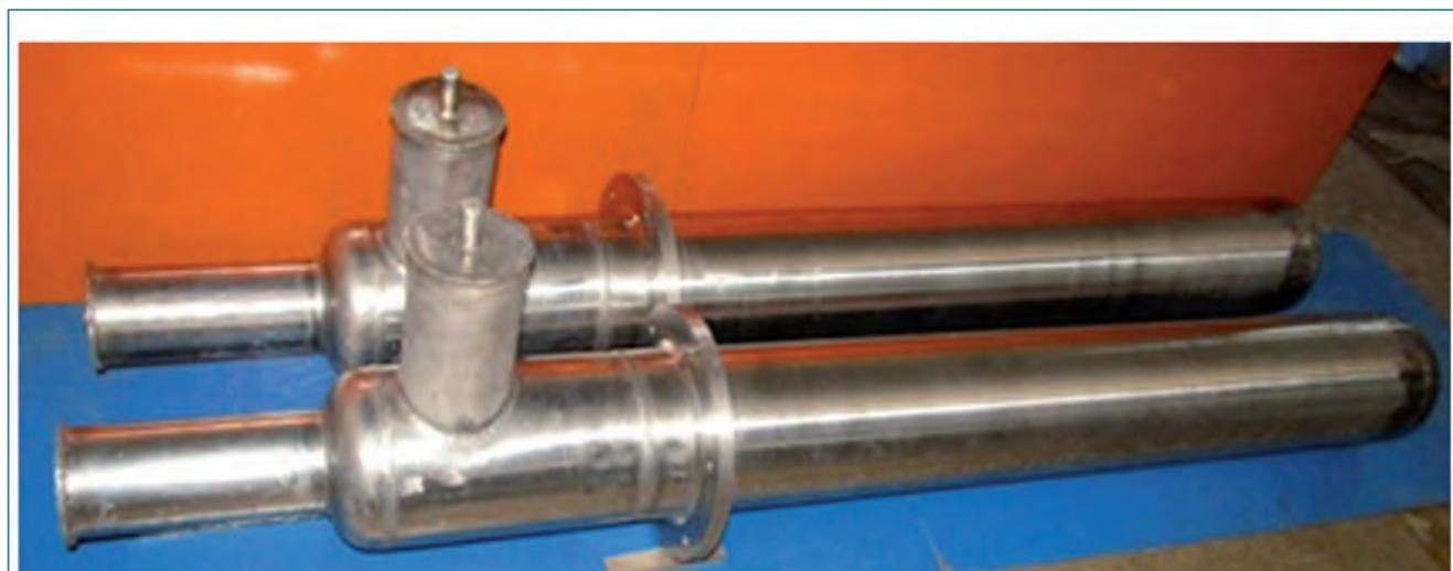
Fig. 15 Inner and outer duct assemblies of PFBR annular linear induction pumps of  $170 \text{ m}^3/\text{h}$  capacity
