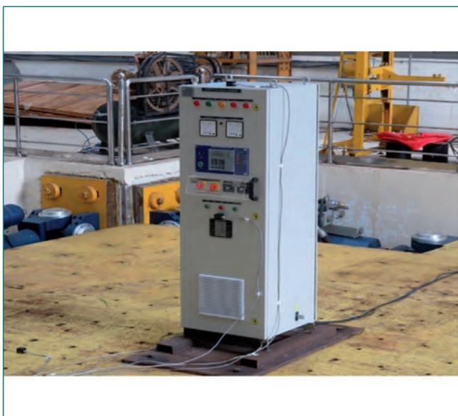
Fig. 1 Prototype 48 V DC charger in shake table
