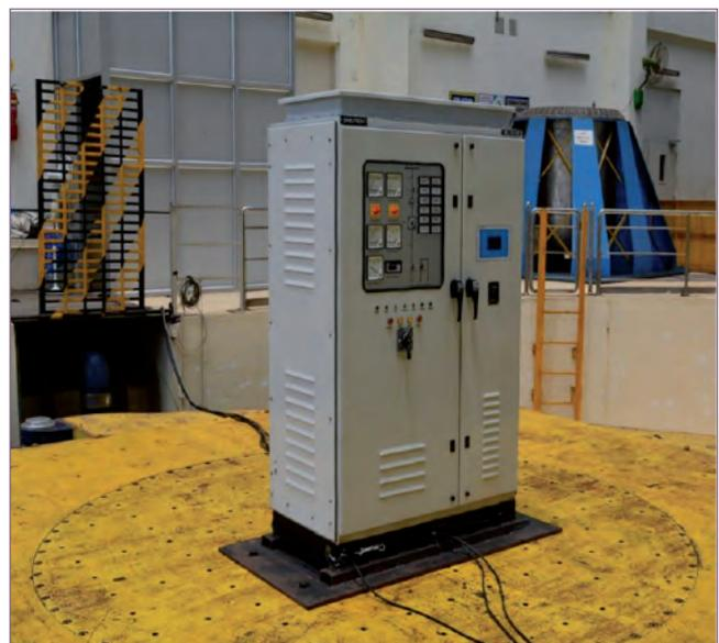
Fig. 3 Prototype 24 V DC charger in shake table
