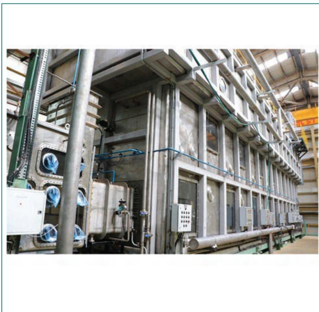
Fig. 1 PPRDF 500m<sup>3</sup> containment box
