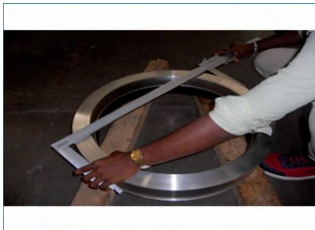
Fig. 2 Outer diameter measurement
