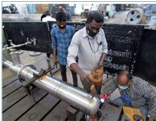
Fig. 14 Quality checks after pneumatic testing
