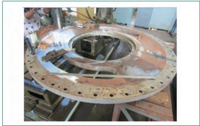
Fig. 8 Ratchet support flange machining in Radial Drilling Machine
