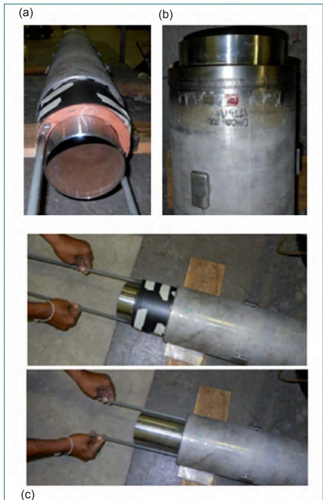
Fig. 4 Sequence of operation (a) Placement of film on the tool (b) Marking and IQI placement (c) Insertion of film cassette inside the annular gap
