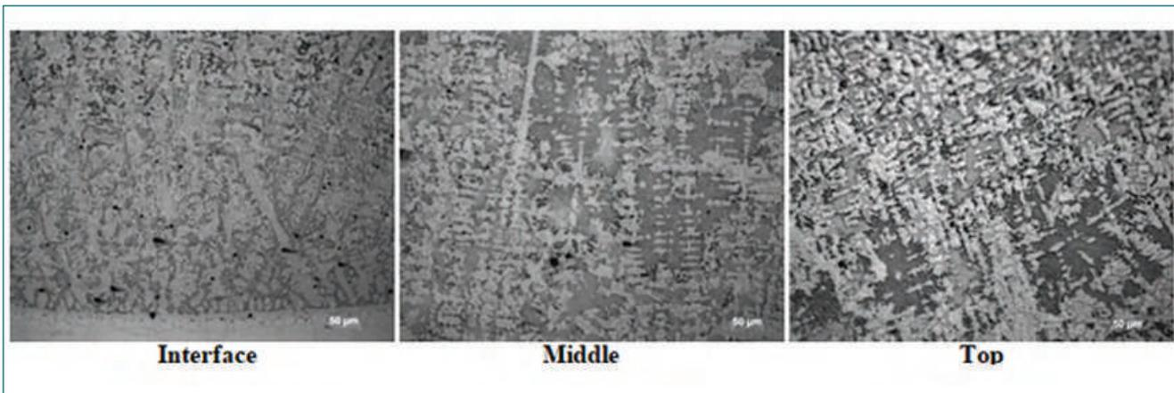
Fig. 12 Microstructure of hardfaced porous shell across coating
