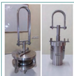
Fig. 1 Electrode grippers
