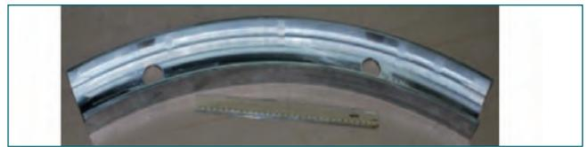
Fig. 2 Machined single piece bottom enclosure
