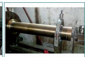
Fig. 5 ID boring of outer duct
