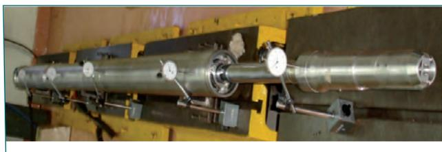
Fig. 1 Concentricity measurement
