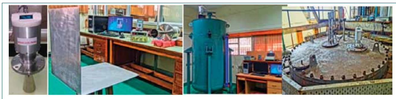
Fig. 1: Functional Testing at Bench Level, for Water Level Measurement and Liquid Sodium Level Measurement
