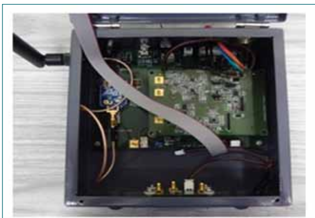
Fig. 1: In-house developed Acoustic Emission WSN Node
