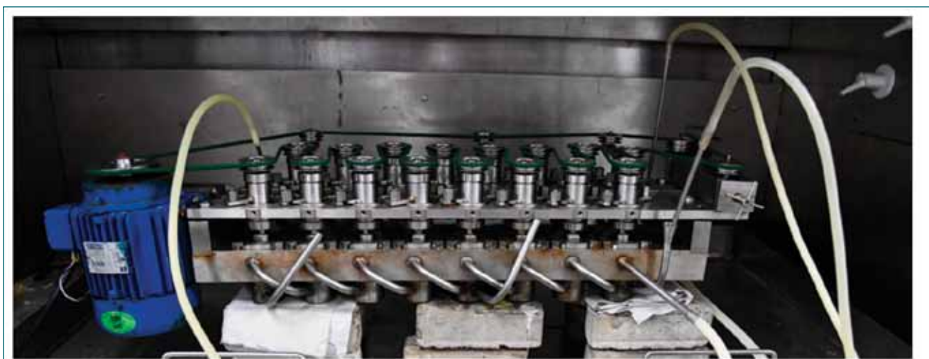
Fig. 1: Photographic view of 16 stages 25 mm ACE bank inside fume hood.
