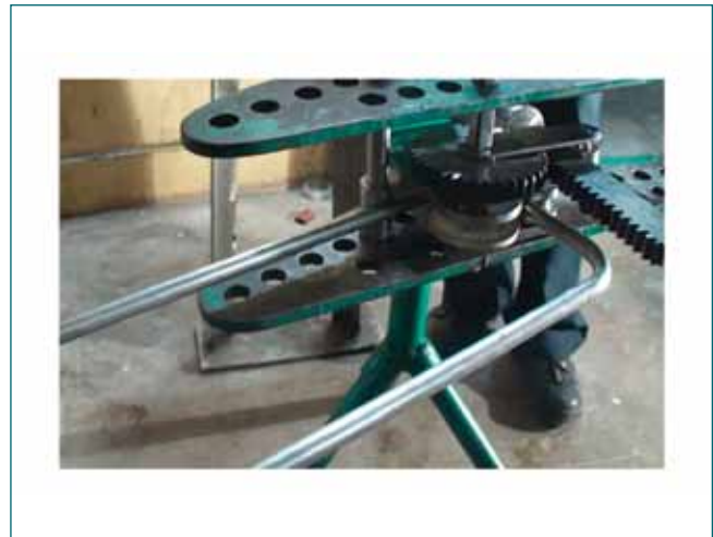
Fig. 7: Fixture attached to conventional bending machine
