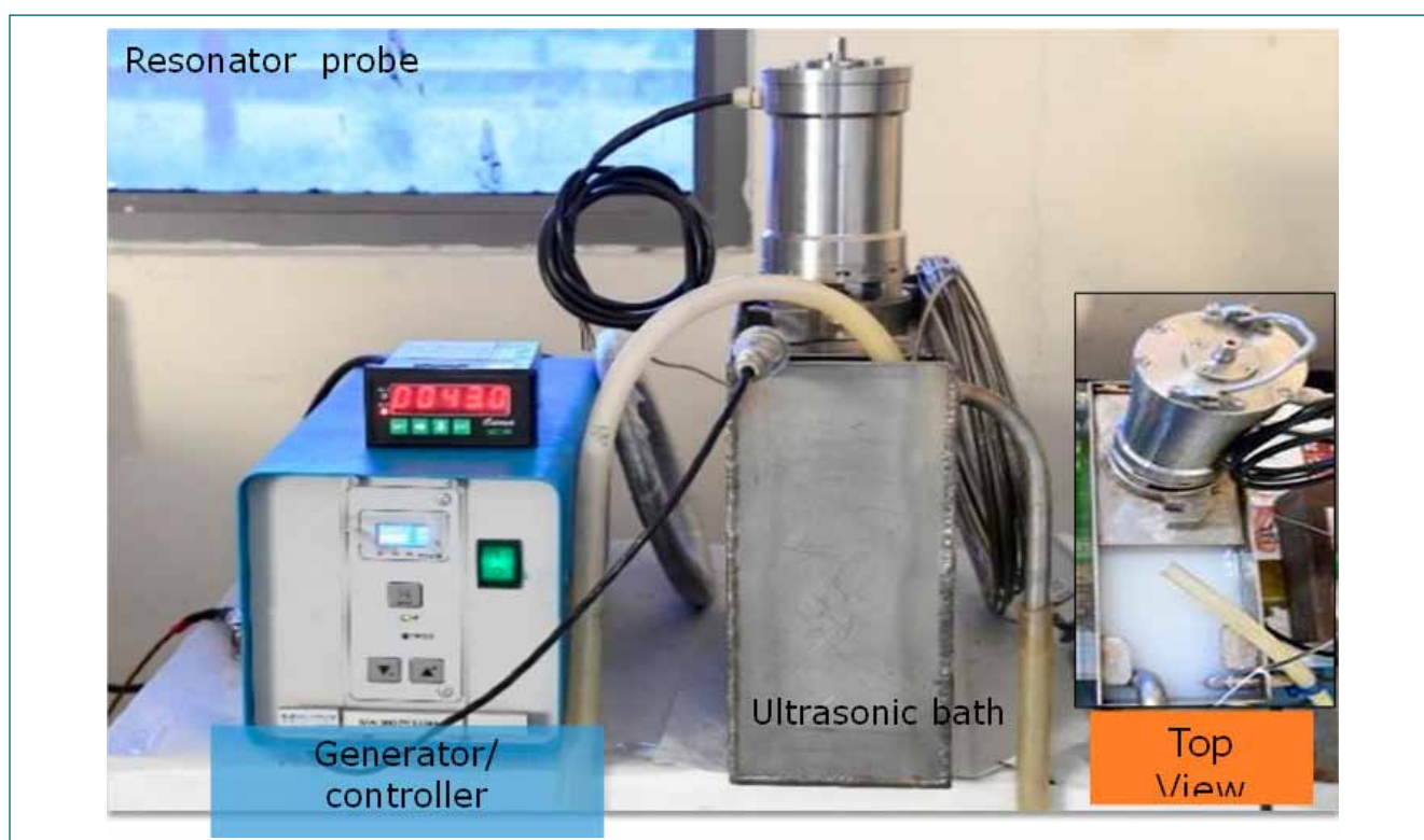
Fig. 1: SS Ultrasonic bath with resonator probe and motor bowl assembly.
