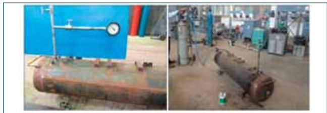
Fig. 2: Hydrostatic and Pneumatic Testing of Compressed Air Receiver Tank
