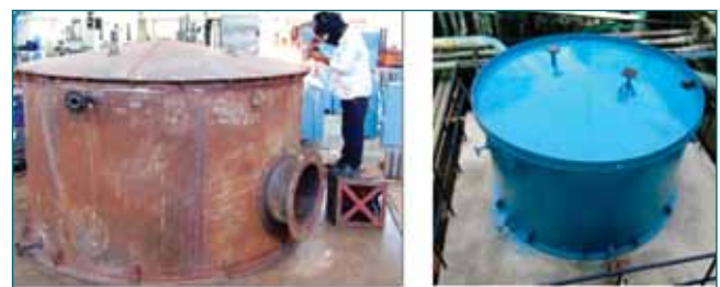
Fig 7: Fabricated and Installed Soft Water Tank
