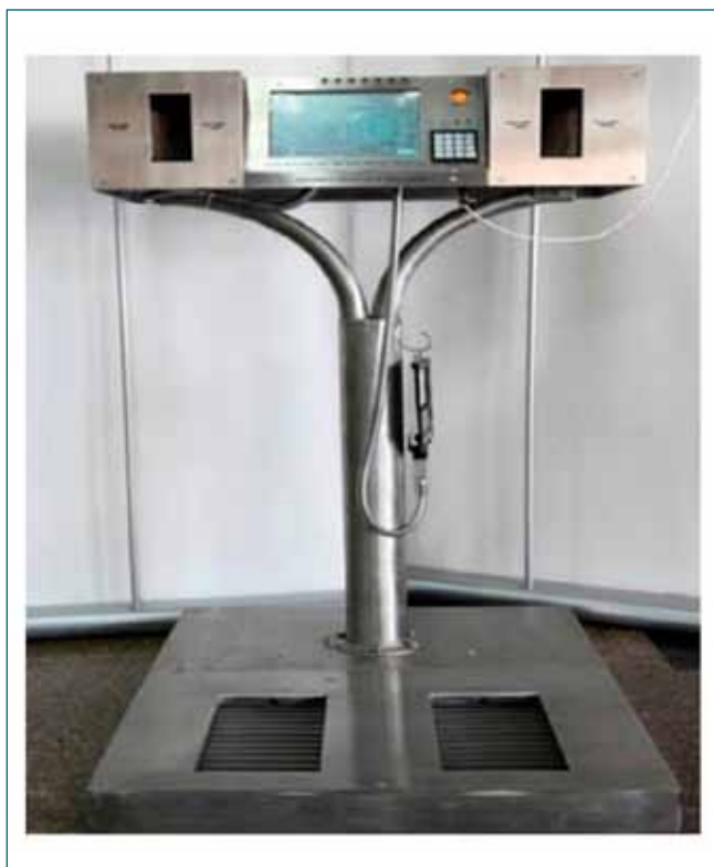
Fig. 1: Alpha Beta Hand Foot and Cloth Contamination monitor using SiPM and optical fiber.
