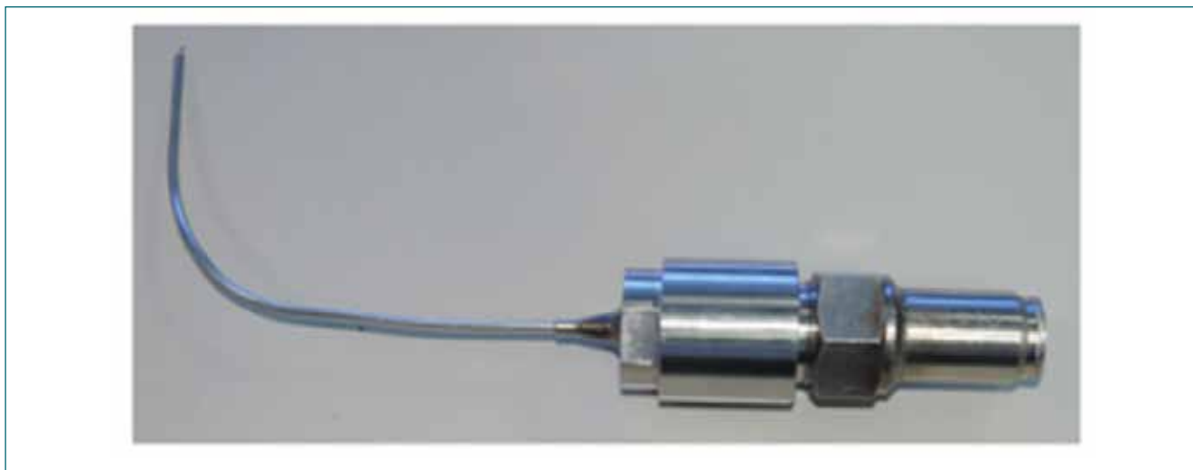
Fig. 1: Dismountable type ultrasonic transducers (UT) assembly
