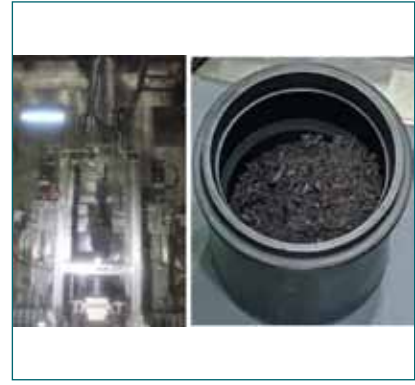
Fig. 6: Scraping station and graphite crucible with scraped uranium
