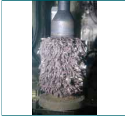
Fig. 5: U deposit in the solid cathode with occluded salt
