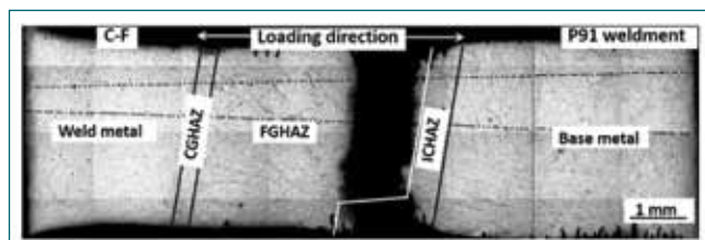
Fig. 2: P91 actual weldment failure location under CFI condition at 550 °C.
