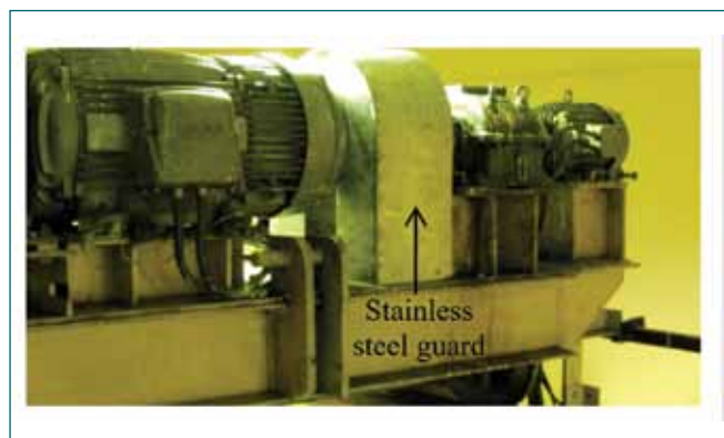
Fig. 5: Image of clutch assembly with stainless steel guard
