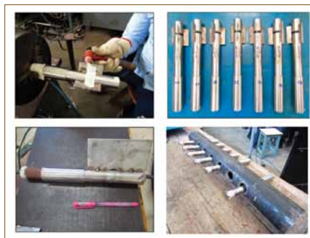
Fig.2: Gas tungsten arc welding of orifice assemblies
