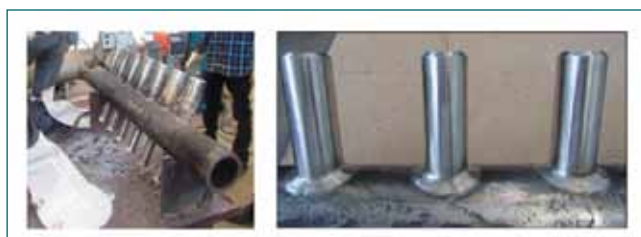
Fig. 3: DMW joint (Carbon Steel and Alloy 800)
