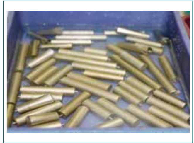
Fig. 3 Uranium metal after cleaning
