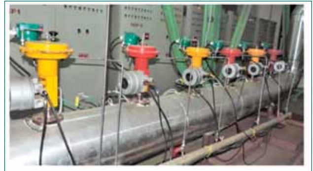
Fig 2: Photograph of bellows test setup with mounting arrangement
