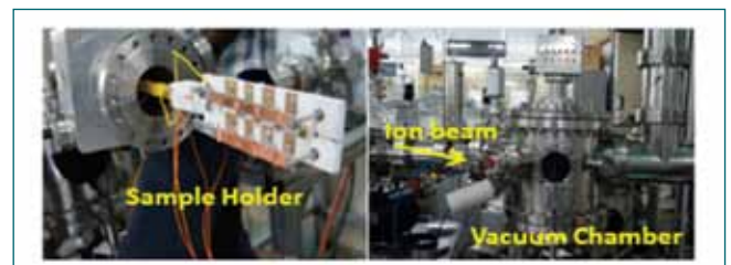
Fig. 3: (a) Detectors mounted on the ceramic sample holder (b) vacuum chamber used for H + ion beam irradiation. The ion beam enters from the left.
