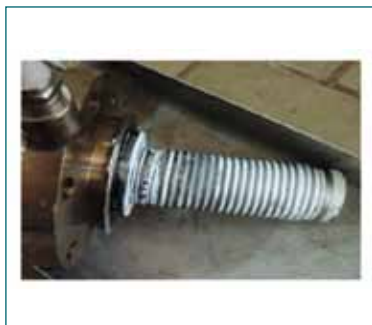
Fig. 3: Bellows after removal from test setup
