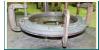
Fig. 4: Clamping arrangement for uniform pressure application
