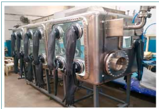
Fig. 1: Special glove box (3m long)
