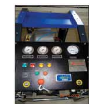
Fig. 2: Self Contained Breathing Apparatus (SCBA) cylinder filling compressor
