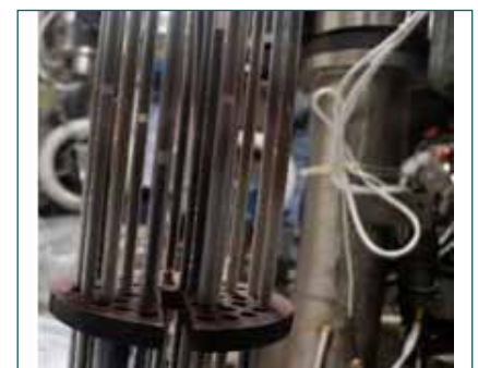
Fig. 4: Cast UZr alloy in Coated quartz mould
