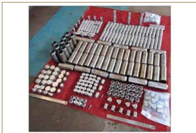
Fig.1: Precisely machined components of modified orifice assemblies
