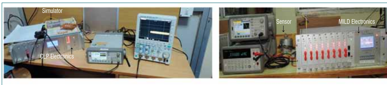
Fig. 1: Validation testing of comprising of Continuous Level Probe electronics (CLPE) and Mutual Inductance type Leak Detector Electronics (MILDE) at Lab
