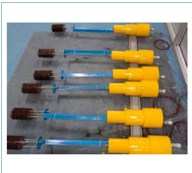
Fig. 1: Heat pipe cooled LED light with Lead shielded Plug
