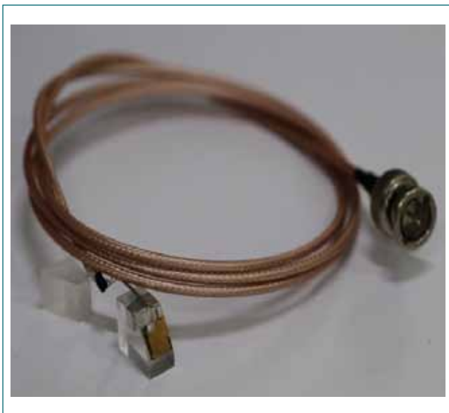
Fig. 1: SAW transducer fabricated with home grown PZN-PT single crystal
