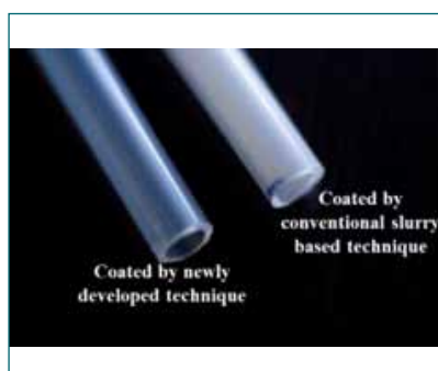
Fig. 2: Quartz tube coated by newly developed and conventional study technique.
