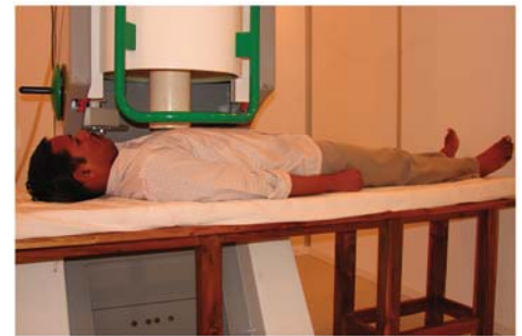
Fig.1: Liquid helium cryostat with four SQUID channels
