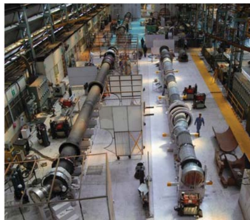
Fig. 5 : PFBR Steam generator under manufacture
