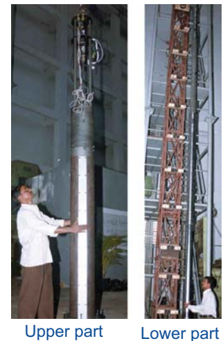
Fig. 3: Diverse safety rod drive mechanism
