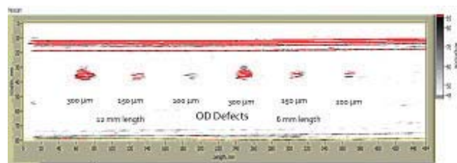
Fig. 2: Collated B-scan image of OD longitudinal defects (generated by processing four longitudinal B-scans obtained at 20 mm intervals)
