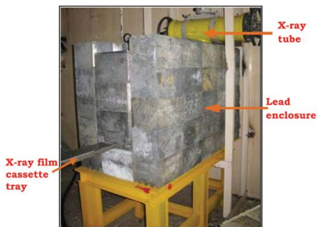
Fig. 1 : Photograph of the X-ray machine and shielding block positioned in the lower isolation area for radiography of the irradiated control rod
