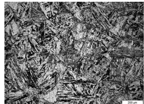
Fig.1b: Microstructure of ICHAZ simulated at 875°C for 5 minutes and tempered at 760°C for 3 h of 1150°C normalized and 760°C tempered in P91B steel
