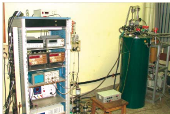
Fig. 3: Photograph of the high field SQUID magnetometer set-up which incorporates the Variable Temperature Regulator (VTR)
