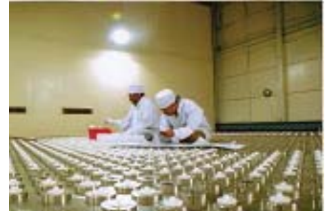
Fig. 4 : PFBR Grid Plate under Assembly in Nuclear Clean Hall
