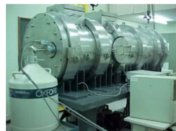
Fig. 1: Compton profile spectrometer
