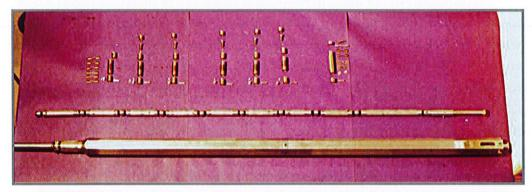
Irradiation capsule and components with steel subassembly
