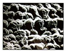
Shrinkage cavity in casting
