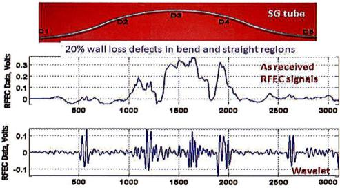
RFEC probe for SG tube inspection and signal processing around the bend region to extract defect information
