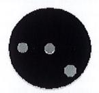
Tomographic slice of aluminium cylinder with holes
