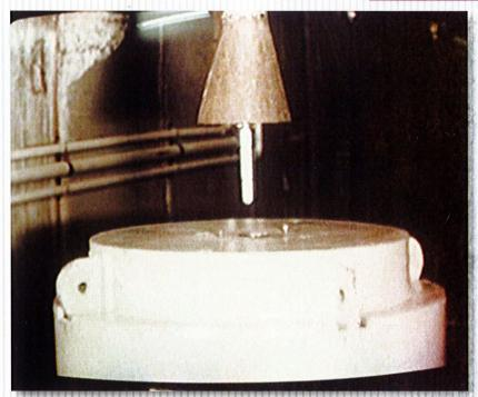
Lowering of neutron source pin into the cask
