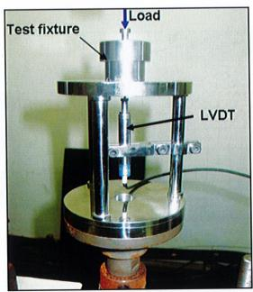
Modified shear punch test fixture
