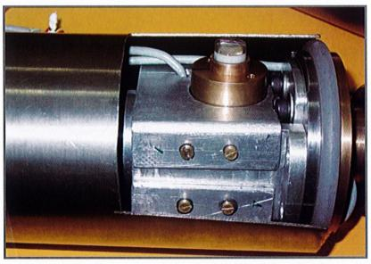
Focused eddy current sensor for scratch detection in calandria tubes
