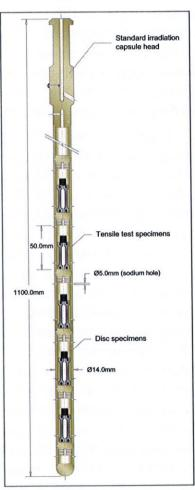
Irradiation capsule for grid plate specimen irradiation in FBTR
