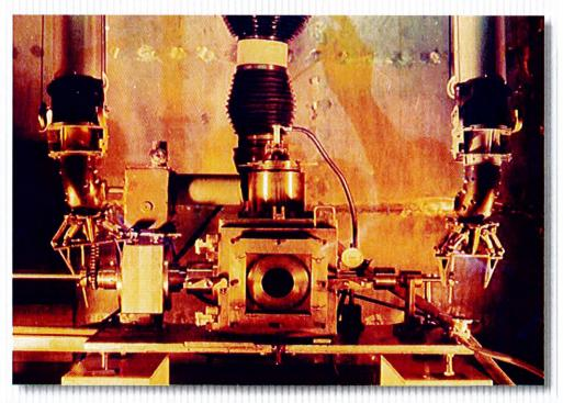
Neutron Source pin welding progressing inside the hot cell
