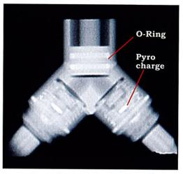
Photograph of pyro thruster and its digitised NR image
