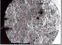
SEM fractograph of delaminated stellite, showing brittle failure along the dentrite
