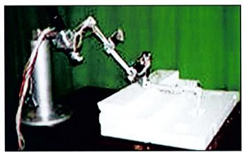
Prototype Snake-like robot reaching out to a task-space location
