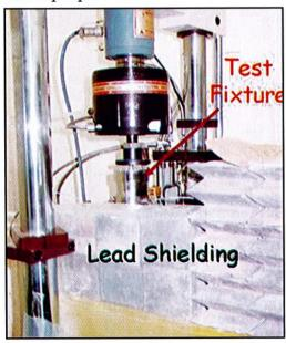
Shear punch testing of irradiated specimen with local shielding around test machine
