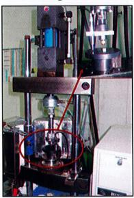
Custom built servo hydraulic machine for ball-indentation test
