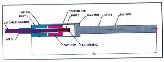
Sketch showing the general coil termination arrangement of ECPS
