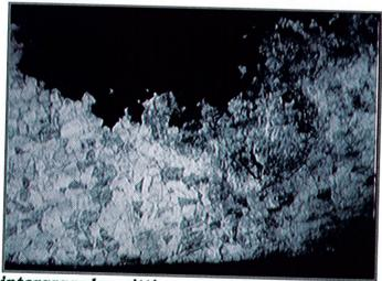
Extensive intergranular pitting attack on the surface of the tube the inner disruption of oxide scales
