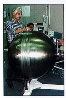
Ultrasonic examination of IR-Satellite propellant tanks of ISRO at LPSC, Bangalore
