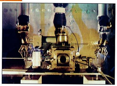
Remote welding chamber in the hot cell
