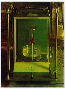
Density measurement system for swelling estimation
