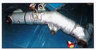
Fatigue damage of landing gears of fighter aircraft assessed using X-ray diffraction and MBE techniques
