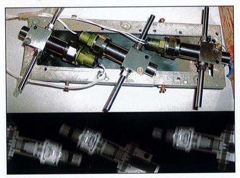
Photograph of a dual pyro valve and its digitized NR image
