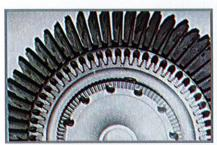
Failed turbine wheel of Aero engine
