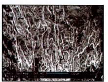
Fractured surface of failed disc showing cleavage and quasi-cleavage fracture
