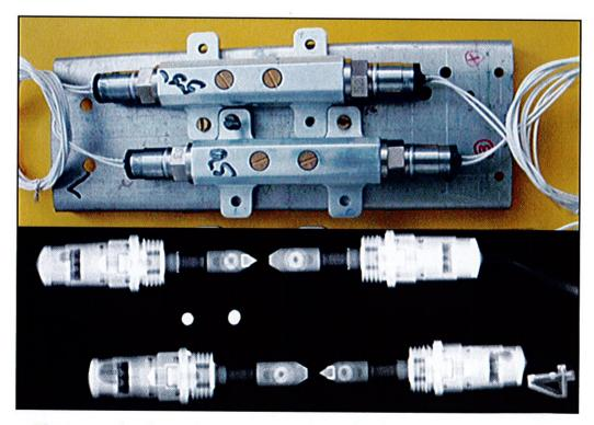
Photograph of satellite cable cutter and its digitized NR image
