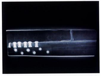
Photograph of riveted aluminium airframe and its digitized NR image indicating ingress of moisture inside the riveted lap joint in an airframe
