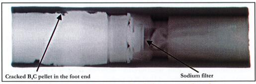
Neutron Radiograph of the control rod
