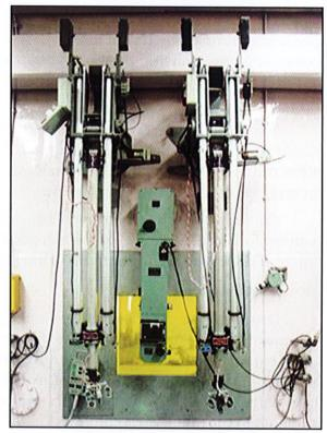
View of the hot cell with shielding glass window and MSM
