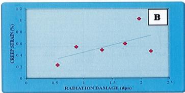
Creep of Zr-2.5% Nb at 314°C and average stress 150 MPa A. Creep strain vs Fluence B. Creep strain vs radiation damage (dpa)
