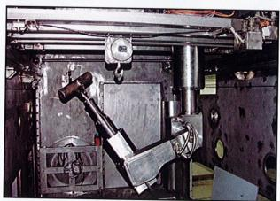
In-cell crane with power manipulator installed in the containment box of pilot pyro-chemical processing
