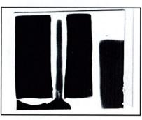
Radiograph showing shrinkage cavities at the transition portion
