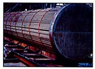
Carbonate re-boiler heat exchanger
