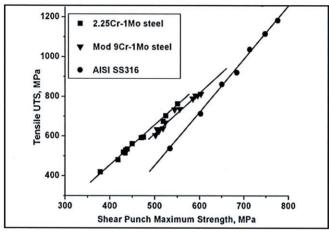
Tensile to shear correlation obtained for various alloys
