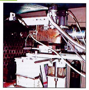
Microfocal radiography of TTS weld joints of PFBR SG
