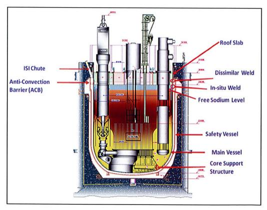
Vertical sectional view of the PFBR under construction showing the ISI chute and interspace between the main vessel and safety vessel
