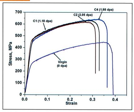
Stress-strain plots of grid plate specimens at various 'dpa'
