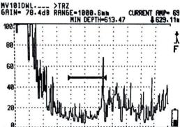
Ultrasonic inspection of shell weld region of mockup sector of PFBR and corresponding A-scan signal of a defect
