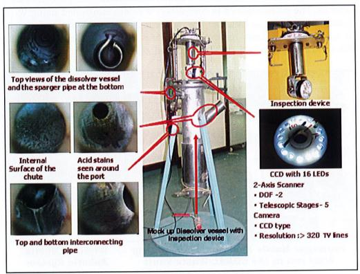
Visual inspection device for dissolver vessel
