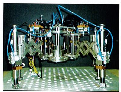
Steam Generator Inspection Device on mockup tube sheet
