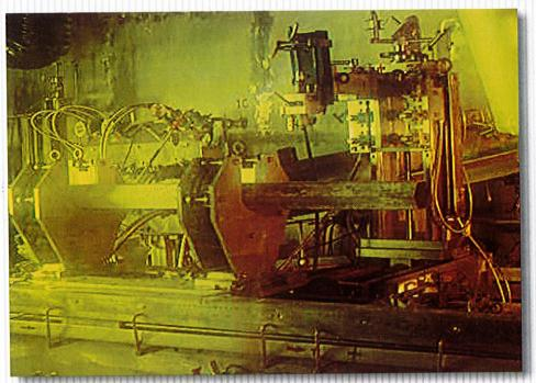
Dimensional Measurement cum Laser Dismantling (DMLD) system in hot cell
