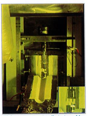
testing were either from the cladding (tubular specimen), wrapper (flat type) or prefabricated miniature tensile specimens (flat type) subjected to irradiation.
