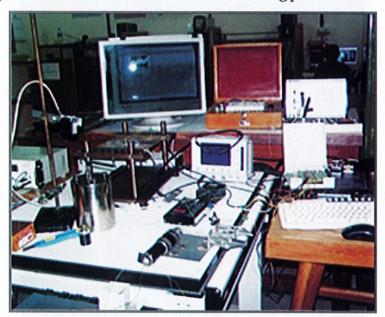
Slip Sensing test set-up
