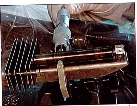
Diameter measurement of the pre-pressurized capsules
