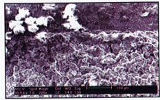
Fractograph showing decohesion of grains and intergranular (secondary) cracks
