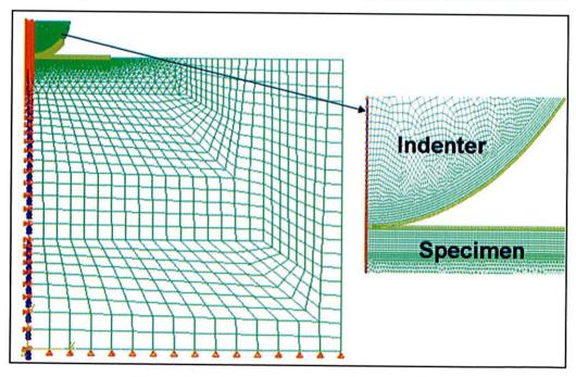
FE model of the spherical indentation
