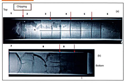
Radiography image indicate the pellet regions of the control rod (a) top portion. (b) bottom portion - The radial cracks at the centre of the pellets are marked by arrows
