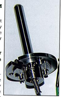
Photograph of sodium leak detector
