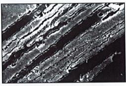
SEM photograph showing grain boundary delamination and corrosion products
