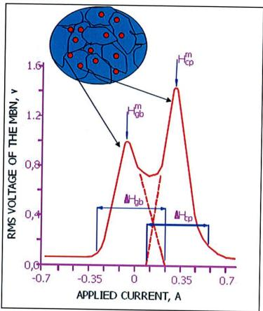
RMS voltage of the MBE vs. applied current showing two stage magnetization process in tempered steels:  $H_{gb}^{\ \ m}$  and  $H_{cp}^{\ \ m}$  correspond to obstruction of the movement of domain walls due to grain boundary and carbide phase respectively
