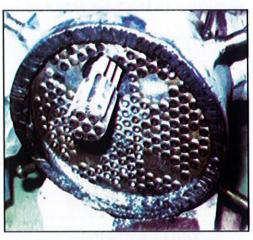
Through and Through Opening and Intergranular Corrosion at the Defective Location due to Sludge Deposit
