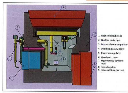
Cross sectional view of a typical Hot Cell
