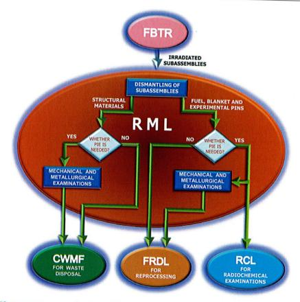
The movement of radioactive materials in/out of RML
