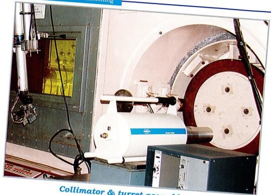
Collimator & turret assembly for gamma scanning of irradiated fuel pin
