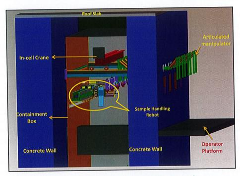
CAD model of the conceived robotic system for DFRP remote analytical cell
