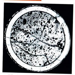
Photomosaic of fuel pin cross-section after 25 GWd/t burnup
