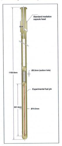
Irradiation capsule for experimental fuel pin irradiation in FBTR
