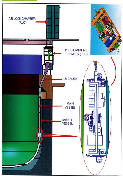
CAD model showing the ISI vehicle deployed in the PFBR MV-SV interspace
