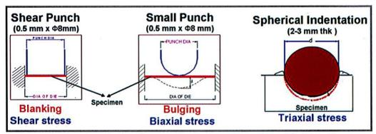
Schematic showing the loading configuration of punch and indentation tests
