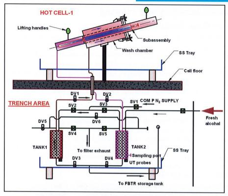
Schematic of sodium cleaning system
