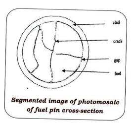
was perfected using special methods like preparation of segmented image of the photomosaic to reduce noise, border killing etc.
