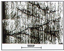
**TGSCC** crack networks
