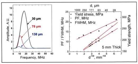
Autopower spectra of ultrasonic backwall wall echoes obtained from 316 stainless steel specimens with different grain sizes and variations in yield stress, peak frequency and full width at half maximum of the autopower spectra of the backwall echoes with the grain size
