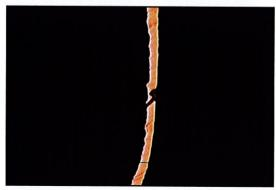
Through-the-thickness cracks in the bellow convolutes
