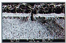
SEM photograph showing matrix depleted zone, crack in protective coating and grain boundary spikes
