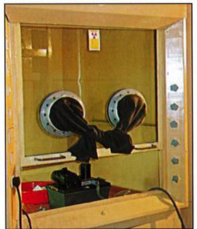
TEM specimen preparation system for irradiated material
