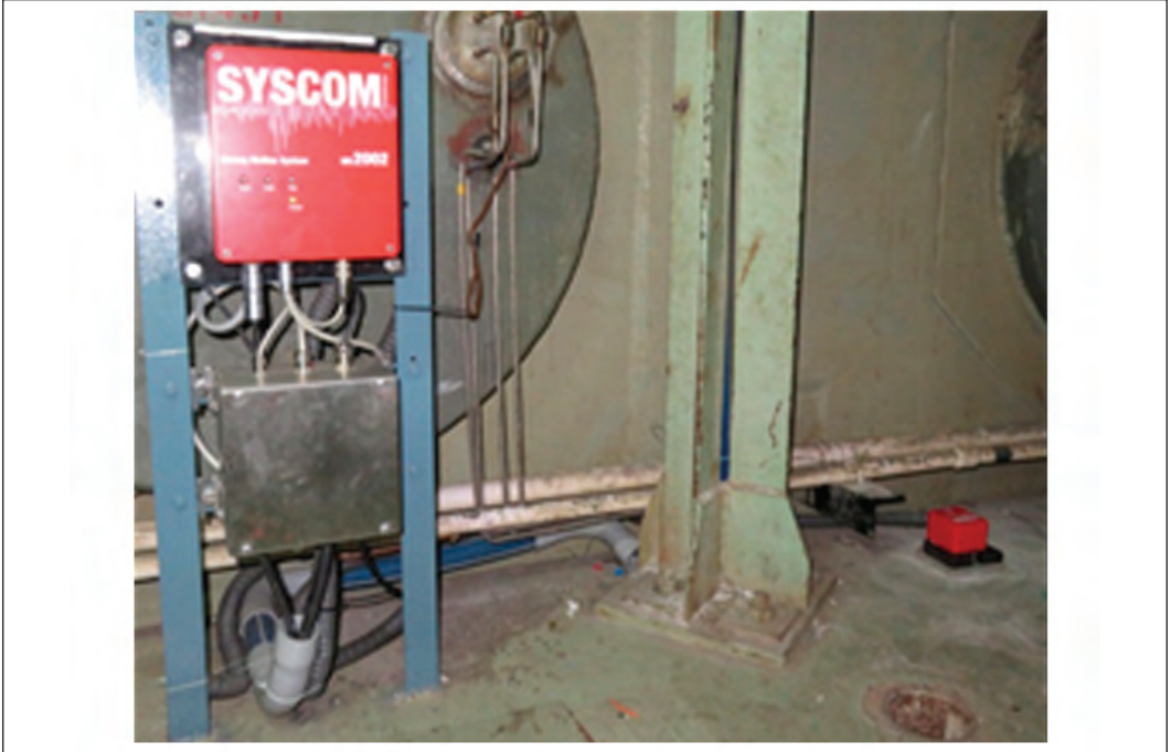
Seismic sensor located at RCB
