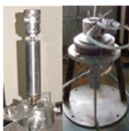
High speed centrifuge for feed clarification for separation of insolubles upto 0.5 microns size
