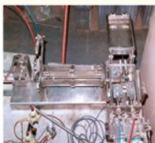
Single pin chopper with microprocessor based controller amenable for remote operation and maintenance
