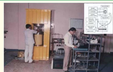
High pressure high temperature resistivity apparatus (circa 1985)
