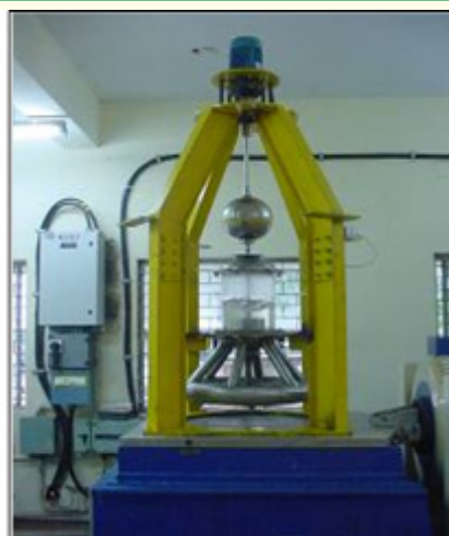
Qualification of hydrostatic bearing at 2t slip table
