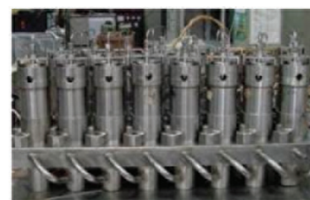
Centrifugal extractors with short residence time to minimize solvent damage
