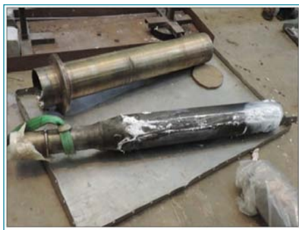
Figure 3: Sodium Cleaning of ALIP for PFBR
